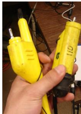
Two-channel (microphones and geophone) motion sensor (a) and single-channel, active noise suppressing geophone (b). (Stewart 1998)
