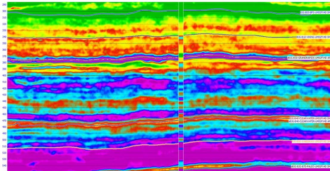
FIG. 4. Impedance inversion section with blind well, stratigraphic interpretation and well based input model
