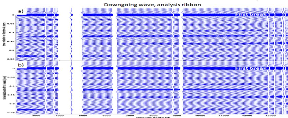
Figure 1: a) A ribbon of data from the VSP downgoing wave approximately 0.3 sec wide and beginning just before the first breaks. b) The result of spatial averaging of the ribbon in panel a) using an averaging half-width of 400ft. Each trace of panel b) is an average of the traces of panel a) over the depth range  $\pm 400$ ft relative to the trace position.
