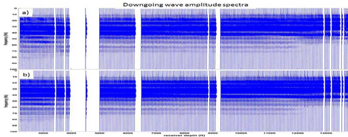
Figure 2: The amplitude spectra of the traces in Figure 1 are shown. The decay of high frequencies with increasing depth is evident in both panels.
