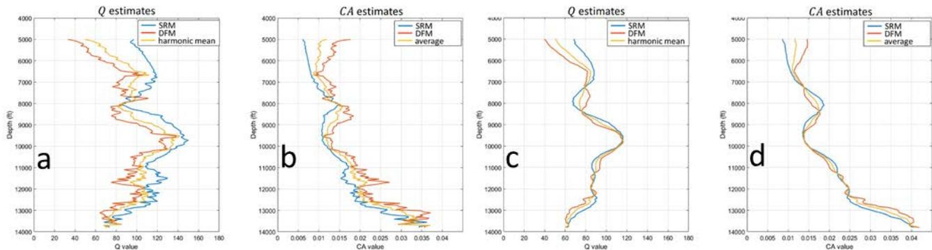
Figure 3: a and b are  $Q$  and  $CA$  estimates using the data of Figure 1a by both the SRM and the DFM. c and d are estimates using the data of Figure 1b.
