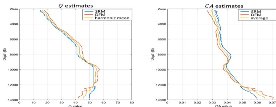
Figure 4: The result of an attenuation analysis where the reference signal,  $w_1$ , is taken to be the Klauder wavelet at depth  $z = 0$ . The input data were those of Figure 1b so this result should be compared to Figure 3 c-d. Note the change in the depth axis which now extends to 2185ft. The stair-stepping on the  $Q$  curve from the DFM happens because that method estimates  $Q$  to the nearest integer only. The resulting  $CA$  estimate shows saw teeth.
