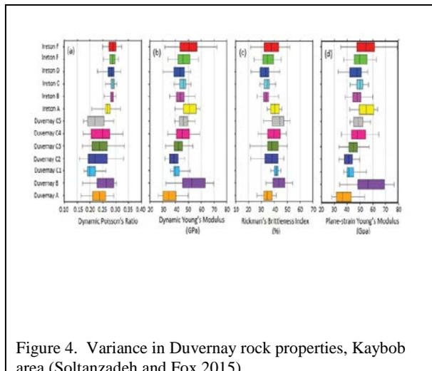
Figure 4. Variance in Duvernay rock properties, Kaybob area (Soltanzadeh and Fox 2015) over 25 well locations using cores and well logs. (Soltanzadeh and Fox 2015). This analysis shows there is variation both laterally and vertically in the Duvernay Formation over the study area.
