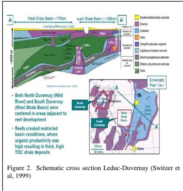
Figure 2. Schematic cross section Leduc-Duvernay (Switzer et al, 1999)
