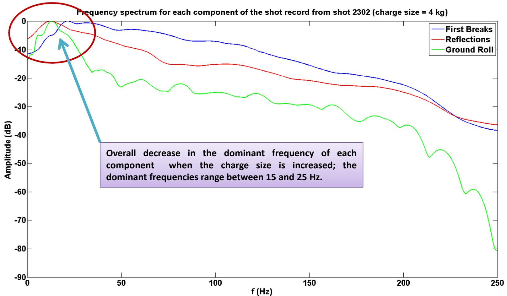
**FIG.5.** Frequency spectra for each of the components of the shot record for shot 2302. Note the decrease in frequency of each component with the increased charge size.
