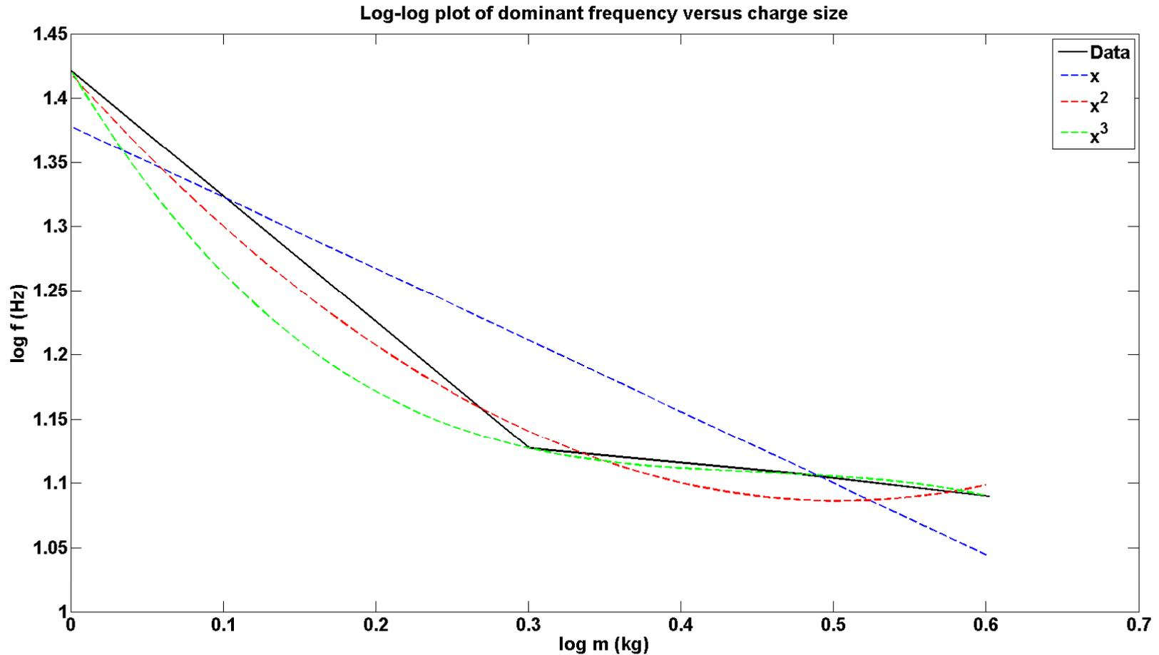
**FIG.8.** Log-log plot of dominant frequency and charge size. A series of polynomial fits which were computed based on the log of the charge size have been superimposed.
