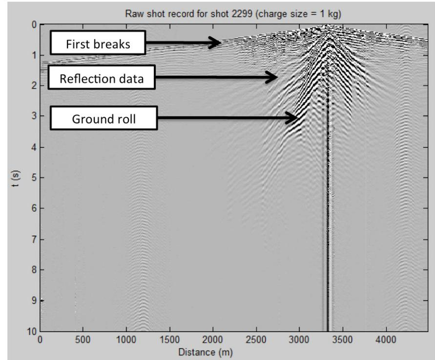
**FIG.1.** Raw shot record showing the individual components of the shot record that were analyzed in this investigation.
