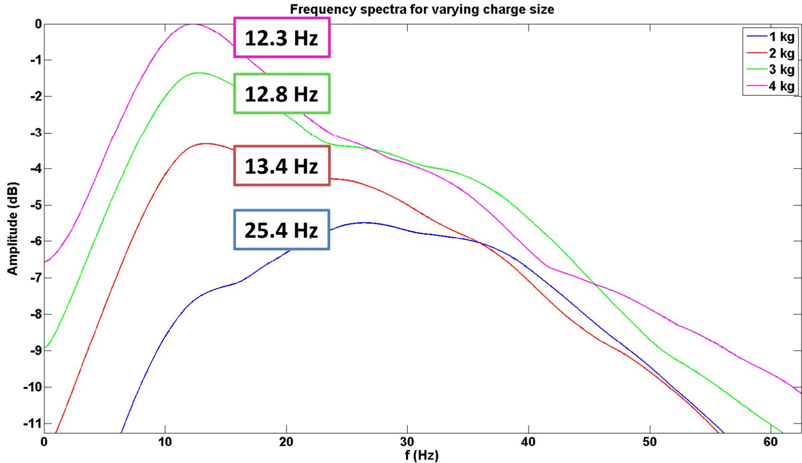
**FIG.7.** Closer view of the peaks in the frequency spectra for the reflection data. The decrease in frequency appears to be most drastic for the 1 and 2 kg charge sizes.
