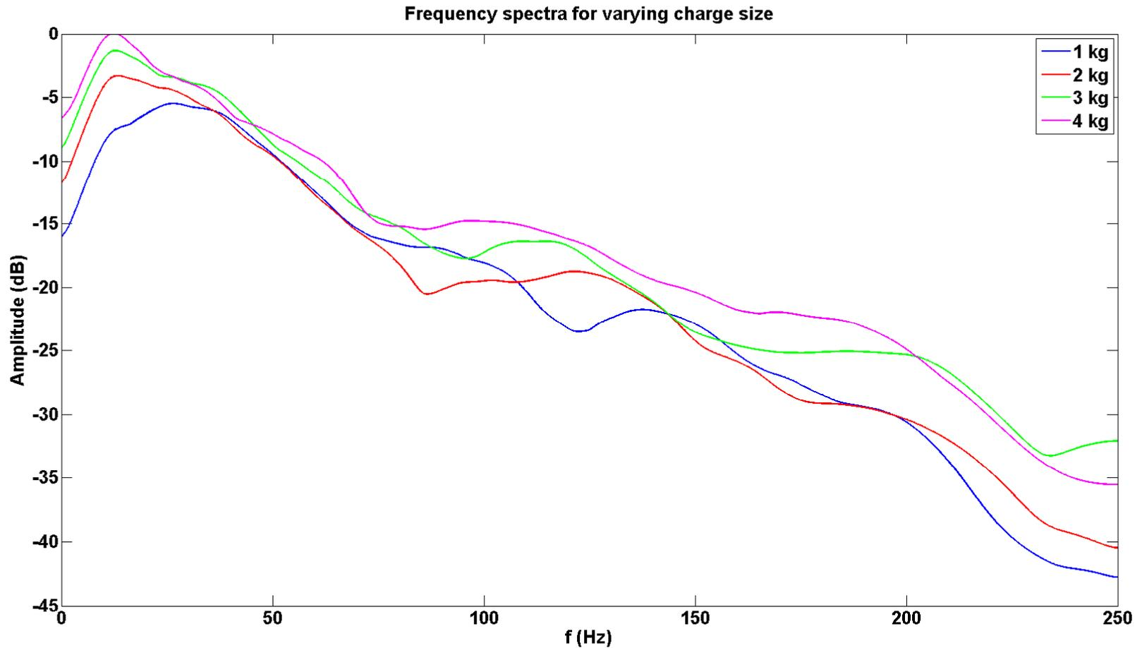
**FIG.6.** Frequency spectra for the reflections that result from different charge sizes. The dominant frequency appears to decrease with increased charge size as predicted by Sharpe, 1942.
