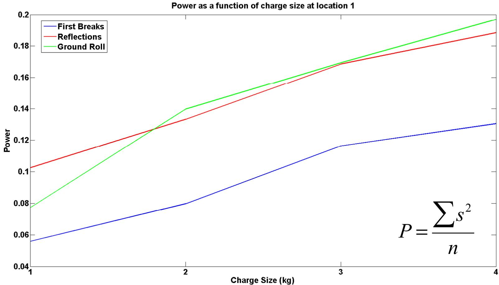
**FIG.3.** Shot power as a function of charge size at location one. The power, and thus displacement amplitude, appears to increase with charge size as predicted by Sharpe, 1942.
