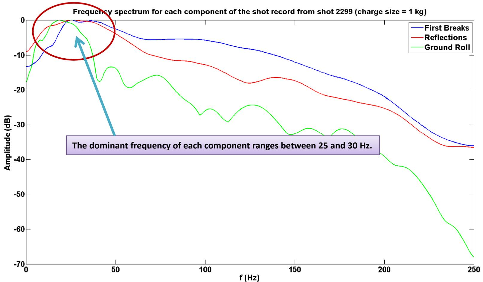
**FIG.4.** Frequency spectra for each of the components of the shot record for shot 2299. These were obtained via the `fxtran_new` code using the time windows for `tmin` and `tmax`.
