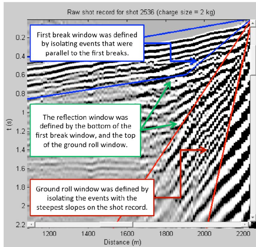
**(Left) FIG.2.** Raw shot record showing the time windows used to isolate each component of the shot record.
