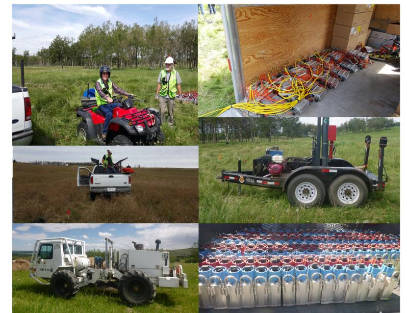
FIG. 2. CREWES using a variety of sources and receivers at the Priddis Test Site.
