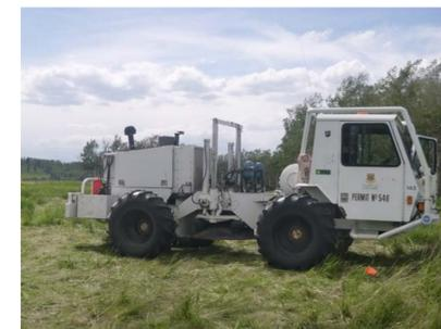
FIG. 5. IVI Envirovibe (sweep 10-200Hz over 16 seconds, two sweeps per source point).
