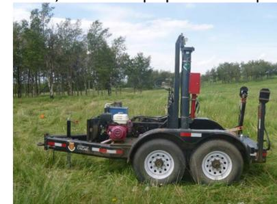
FIG. 6. Shear wave thumper.
