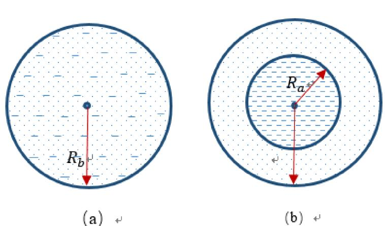
In this model, we assumed that: The seismic wavelength is much larger than the gas pocket size and there is no interaction between two gas pockets(White's assumption), and, there is no movement between fluid 1 and the skeleton, but there is relative movement between fluid 2 and the skeleton.
