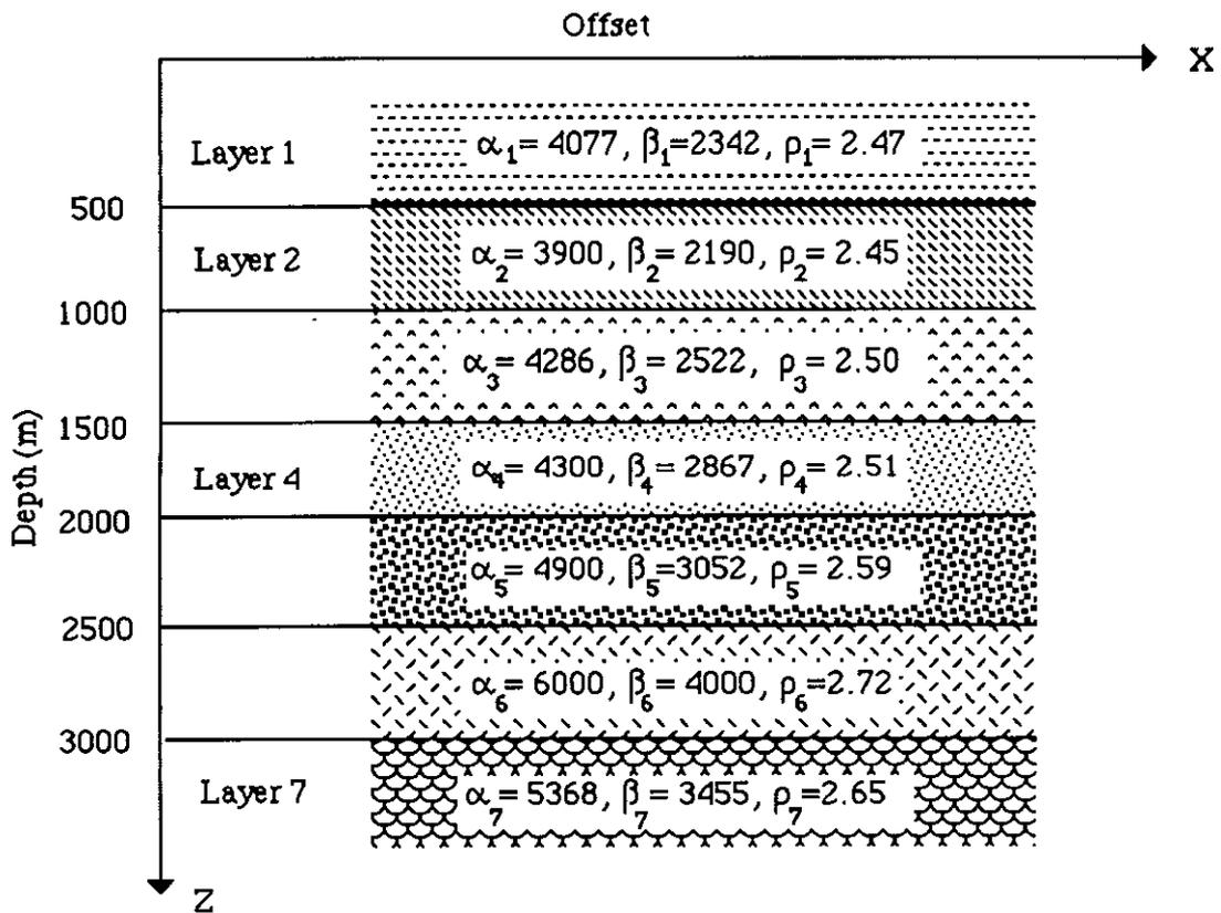
Fig.1: Layered elastic-wave model
