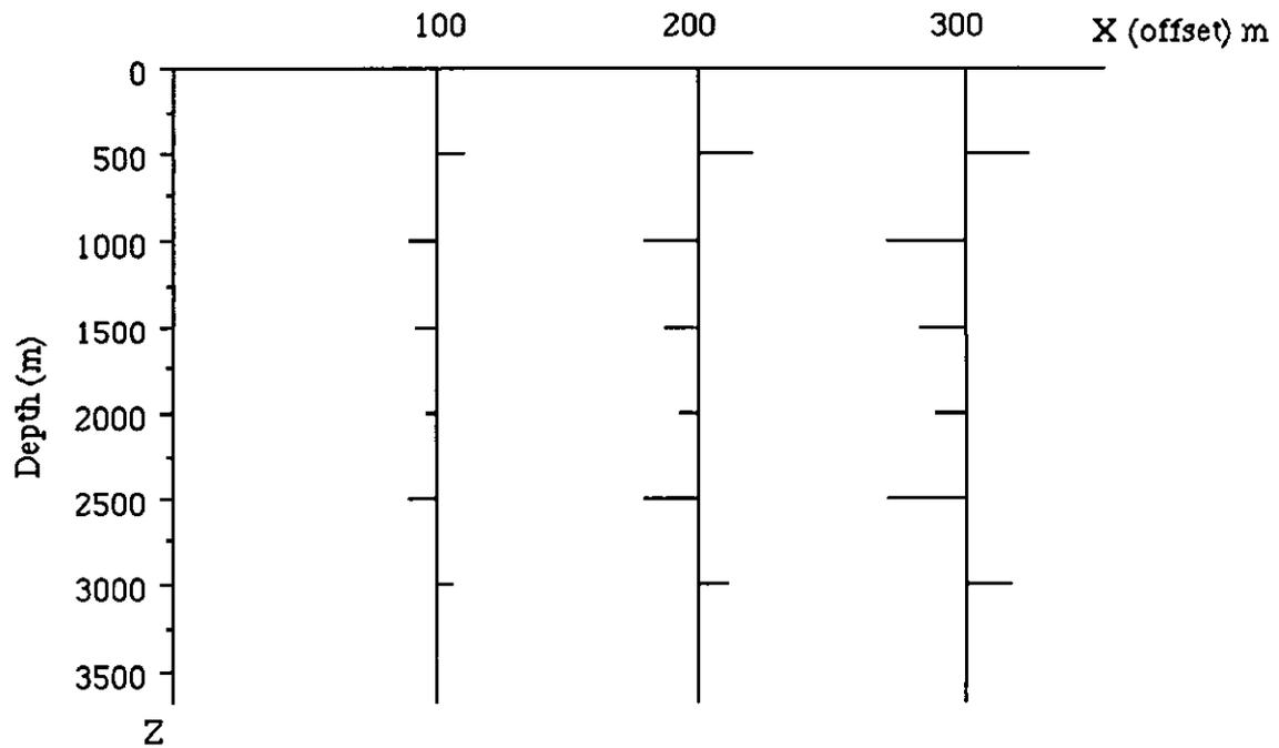
(b): P-SV reflectivity  $R^{PS}$ **FIG.2 : Reflectivity versus offset**
