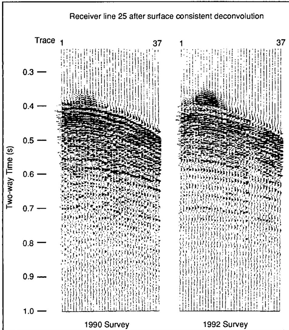
FIG. 5. The same receiver line as in Figure 4, after bandpass filtering, geometric spreading compensation and surface consistent deconvolution.
