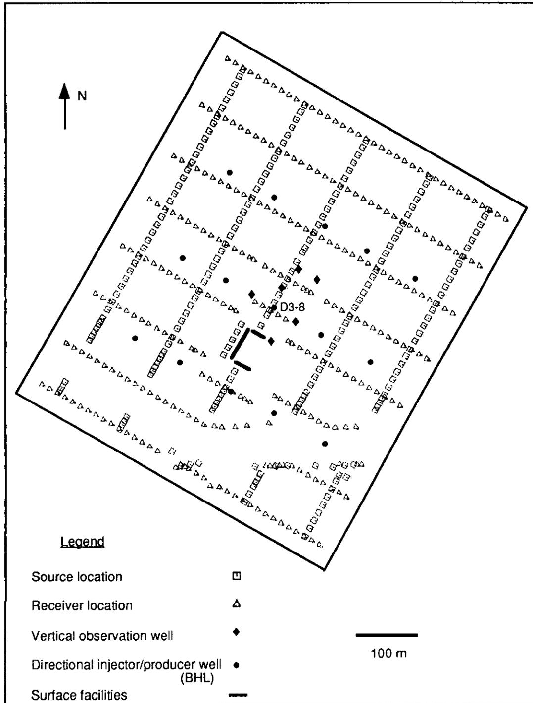
FIG. 3. Layout of seismic grid at the D3 pad.
