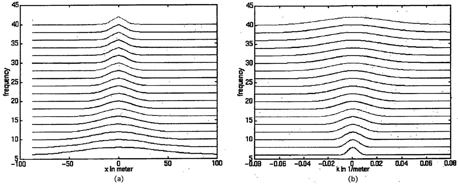
FIG. 4. Schematic diagram of using a gaussian function as a 2-pass 2-D symmetric 3-D f-k filter to reject velocity up to 500m/s. (a) filter in  $\omega$ -x domain. (b) filter in  $\omega$ -k domain.
