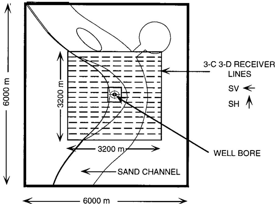
FIG. 7. Schematic diagram showing the 16 receiver lines, the inline and cross line polarizations as well as the well bore.
