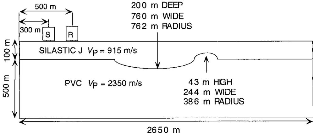
FIG. 11. Schematic diagram showing the two-layer weathering layer model.
