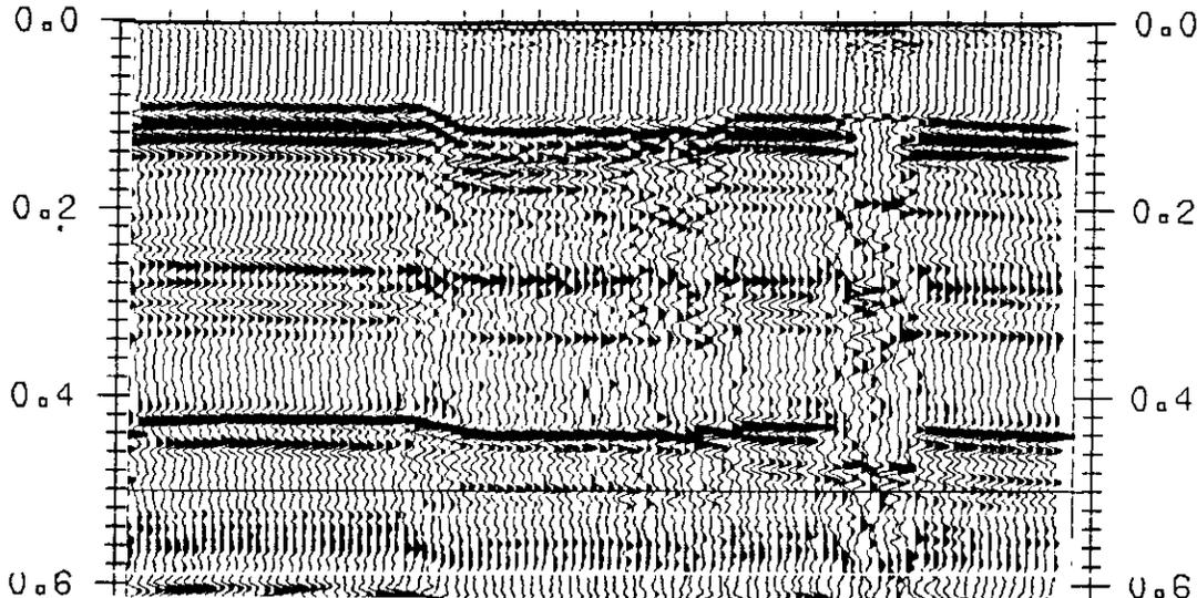
FIG. 10. Rugose model data showing a P-SV survey of line 5.
