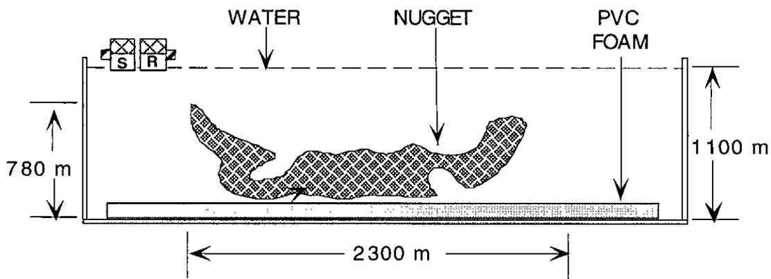
FIG. 5. Schematic showing experimental setup over copper nugget.
