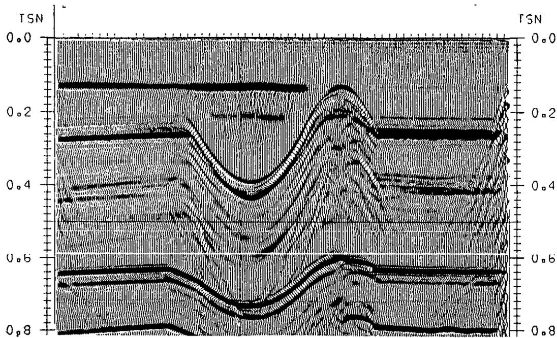
FIG. 12. Constant offset P-P record over the model.
