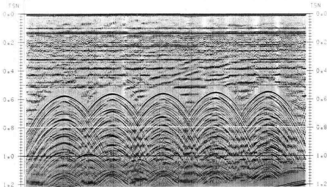
FIG. 16 Data from a constant offset P-P survey across the aluminum rods.
