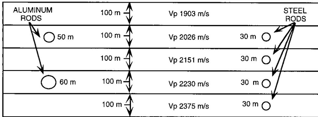
FIG. 1. Schematic diagram of velocity gradient model.
