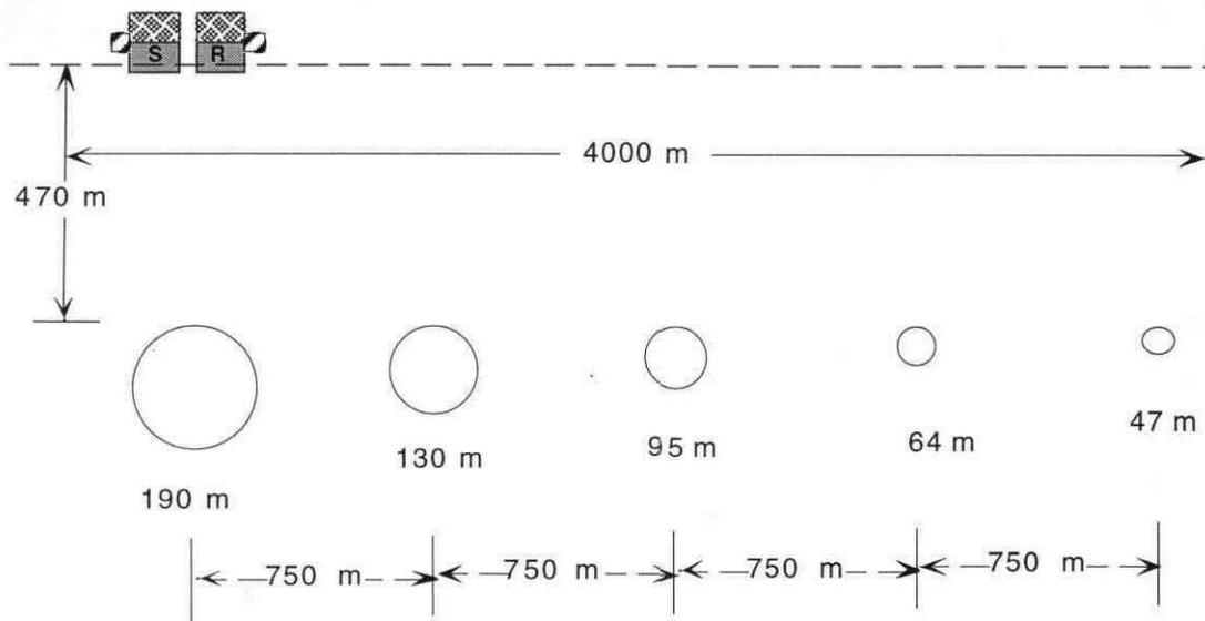
FIG. 15. Schematic diagram of aluminum rod experiment showing the survey geometry.
