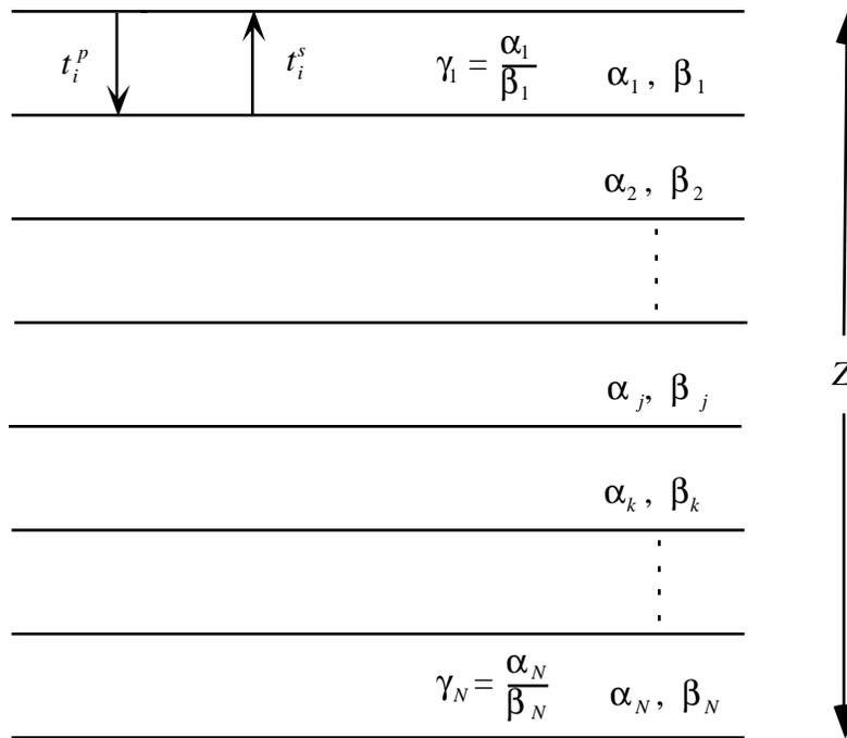
Fig. 1. Plane-layer elastic medium with N layers.
