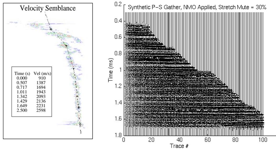
Fig. 6. Semblance velocity analysis of P-S gather. Horizon times and corresponding P-S NMO velocities on left.
