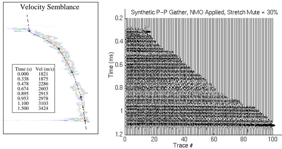
Fig. 5. Semblance velocity analysis of P-P gather. Horizon times and corresponding P-P NMO velocities on left.
