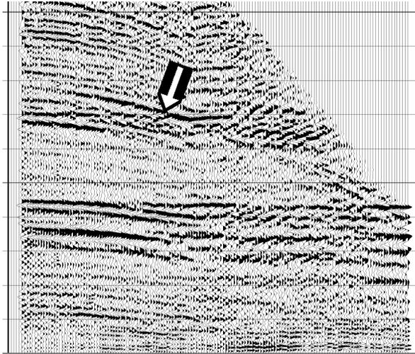
FIG. 6. Illustration of energy concentrated on a hyperbola from a dipping event.
