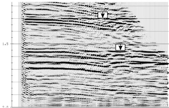
FIG. 3. CSP gather illustrating horizontal events (see arrows) and hyperbolic events forming a prow shape.
