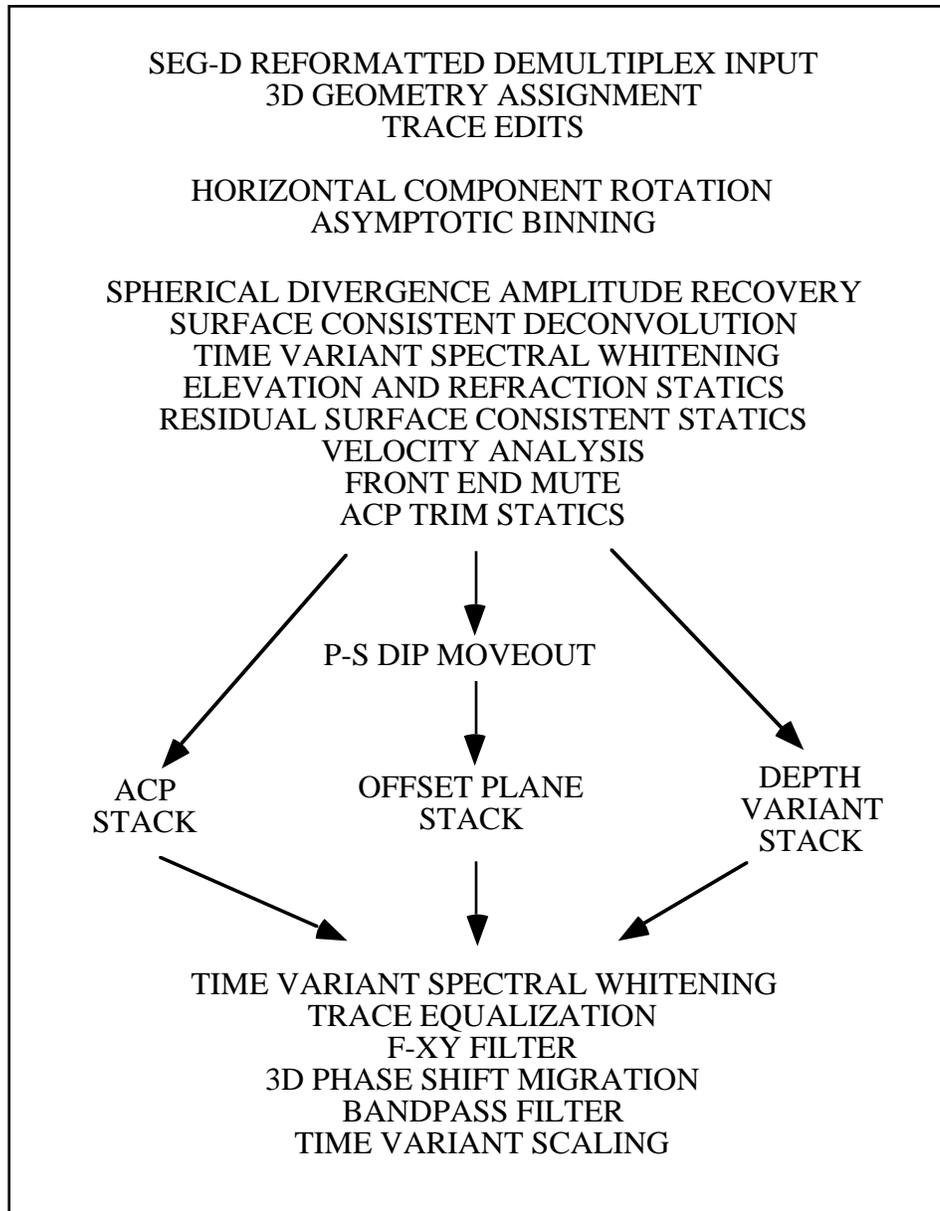
Fig.5. Sensor's radial processing flow for Asymptotic, DMO and Depth Variant binning methods
