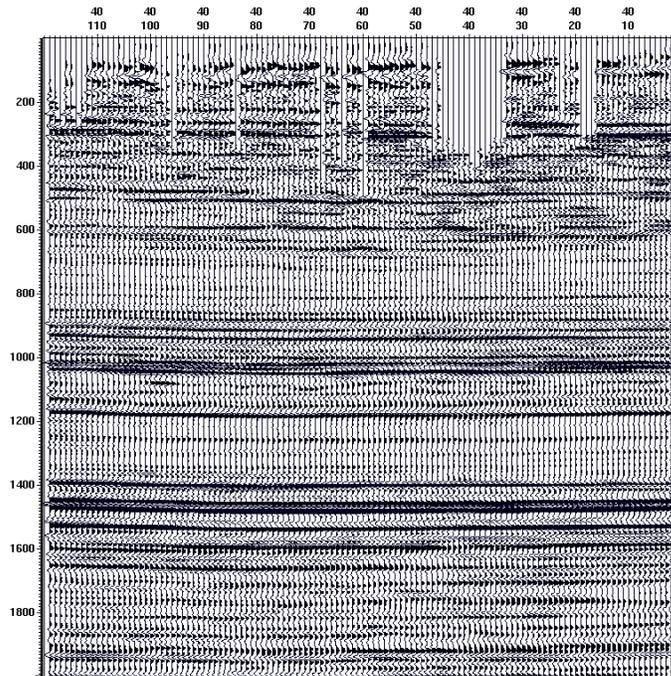
Fig.11. Crossline 40 from Sensor's vertical migrated volume
