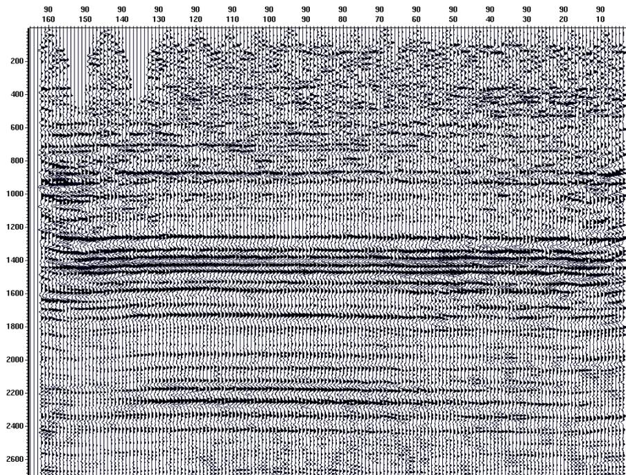
Fig.10. Crossline 90 from Pulsonic's radial migrated volume
