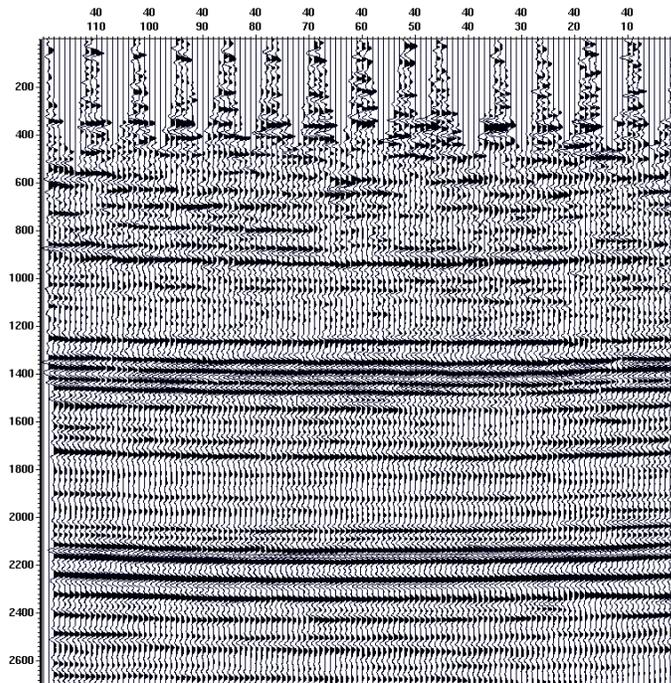
Fig.12. Crossline 40 from Sensor's radial migrated volume
