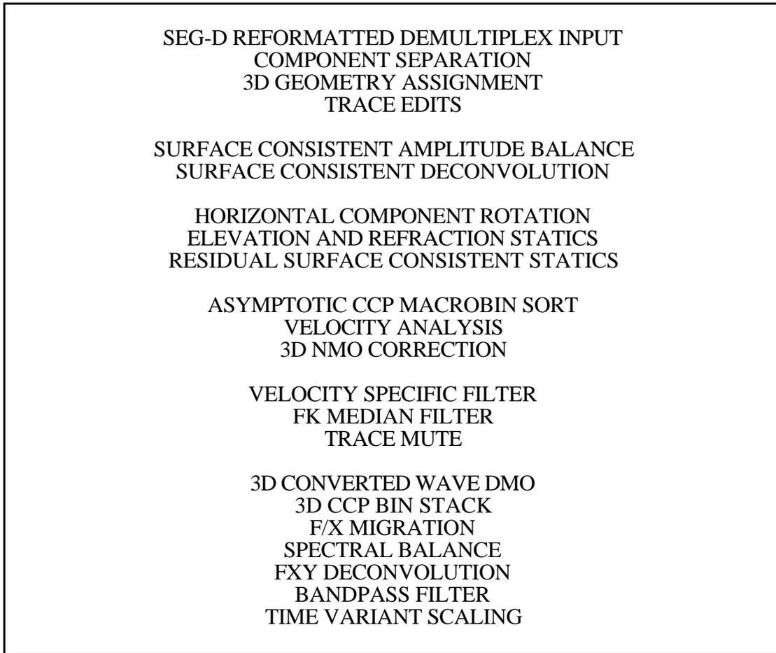
Fig.4. Pulsonic's radial processing flow
