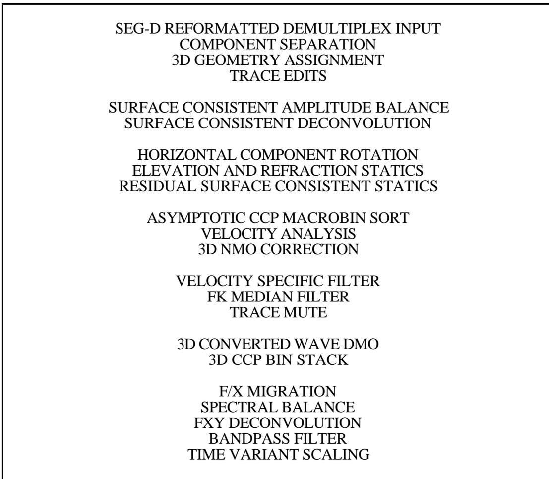
Fig.3. Pulsonic's vertical processing flow
