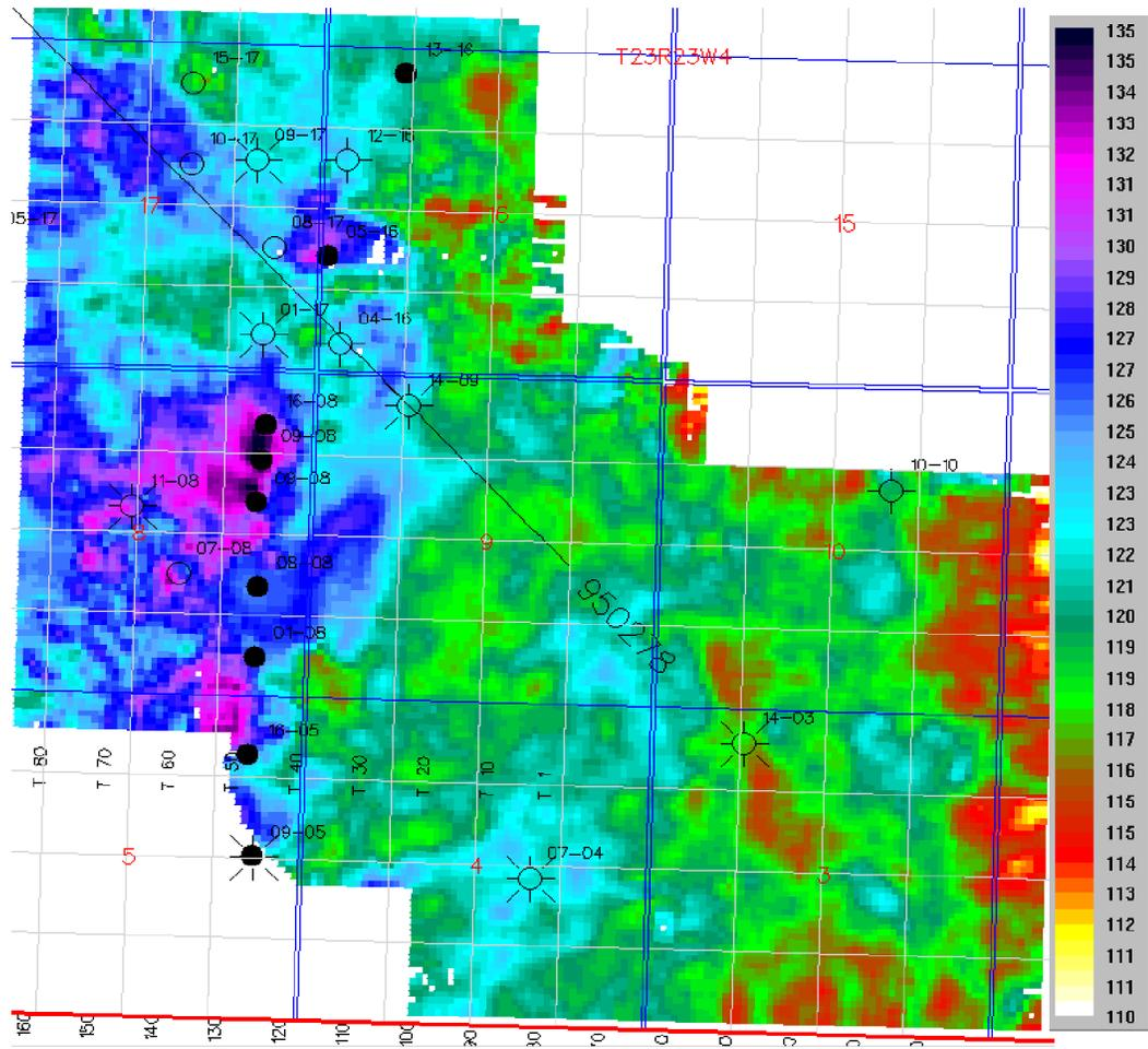
Fig. 16a. *P-P* isochron map from Wabamun to Top channel event. Color bar is traveltime (ms). The red/yellow color of smaller values indicate thinning.
