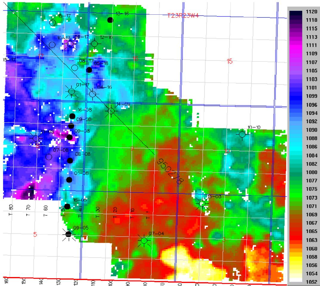
Fig. 7a. P-P time structure, Mississippian event. Color bar is reflection time (ms).
