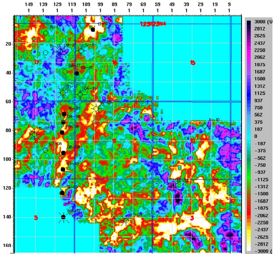
Fig. 12a.  $P$ - $P$  time slice at 1054 ms (flattened at Mannville). This time slice cuts the volume at about the level of the channel. The color bar represents seismic reflection amplitude.
