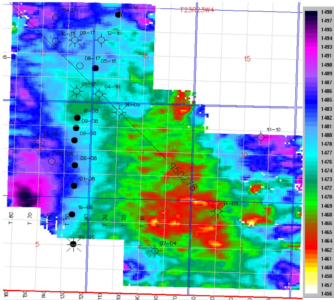
Fig. 11b. *P-S* time structure, Viking event. Color bar is the reflection time (ms).
