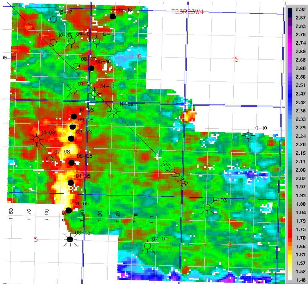
Fig. 18b.  $V_p/V_s$  map, top channel event - Wabamun , showing that the oil wells lie within the smaller  $V_p/V_s$  values of red / green color zone, while the 12-16 and 04-16 dry holes lie within the larger  $V_p/V_s$  value zone of blue color zone
