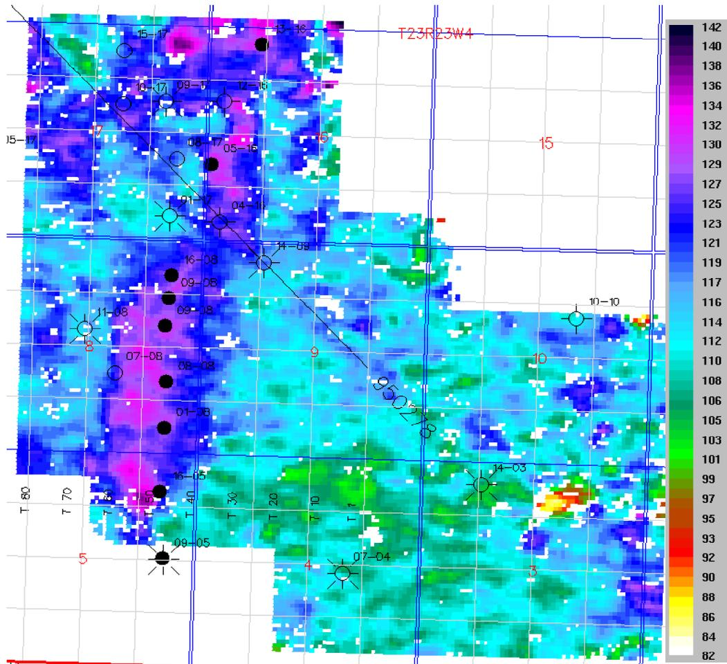
Fig. 17b. P-S isochron map from Mississippian to Mannville event. Color bar is traveltime (ms). The red/yellow color of smaller values indicate thinning.
