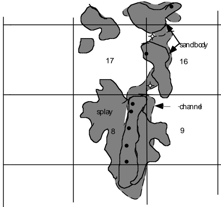
Fig. 20. The interpreted Glauconitic channel sand bodies
