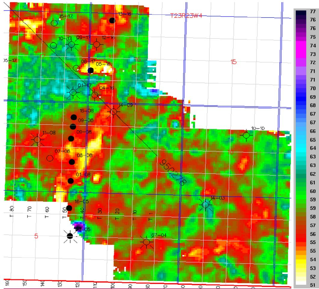
Fig. 14a. *P-P* isochron from Mannville to top channel events. Color bar is traveltime (ms).
