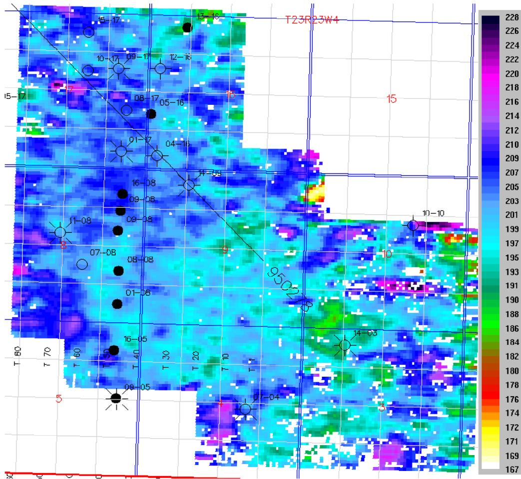
Fig. 15b. *P-S* isochron map from Wabamun to Lower Mannville. Note the thickness trend running north-south direction. Color bar represents traveltime (ms).
