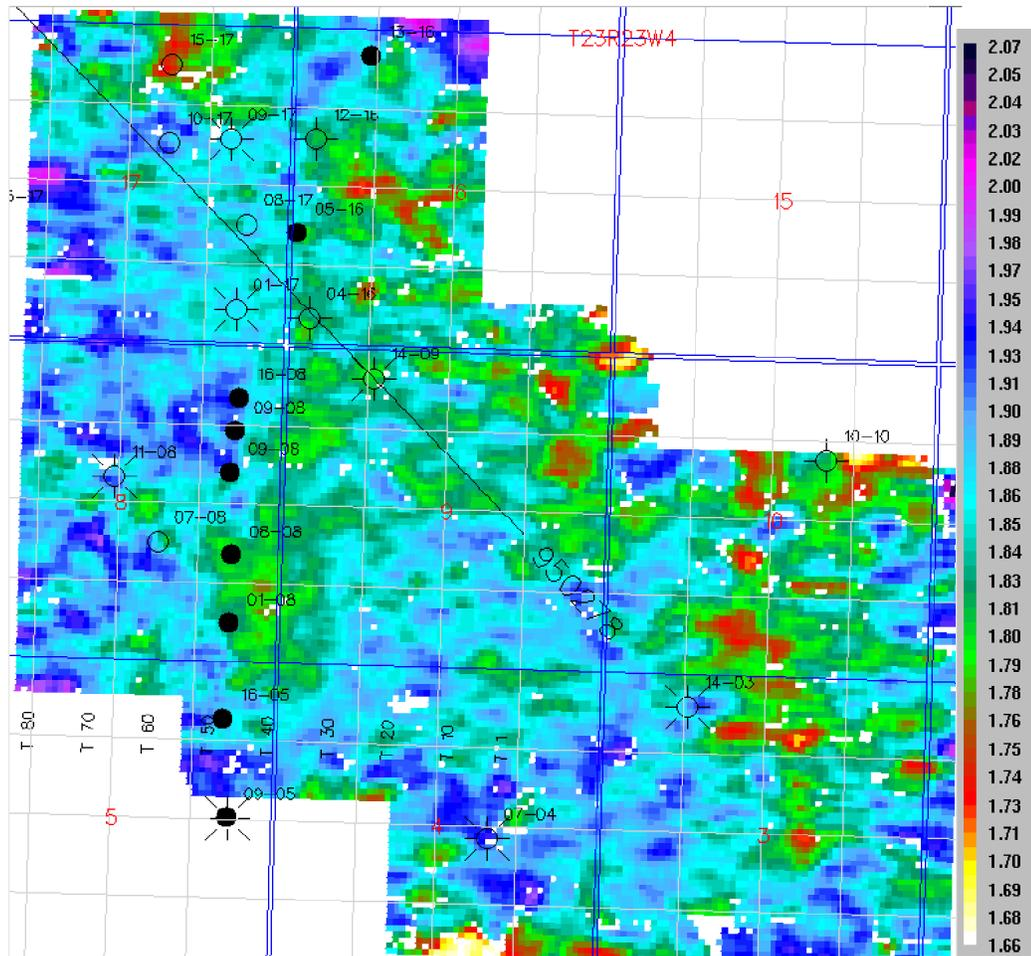
Fig. 18c.  $V_p/V_s$  map, basal Cambrian time - Wabamun , showing lower  $V_p/V_s$  values along the margins of the horst block.
