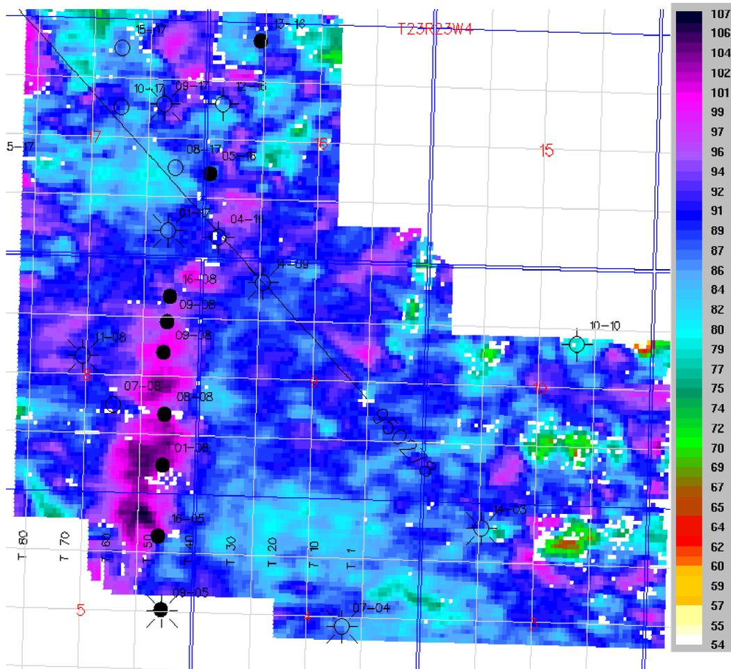
Fig. 14b. P-S isochron from Mannville to Top Channel event. Color bar is traveltime (ms).
