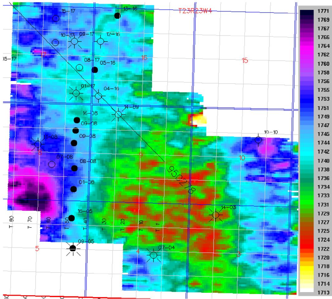
Fig. 6b. P-S time structure map, Wabamun event. Color bar is reflection time (ms).
