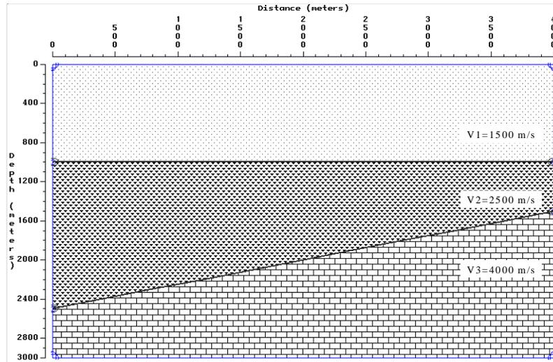
Figure 1: A simple synthetic model
