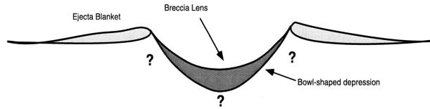
Figure 2a. Schematic of a simple crater (Westbroek and Stewart, 1995)
