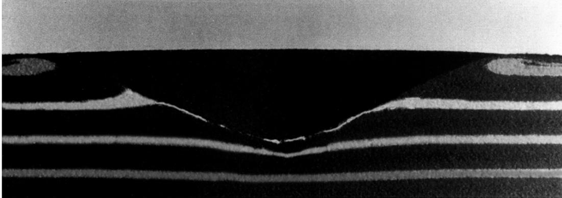
Figure 11. When examined in cross-section, a crater simulated by hypervelocity impact shows many of the morphological characteristics observed in seismic examples of impact structures. (Melosh, 1989)
