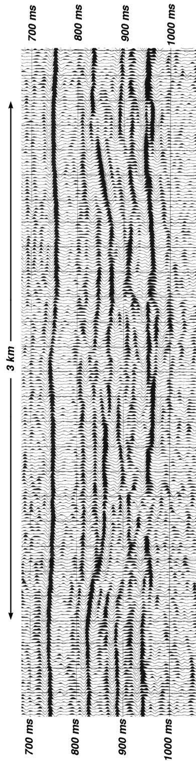
Figure 7. The Muskingum structure in Ohio exhibits the general characteristics of a simple impact crater. The width of the structure is about 3 km.
