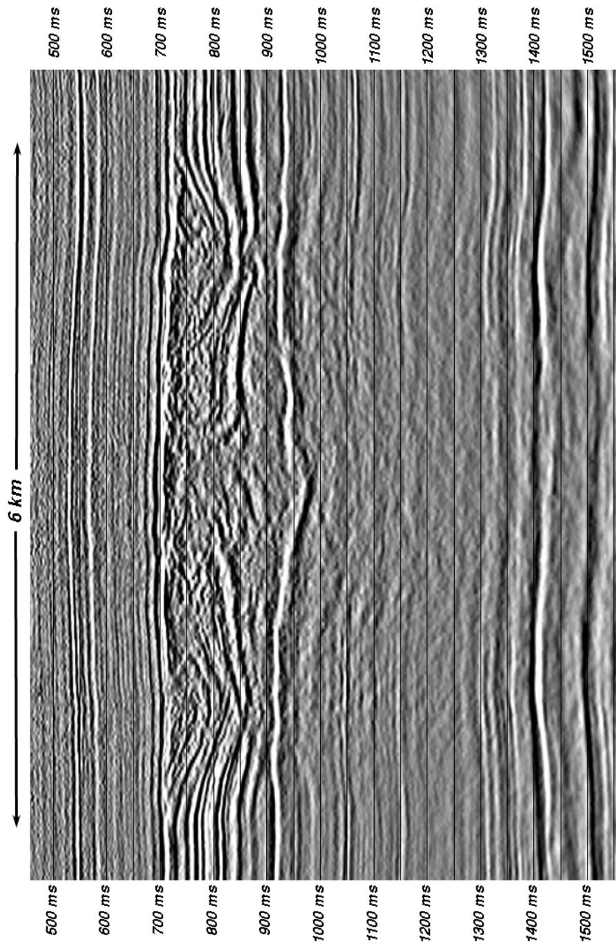
Figure 4. The Hotchkiss structure in northern Alberta shows many of the morphological characteristics that are diagnostic of a small complex impact crater. The structure has a diameter of about 6 km and is similar in appearance to the White Valley structure (Figure 8).
