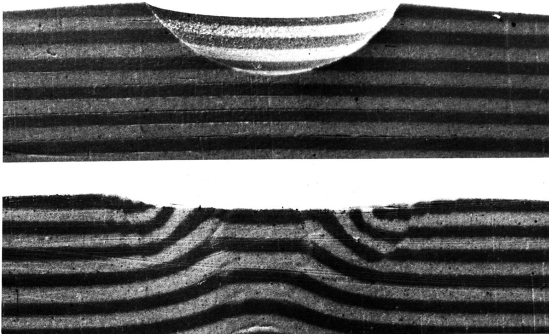
Figure 12. A complex crater can be created by centrifuging a model at gravities of up to 300g. (Melosh, 1989)
