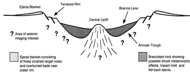
Figure 2b. Schematic of a complex crater (Westbroek and Stewart, 1995)
