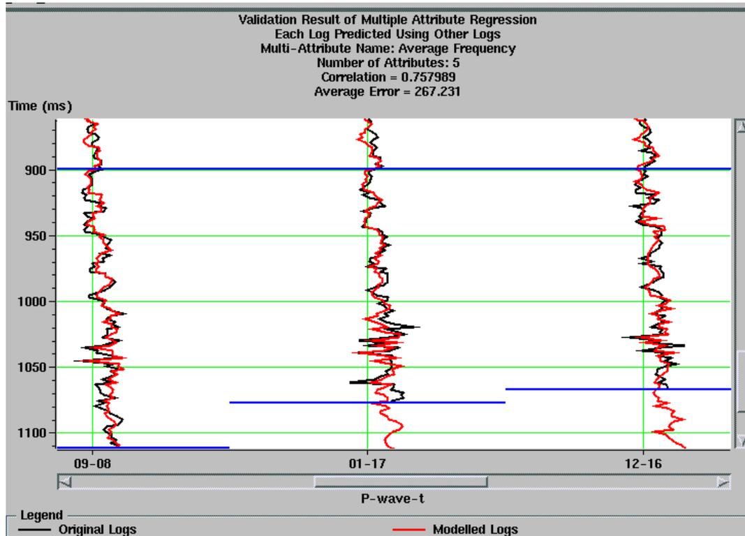
Figure 6: Measured logs (in black) and predicted logs (in red) using convolution operator.
