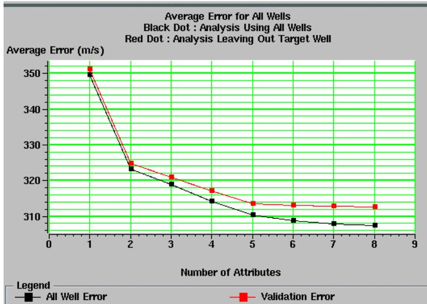
Figure 3: RMS average error vs number of seismic attributes.
