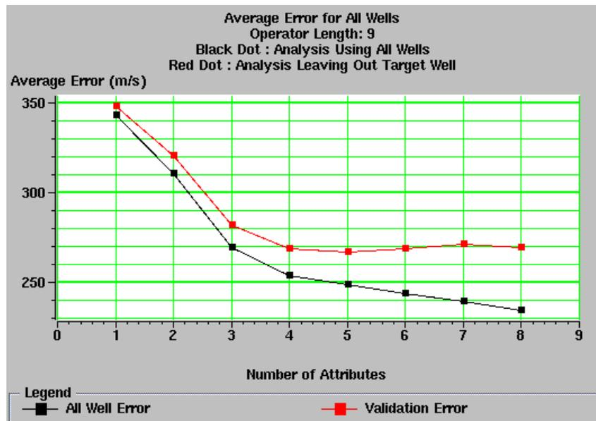
Figure 5: RMS average error vs number of seismic attributes using a convolution operator.
