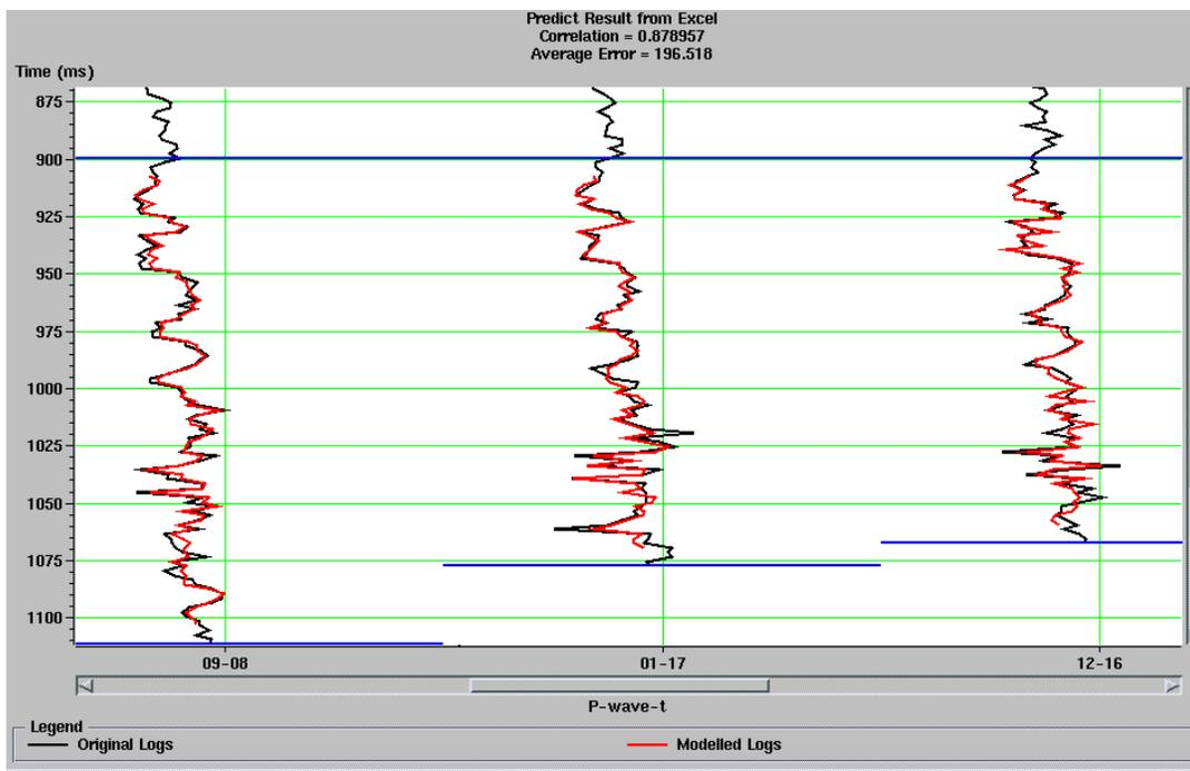
Figure 7: Measured logs (in black) and predicted logs (in red) using a neural network.
