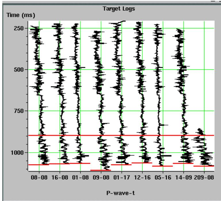
Figure 2: Measured sonic logs in the Blackfoot area.
