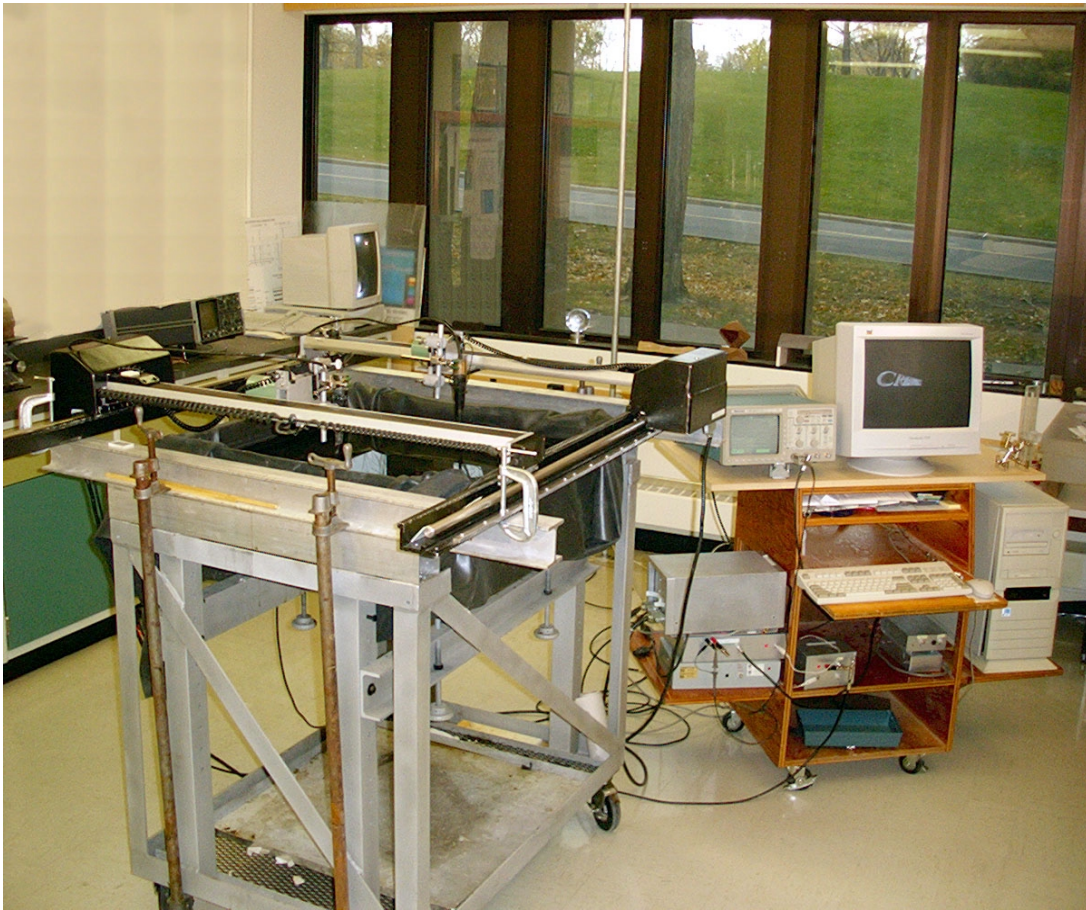
Figure 2. The physical modelling system consists of the modelling jig (left), the computer and electronics systems (right). The configuration above shows a small water tank inserted into the jig aperture to simulate marine surveys.
