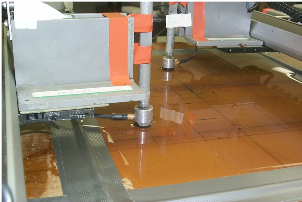
Figure 1. Transducers transmit and receive ultrasonic signals through a physical model during a simulated 3-D seismic survey.
