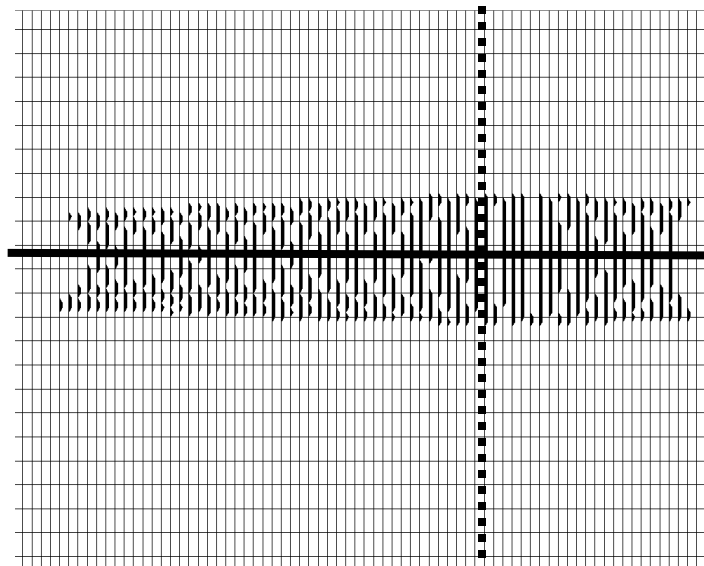
Fig. 8(b). The CCP coverage of the cross-spread in Fig. 8(a). The traces have moved toward the receivers after CCP binning.
