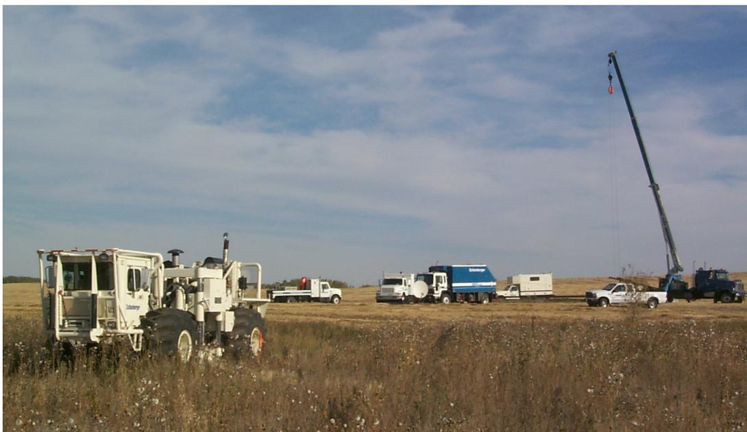
Figure 3. Vertical vibrator at Pike's Peak offset 90 m from the VSP well.
