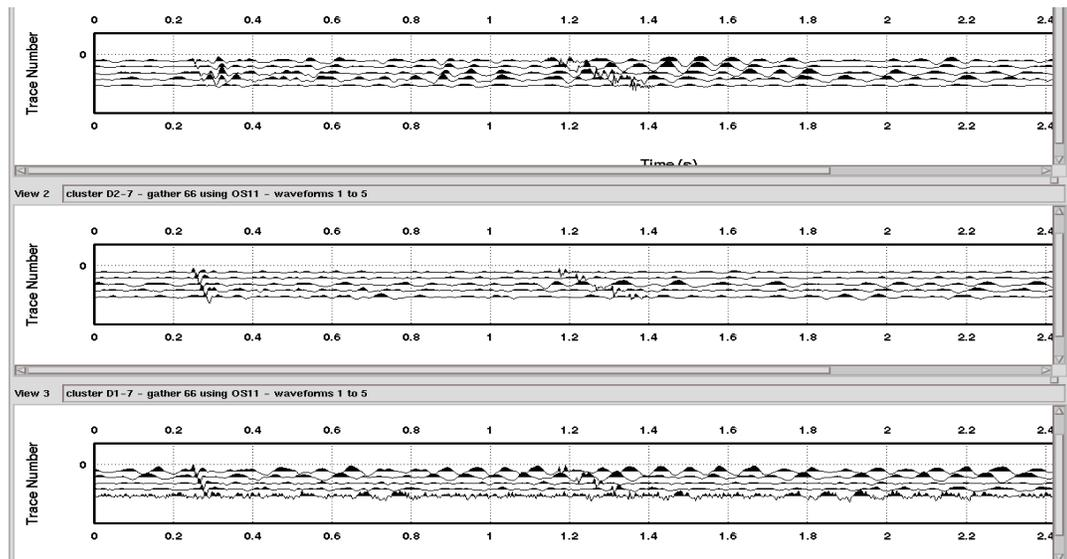
Figure 6. Shot gather records from the lake-bottom survey. The top of the receiving array is 409 m from the recording truck. The top five traces are the vertical (Z) components across the receiver while the next two groups are the horizontal components, Y and X respectively.
