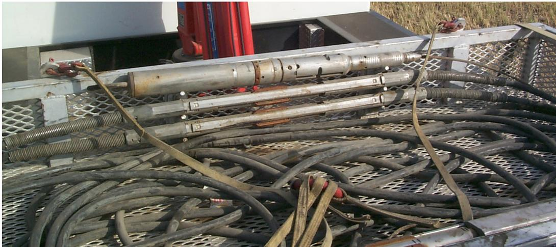
Figure 2. The Schlumberger ASI tool with five shuttles each separated by 15 m and containing a 3-C geophone.
