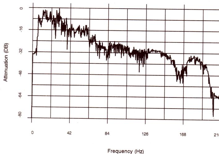
Figure 8. Spectrum from a Y-channel geophone of the lake-bottom cable at a distance 440 m from the recording truck.
