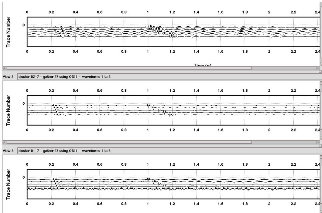
Figure 7. Shot gather records from the lake-bottom survey. The top of the receiving array is 304 m away from the recording truck. The top five traces are the vertical (Z) components across the receiver while the next two groups are the horizontal components, Y and X respectively.
