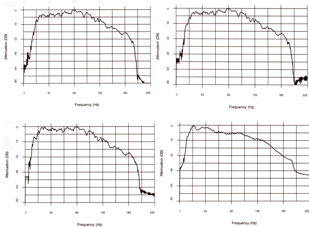
Figure 4. Comparison of geophone spectra at a depth of 515 m for non-linear sweeps: (a) 3 dB/octave, (b) 2 dB/octave, (c) linear. Plot (d) is the spectrum from a linear sweep at a geophone depth of 240 m.
