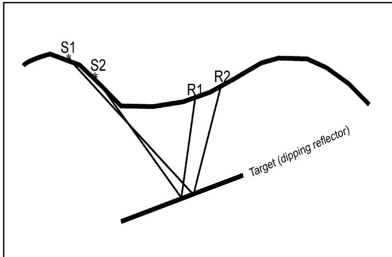
Figure 1. The dipping reflector violates the assumption of common midpoint.
