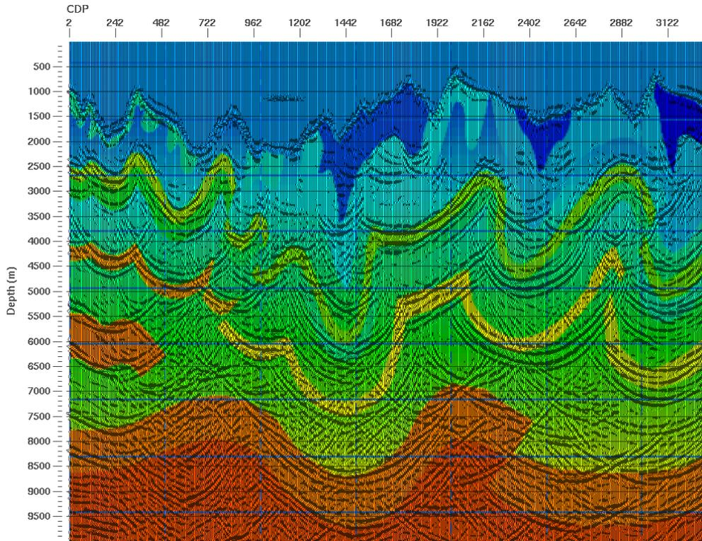
Figure 7. The depth image from pre-stack depth migration from topography is superimposed the correct velocity model. The migration velocity model was derived from stacking velocities (Figure 5b).
