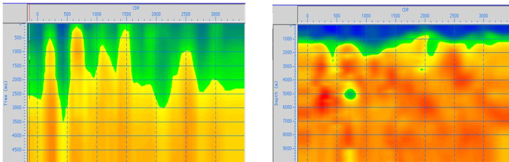
Figure 5 (a) and (b) The stacking velocity is on the left, the smoothed (170 CDP smooth length) interval velocity converted from stacking velocity is on the right.
