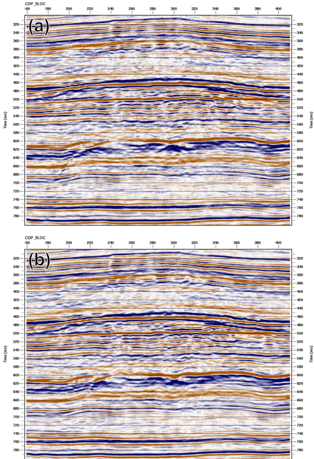
Figure 6. (a) Structure stack of the vertical geophone array P-P data and (b) its post-stack time migration. The data has been windowed between stations 160 – 410 and 300 – 800 ms to encompass the reflectors of the producing Waseca Formation. The top of the Waseca Formation is situated approximately at 450 ms.
