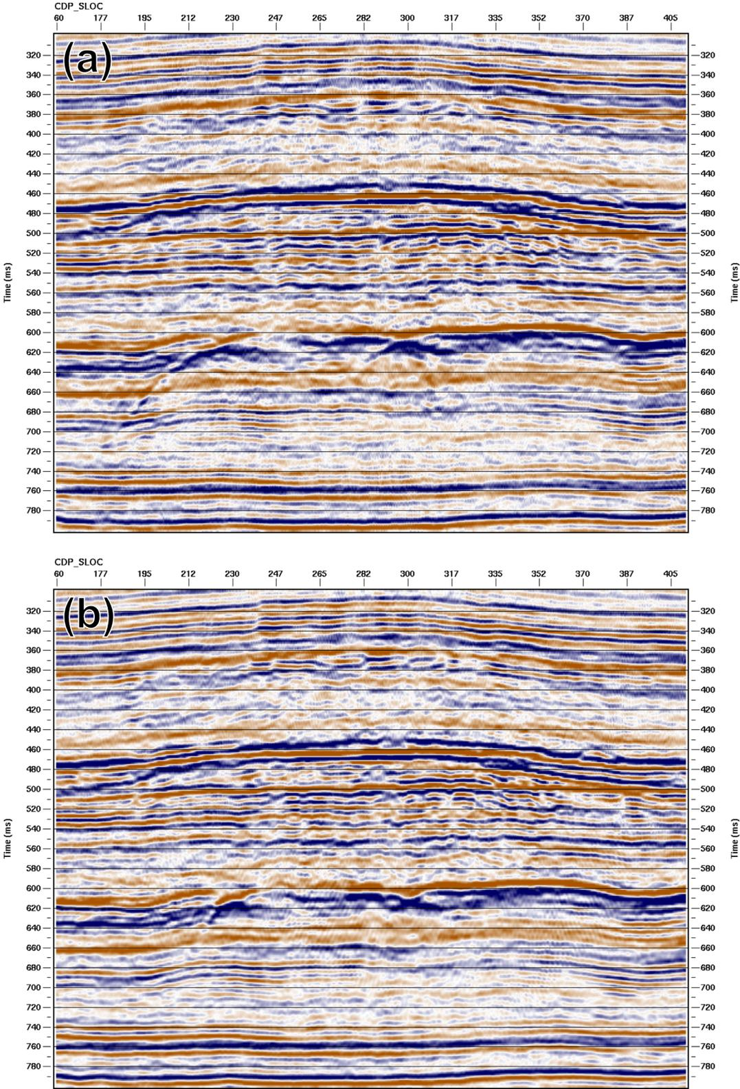
Figure 7. (a) Structure stack of the single vertical component P-P data and (b) its post-stack time migration. The data has been windowed between stations 160 – 410 and 300 – 800 ms to encompass the reflectors of the producing Waseca Formation.
