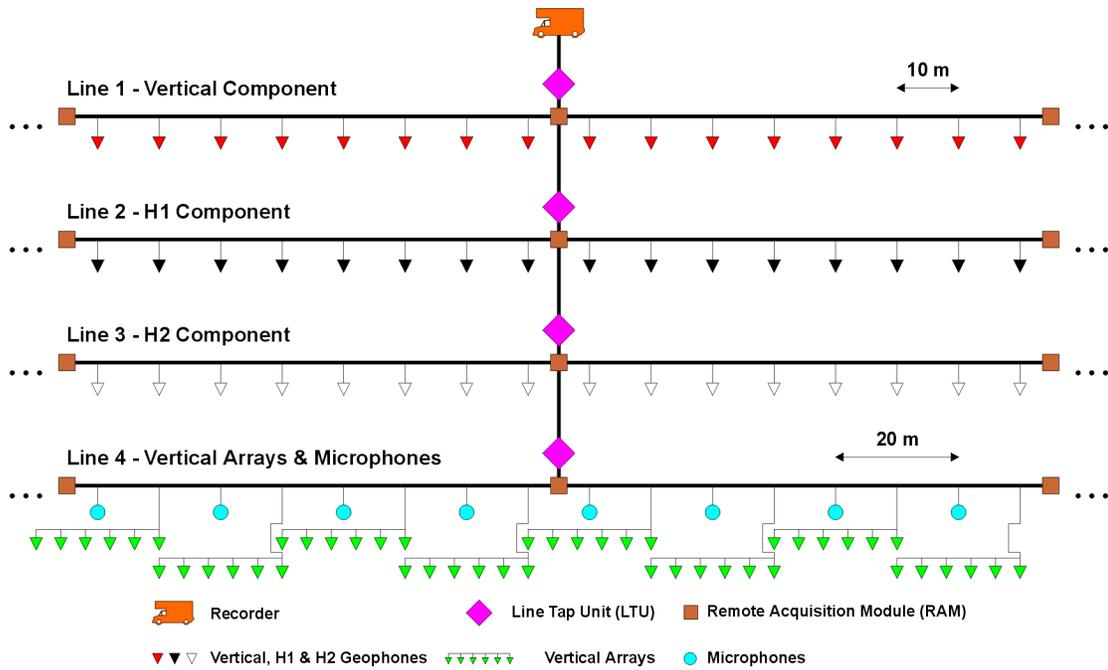
Figure 2. Field layout used for the Pikes Peak 3C-2D survey. Note that the vertical, H1 and H2 components of the 3C acquisition were recorded separately as three distinct receiver lines. The vertical arrays and microphones were assigned to a fourth receiver line.
