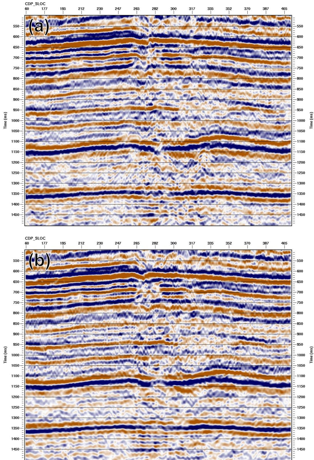
Figure 8. (a) DMO structure stack of the radial component P-S data and (b) its post-stack time migration. The data has been windowed between stations 160 – 410 and 500 – 1500 ms to encompass the reflectors of the producing Waseca Formation. The top of the Waseca Formation is situated approximately at 950 ms.
