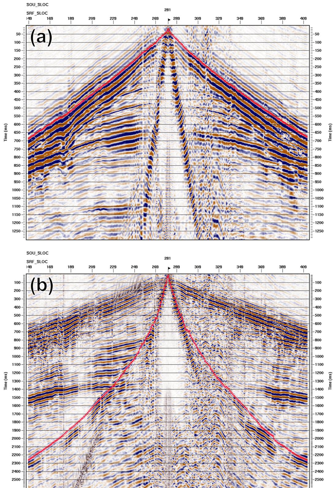
Figure 3. Selected source gathers for (a) vertical component data and (b) radial component data. Travel-time picks of the P and S refracted wave on (a) and (b) respectively is indicated in red. These travel times were used to compute the P-wave source statics and S-wave receiver statics of the P-S refraction statics solution.
