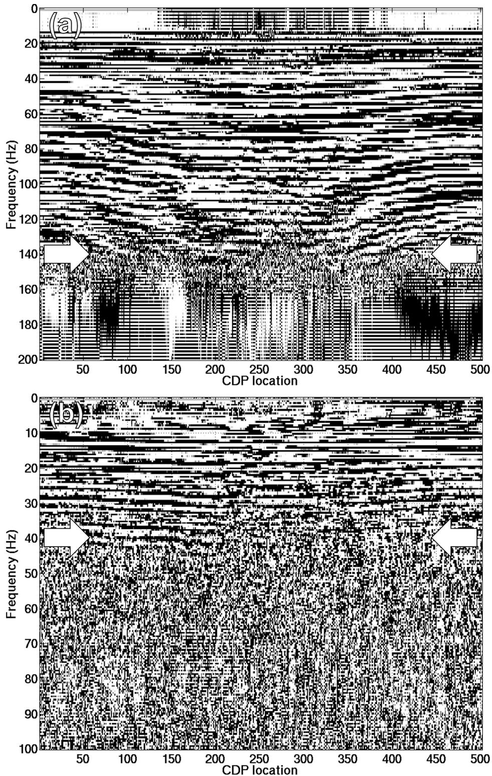
Figure 9.  $f$ - $x$  phase spectra of (a) the structure stack of the vertical component P-P data and (b) the DMO structure stack of the radial component P-S data. The input stack data used to compute the phase spectra have been windowed as per Figures 7 and 8. The white arrows indicate the frequency limit of the maximum coherent phase which is  $\sim 140$  Hz for (a) and  $\sim 40$  Hz for (b).
