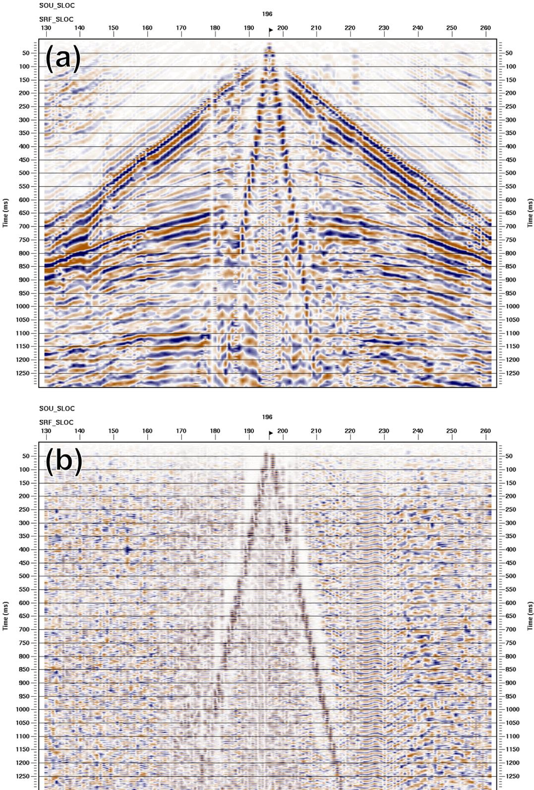
Figure 5. Common source gathers for (a) vertical geophone data decimated from the vertical component of the 3C geophones and (b) microphone data. Note that the air blast (~ 330 m/s) is the dominate energy on the source gather of the microphone data.
