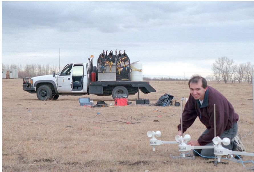
FIG. 2. Three anemometers were setup at the field site to monitor wind speed. Once configured, the anemometers were distributed around the periphery of the test area (visible in the background) and adjusted to stand 30cm above the ground.
