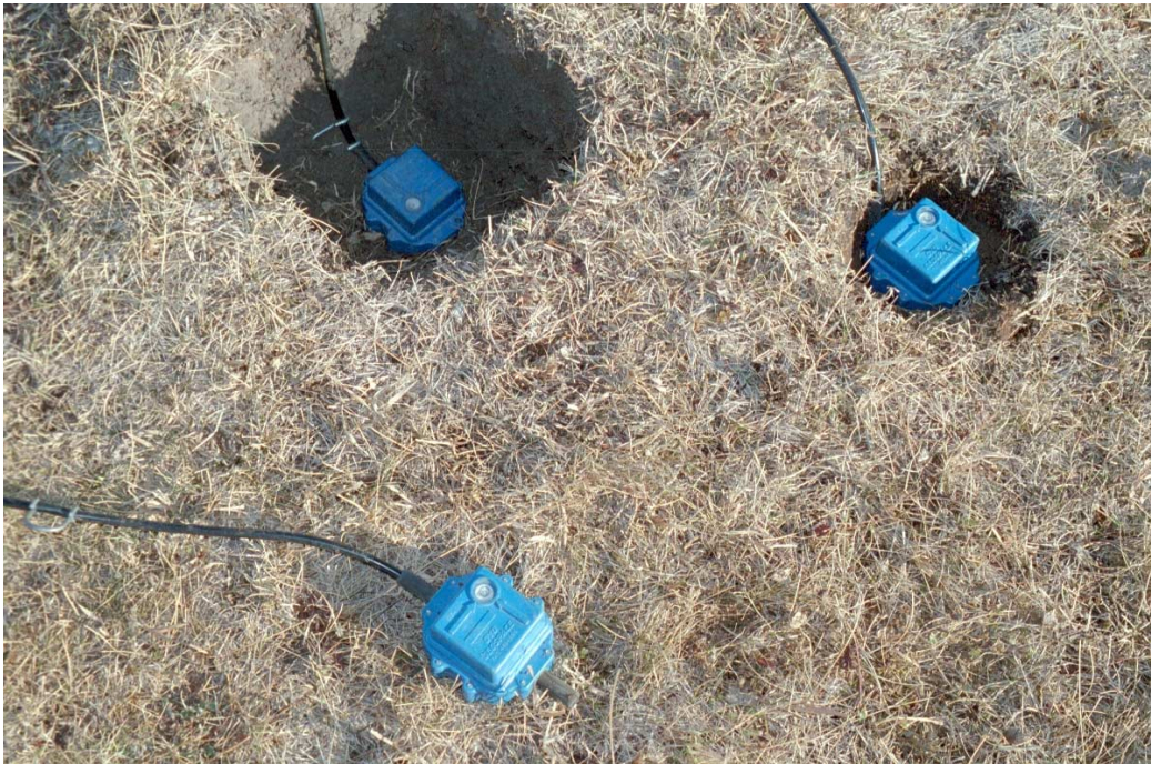
FIG. 11. Geophones were placed on the surface, and buried in holes of different depths. The figure shows holes of 18cm (top), 5 cm (right), and 0 cm (bottom).
