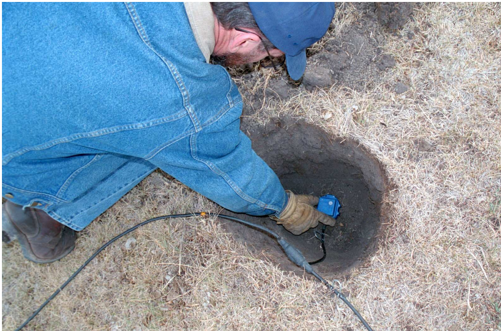
FIG 12. A 3-C geophone is carefully leveled at the bottom of a 48cm hole. This hole took approximately 10 minutes to dig with a shovel. The soil was naturally compacted clay, leading to relatively easy digging. The hole must be dug with care, so as to finish with a flat, undisturbed base at the bottom.
