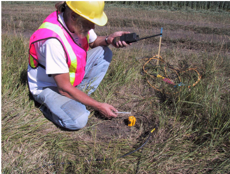
FIG. 2. Two people must coordinate their efforts to successfully record a tap test. The tapper (shown above) goes to a tap test station and stands on the receiver line facing the next bigger geophone station number. Once oriented, the tapper taps the geophone, and calls-in the tap direction and geophone station number. The recorder manually triggers the instruments and makes note of the tap test details.
