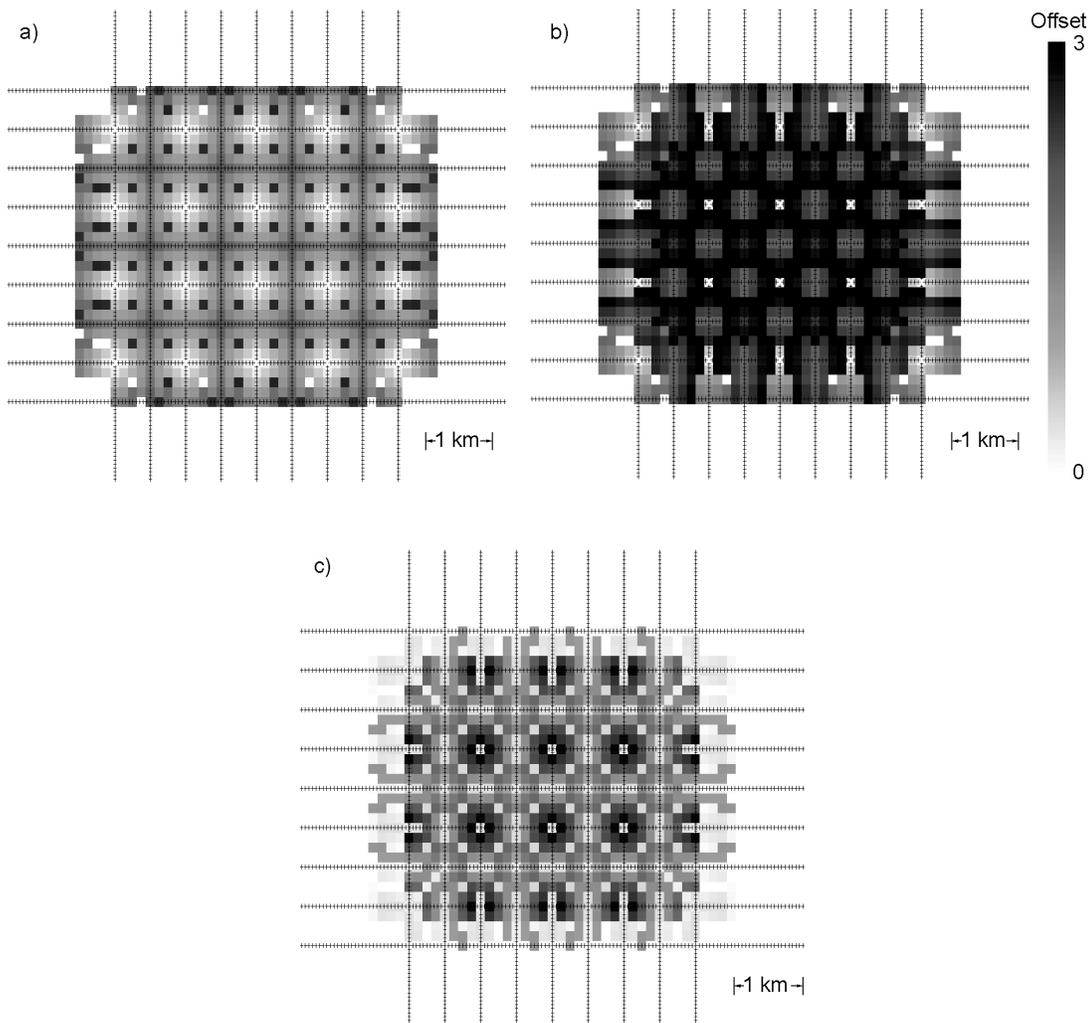
FIG. 7. Near offsets (Figure 7a), Far offsets (Figure 7b) and Offset Range (Figure 7c) for Design 2 with a 125 m bin size, P-S depth specific binning for  $V_p/V_s = 2.0$ .
