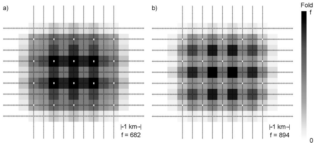
FIG. 3. Design 2. Shot interval is 50 m, receiver interval is 1000 m, water column is 120 m, target depth is 3000 m, source-receiver offsets are limited to 3000 m, and bin widths are 500x500 metres (source line spacing by half receiver spacing). Figure 3a) P-P fold. Figure 3b) P-S depth specific fold for  $V_p/V_s$  of 2.0.
