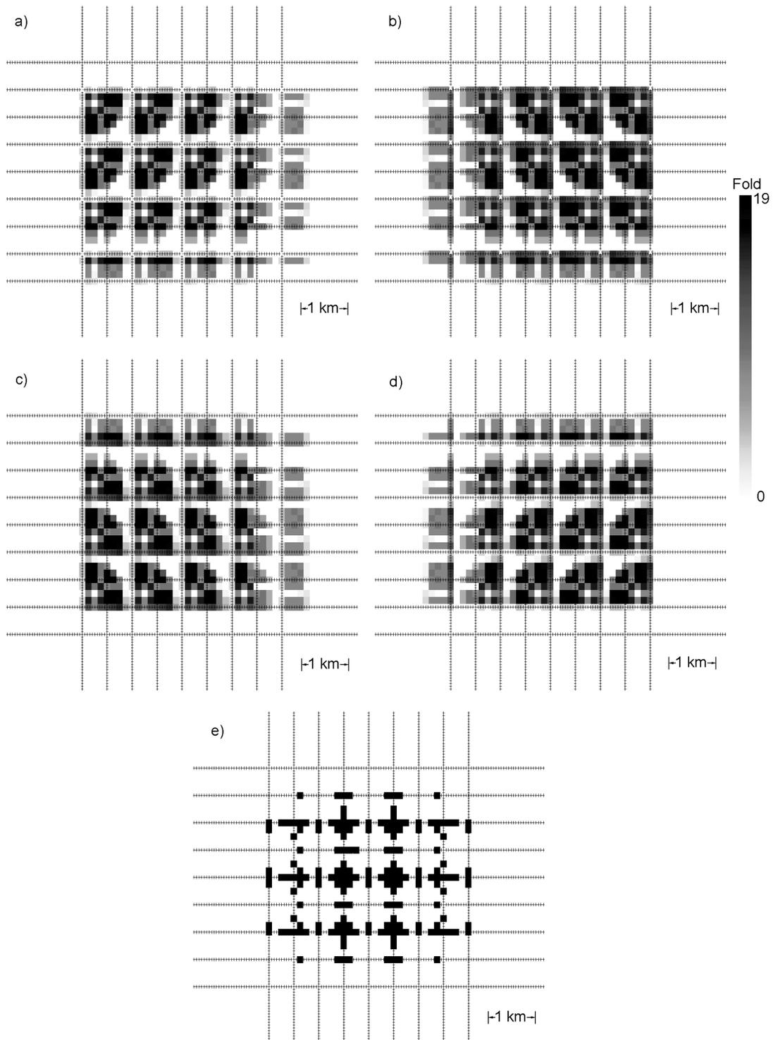
FIG. 8. P-S azimuth distribution for Design 2 with a 125 m bin size. Figure 8b) 0-90 degrees, Figure 8d) 91-180 degrees, Figure 8c) 181-270 degrees, and Figure 8a) 271-360 degrees. Figure 8e) shows bins with full azimuth range (intersection of Figures 8a-8d).
