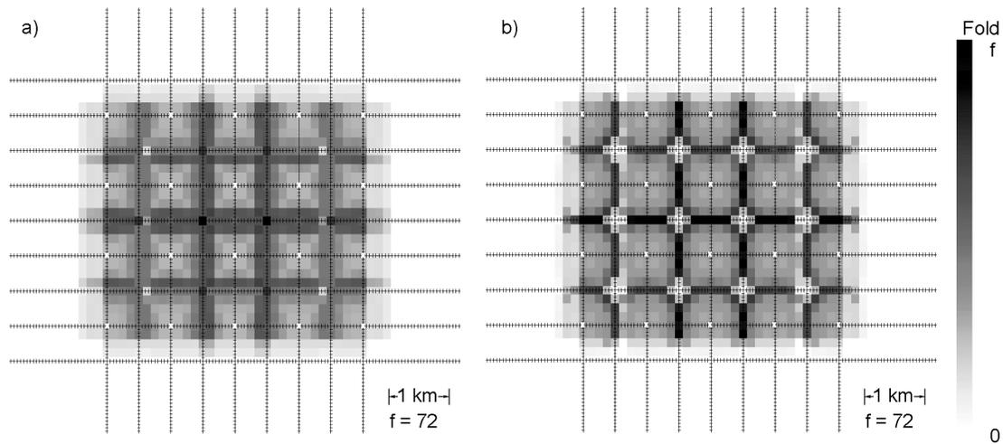
FIG. 6. Effect of increasing  $V_p/V_s$  for Design 2 with 125 m bins.  $V_p/V_s = 2.0$  (Figure 5b),  $V_p/V_s = 2.5$  (Figure 6a).  $V_p/V_s = 3.0$  (figure 6b).
