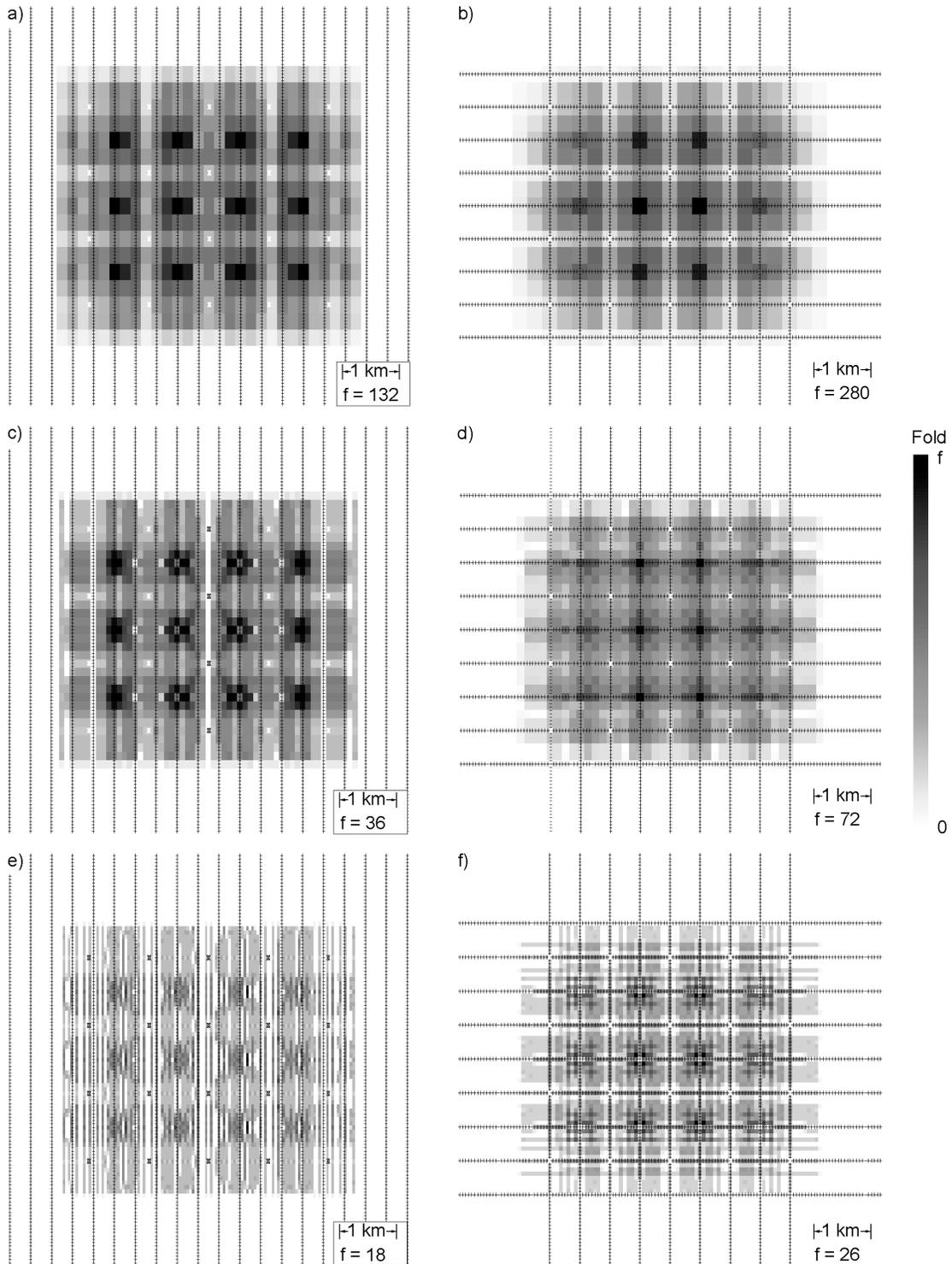
FIG. 4. Effect of decreasing bin size. Figures 4a ( $175 \times 250 \text{ m}^2$ ), 4c ( $87.5 \times 125 \text{ m}^2$ ) and 4e ( $43.25 \times 62.5 \text{ m}^2$ ) show P-S depth specific fold for Design 1 (compare with Figure 2b). Figures 4b ( $250 \times 250 \text{ m}^2$ ), 4d ( $125 \times 125 \text{ m}^2$ ) and 4f ( $62.5 \times 62.5 \text{ m}^2$ ) show P-S depth specific fold for Design 2 (compare with Figure 3b).
