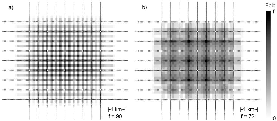
FIG. 5. Comparison of P-P (Figure 5a) and P-S fold (Figure 5b is same as Figure 4d) for Design 2 with 125 metre bins. Compare with Figure 3.
