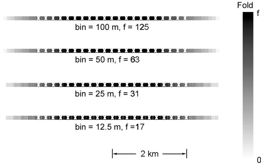
FIG. 1. Effect of bin size on P-S depth specific fold for 2D design with shots every 25 m (shots not shown), receivers every 200 m (white X's). Parameters: 120 m water column,  $V_p/V_s$  of 2.0, Source-receiver offsets limited to 3000 m.  $f$  is maximum fold.
