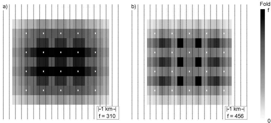
FIG. 2. Design 1. Shot interval is 50 m, receiver interval is 1000 m, water column is 120 m, target depth is 3000 m, source-receiver offsets are limited to 3000 m, and bin widths are 350x500 metres (source line spacing by half receiver spacing). Figure 2a) P-P fold. Figure 2b) P-S depth specific fold for  $V_p/V_s$  of 2.0.
