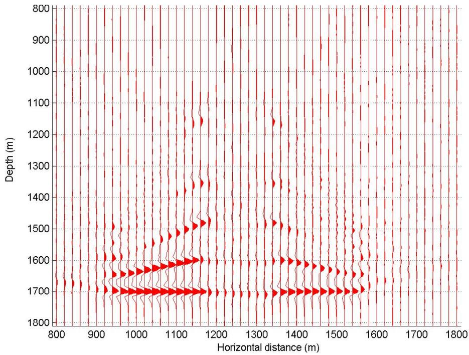
FIG. 7b. Migrated section (model 1) using shots every 400 m, from SP101 to SP105 and SP123 to SP127.
