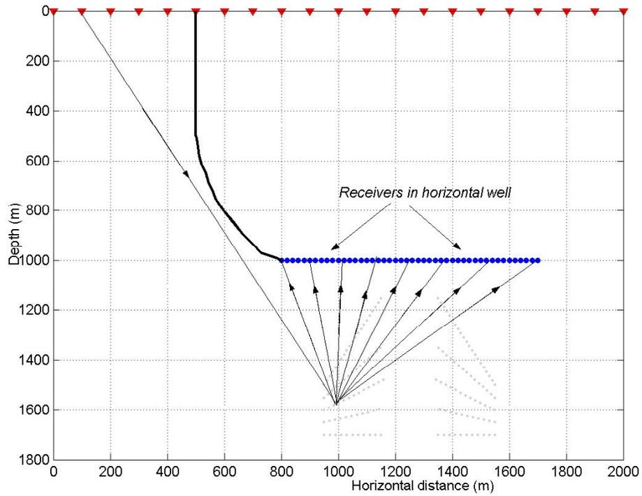
FIG. 1c. Diagram showing scattered energy coming from one of the SP102 rays.
