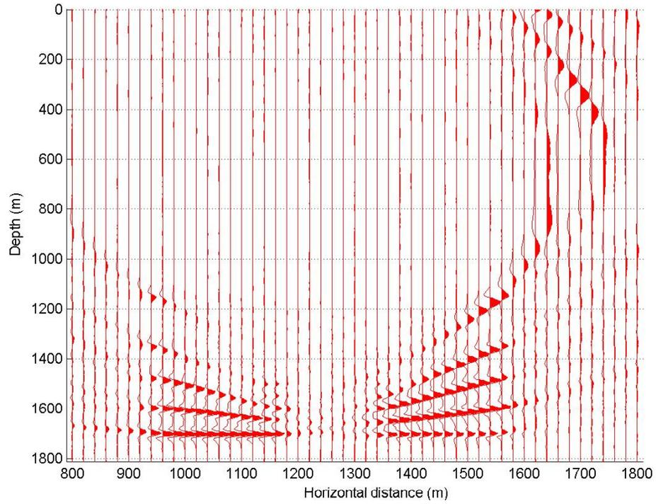
FIG. 4b. Migrated section (model 2) using shots every 800 m, from SP101 to SP127. Notice the low fold residual energy on the right side of the image.
