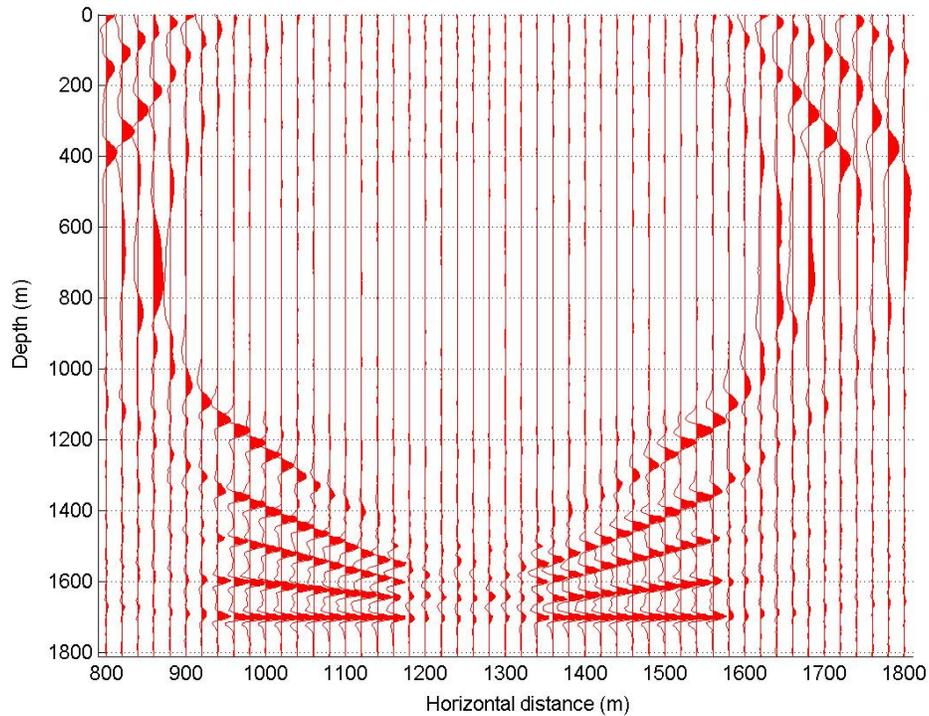
FIG. 8b. Migrated section (model 2) using shots every 400 m, from SP101 to SP105 and SP123 to SP127.
