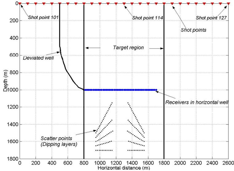
FIG. 1a. Walk-away VSP model 1. A string of 46 receivers is used on the horizontal well.
