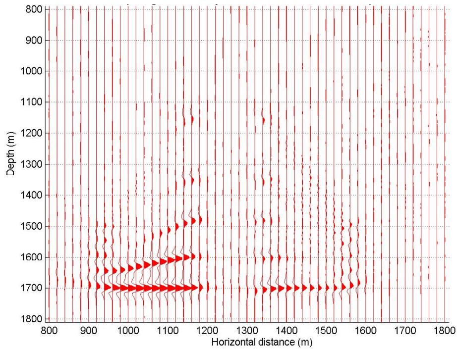
FIG. 5a. Migrated section (model 1) using shots every 400 m, from SP101 to SP114.
