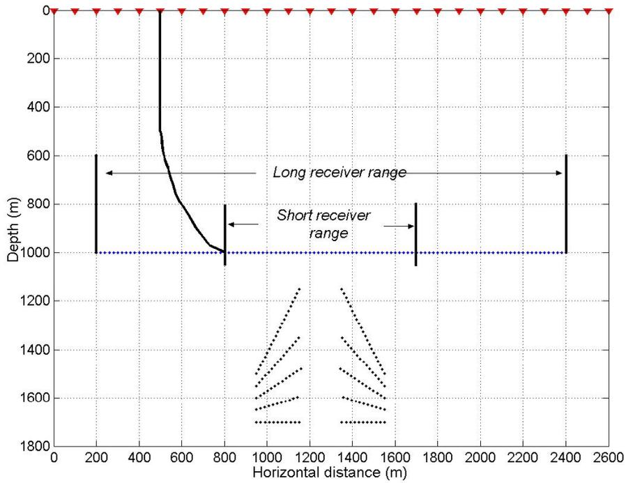
FIG. 9a. Model using a longer receiver range (65 additional sensors were used). Notice that the spread of receivers is longer to the right side respect to the scattering points centre (5 more receivers).
