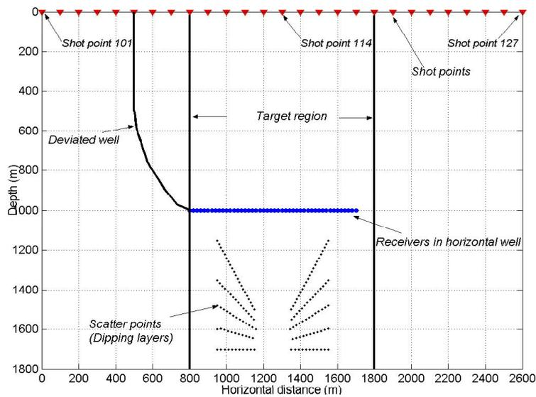
FIG. 1b. Walk-away VSP model 2. A string of 46 receivers is used on the horizontal well.
