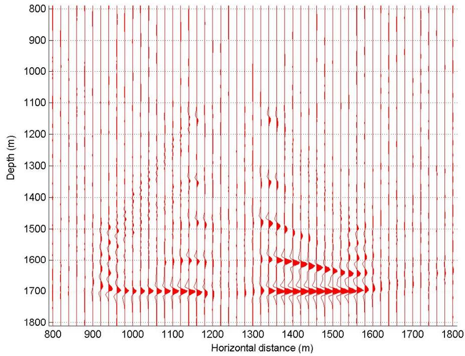
FIG. 5b. Migrated section (model 1) using shots every 400 m, from SP114 to SP127. Reasonable no signal arrival recorded due to geometry of the rays.
