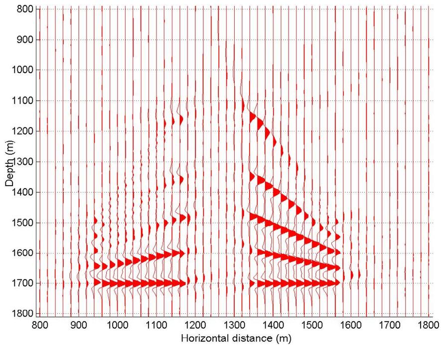
FIG. 9b. Migrated section obtained when more receivers are included in the model. Observe how the reflectors to the right side of the model (where there are more receivers) are better imaged.
