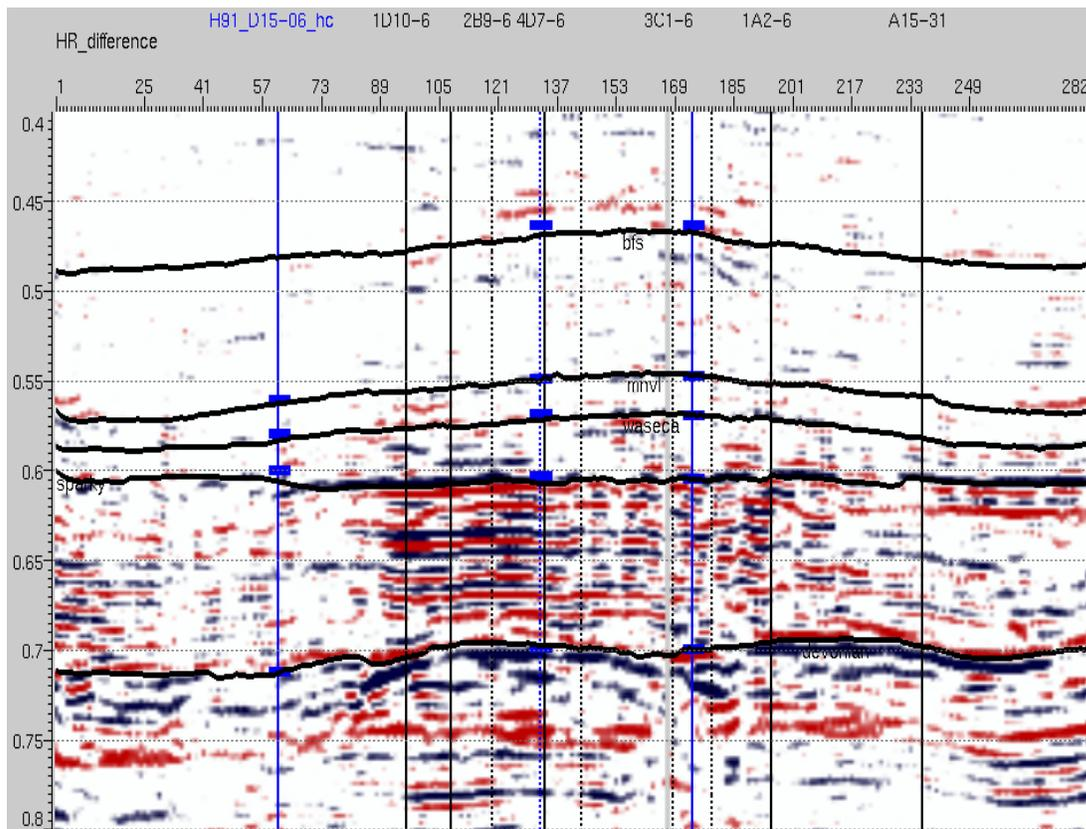
FIG. 1 Seismic amplitude difference section from Watson and Lines (2001). Time window is from 0.4 to 0.8 s over a distance of 2.81 km with trace spacing of 10 km.
