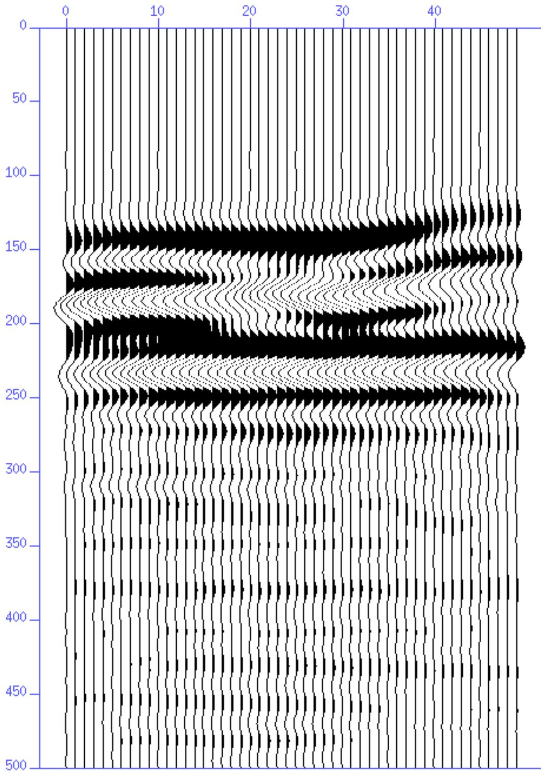
FIG. 3. Zero-offset seismic section for the wormhole model. Traces are at 10 m spacing and at offsets 50 m to 550 m and the vertical axis is in ms. The dominant frequency is 35 Hz.
