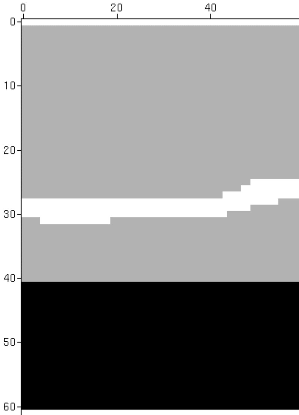
FIG. 2. Velocity "mega-wormhole" model for a highly porous sand with low velocities of 1677 m/s (white), embedded in porous sands of 1923 m/s (grey), overlying a carbonate of 2500 m/s (black). The model is a 60 by 60 array of cells of size 10 m by 10m.
