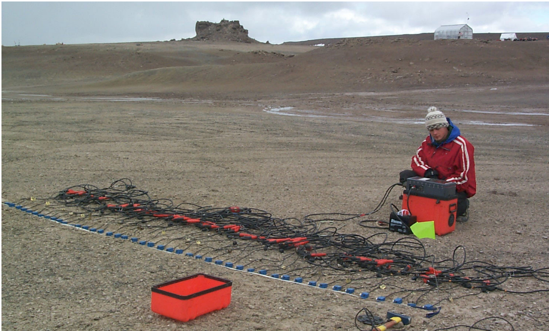
FIG. 1. Vertical receivers deployed in the Von Braun Valley, with student R. Birch checking the seismic recorder.
