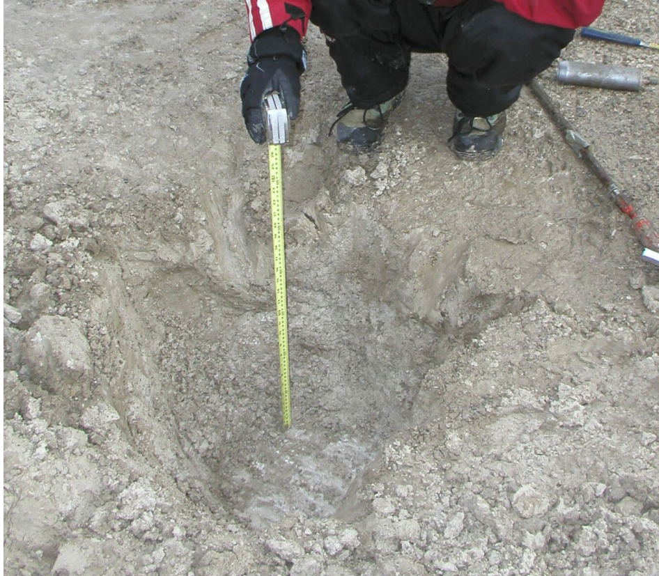
FIG. 2. Depth to the permafrost layer is approximately 60 cm in the Von Braun Valley. The soil is mainly composed of silts with the presence of some clasts. Permafrost can be observed in the bottom of the hole.
