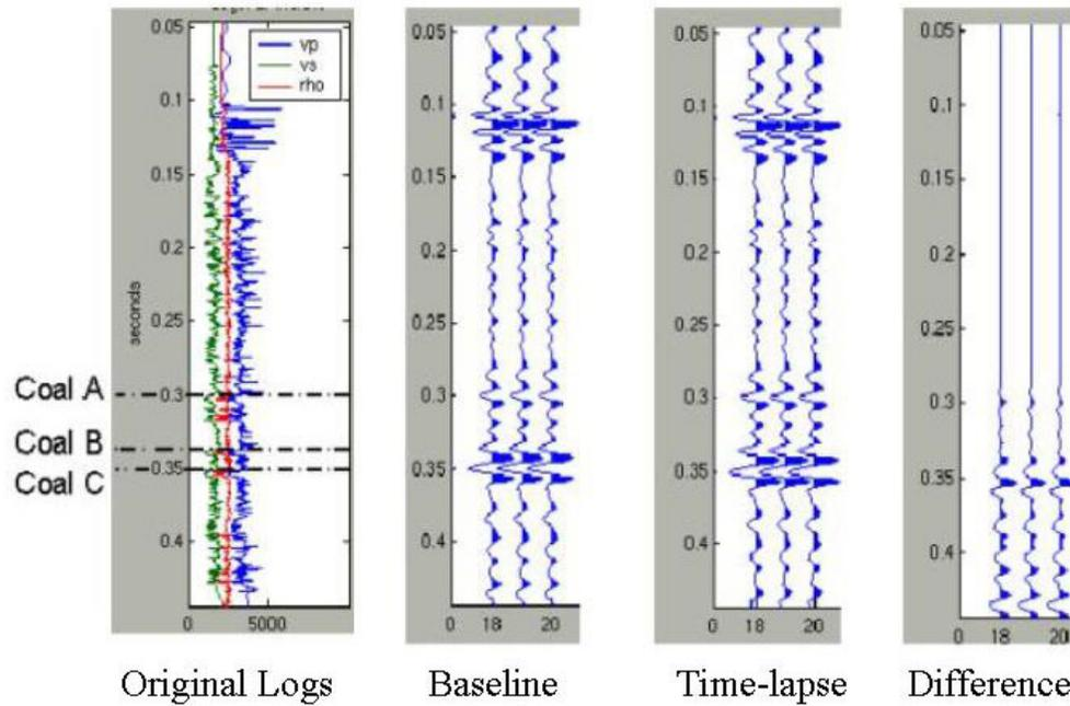
FIG. 5: Baseline, time-lapse, and difference P-P synthetic seismograms using convolution with a 60 Hz Ricker wavelet. After time-lapse, coal reflectivity is increased, and all events underlying the uppermost coal zone are delayed in time.
