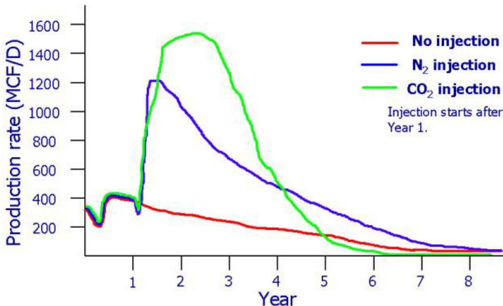
FIG. 3: Graph illustrating difference in production rate by varying injected gas. The red line represents production with no injection whereas the blue line represents injection of N<sub>2</sub>, and the green line represents the injection of CO<sub>2</sub>. Injection and production wells were arranged in a five spot pattern (Gunter et al., 1997).
