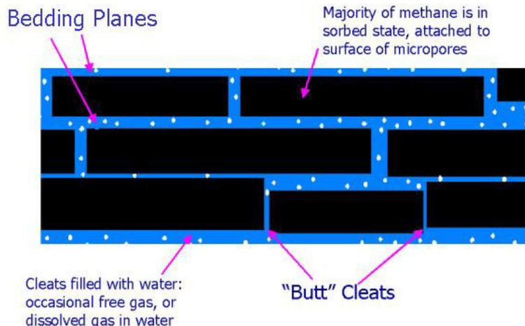
FIG. 1: Typical coal reservoir. Methane is in a sorbed state, attached to the surface of micropores within the coal, and may also be present dissolved in the water filling the cleat system. Plane of view is the face cleat.
