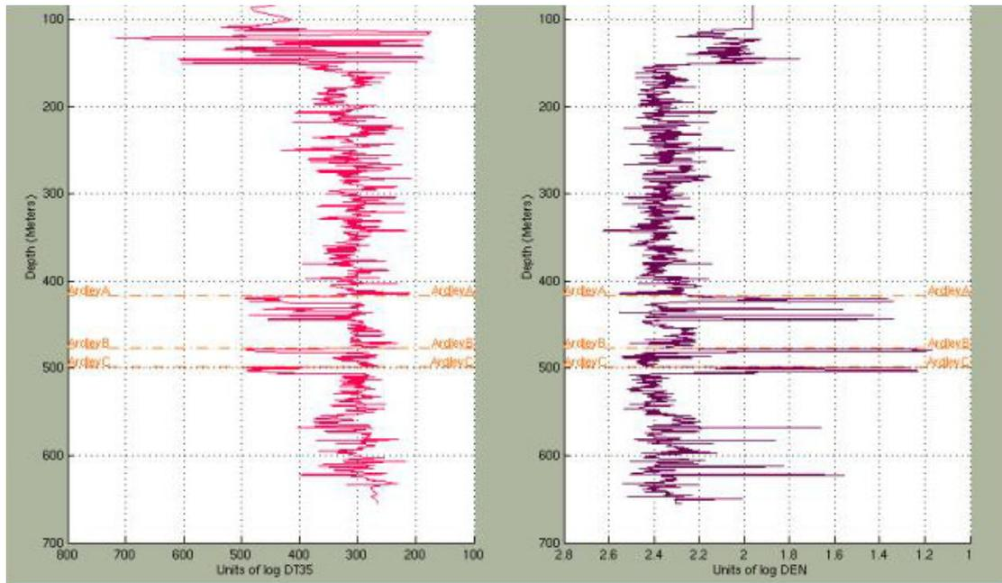
FIG. 4: Well logs of 6-22-50-11W5, indicating three zones of Ardley coal. Compressional sonic-log is on the left; density log is on the right.
