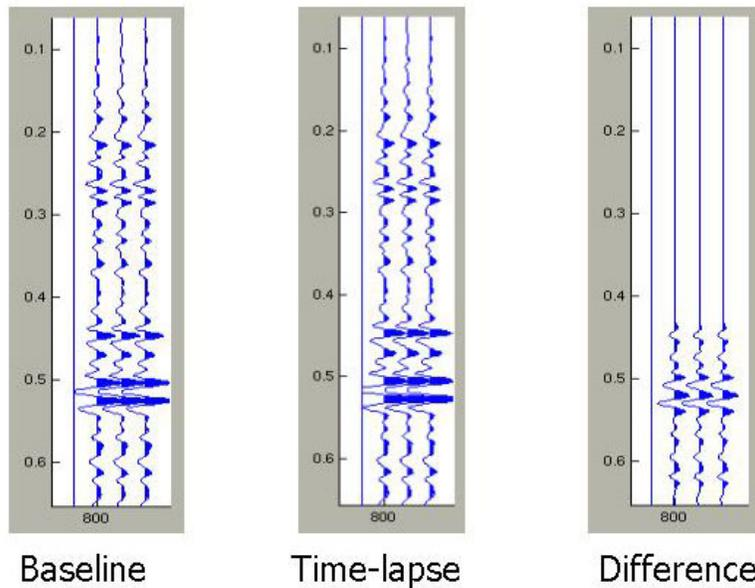
FIG. 9: Converted-wave synthetic seismograms of well 06-22. Convolution is with a 40 Hz Ricker wavelet. Once again reflectivity changes are noted within the coal seams, and push-down effects are seen in all events underlying the uppermost coal.
