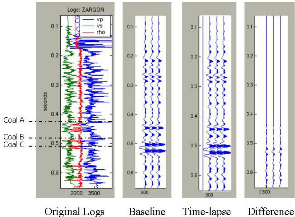
FIG. 6: Baseline, time-lapse, and difference P-S sections. Convolution is with a 40 Hz Ricker wavelet. As in the compressional-wave case, coal reflectivity is altered by the increase in acoustic impedance that accompanies a change in acoustic impedance. Velocity push-down is noted in all events underlying coal.
