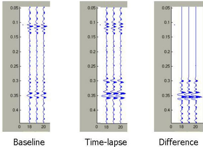
FIG. 8: P-P synthetic seismograms of well 06-22. Convolution is with a 60 Hz Ricker wavelet. A substantial increase in coal reflectivity is noted on the time-lapse section, and velocity push-down effects are noted on the difference plot.
