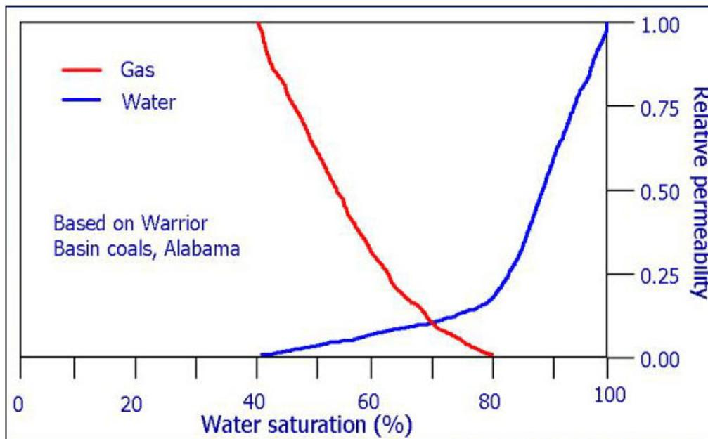
FIG. 2: Graph of relative permeability of gas and water vs. water saturation within coal seams of the Warrior Basin, Alabama. As water saturation decreases, gas production improves as the relative permeability to gas improves substantially (Alberta Geological Survey, 1990).
