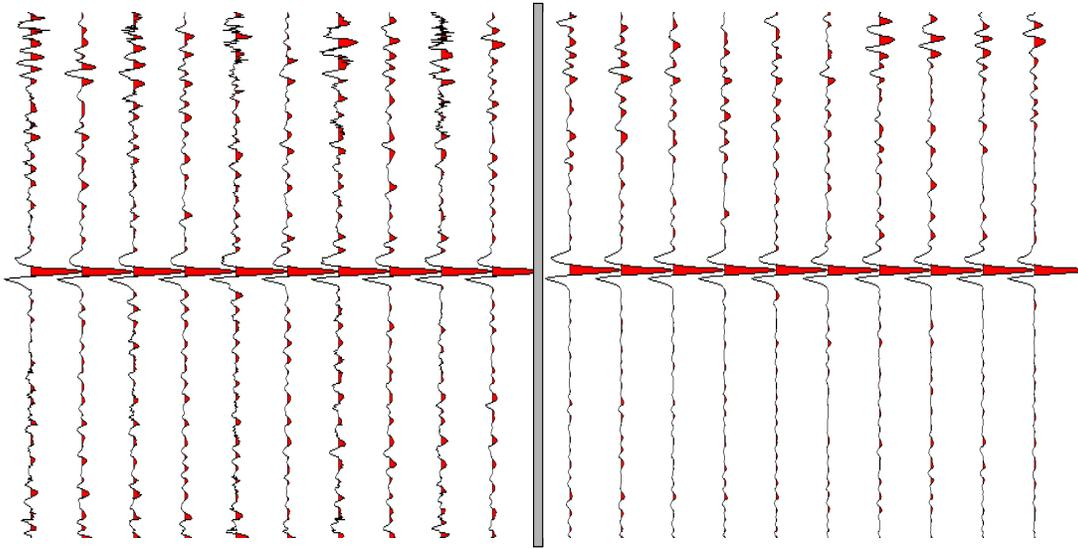
FIG. 8: The ten left-most traces are migrated CSP gathers without matched filtering. The remaining 10 traces are migrated CSP gathers located at the same positions, but have been match-filtered by a signal RC surface produced from the earth parameters found in Figure
