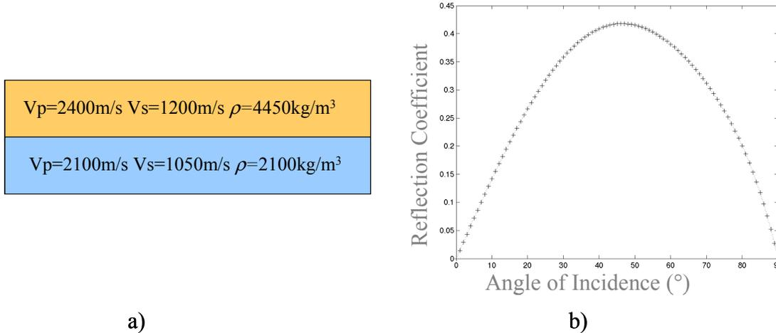
FIG. 5: a) P-S synthetic model parameters. Depth of interface is 400m; b) Zoeppritz-defined reflection coefficient curve given the earth parameters of shown in a)
