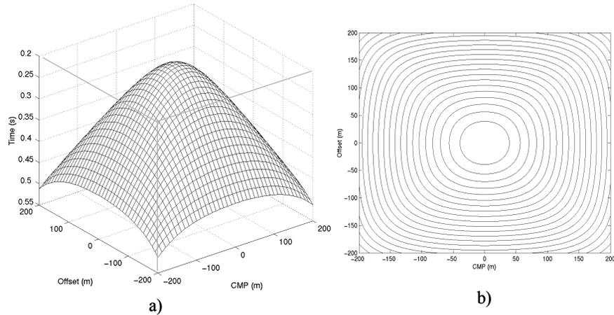
FIG. 1: a) Perspective view of a P-P wave traveltimes surface for a scatterpoint located at  $z_0=100m$ .  $V_P=800m/s$ . b) plan view of (a) showing contour lines of constant traveltimes.
