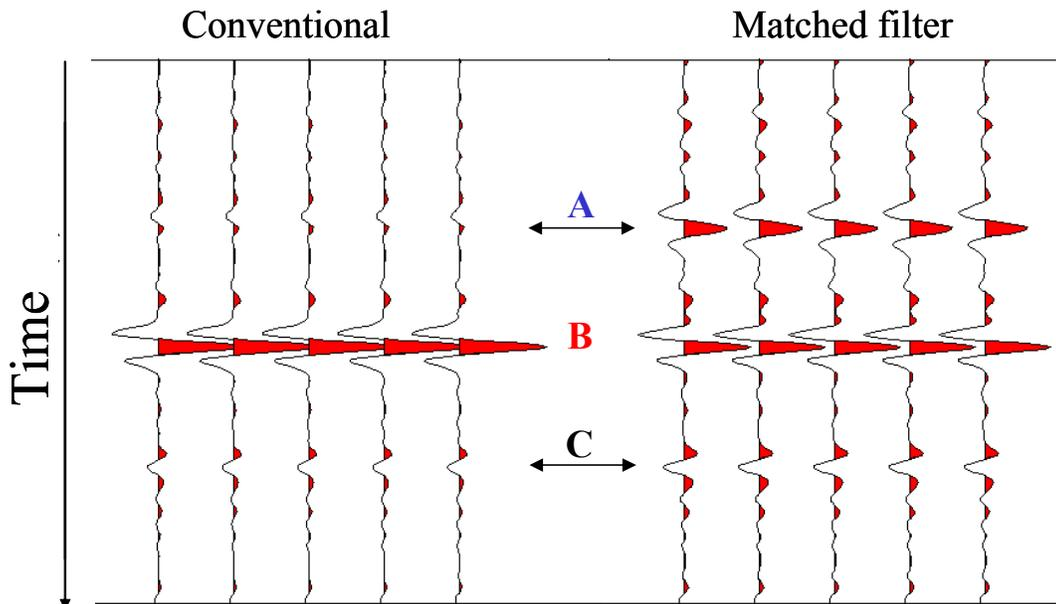
FIG. 10: Output traces from conventional prestack migration (left) compared with output-migrated traces where the amplitudes have been match-filtered to the reflection coefficients defined by the first interface.
