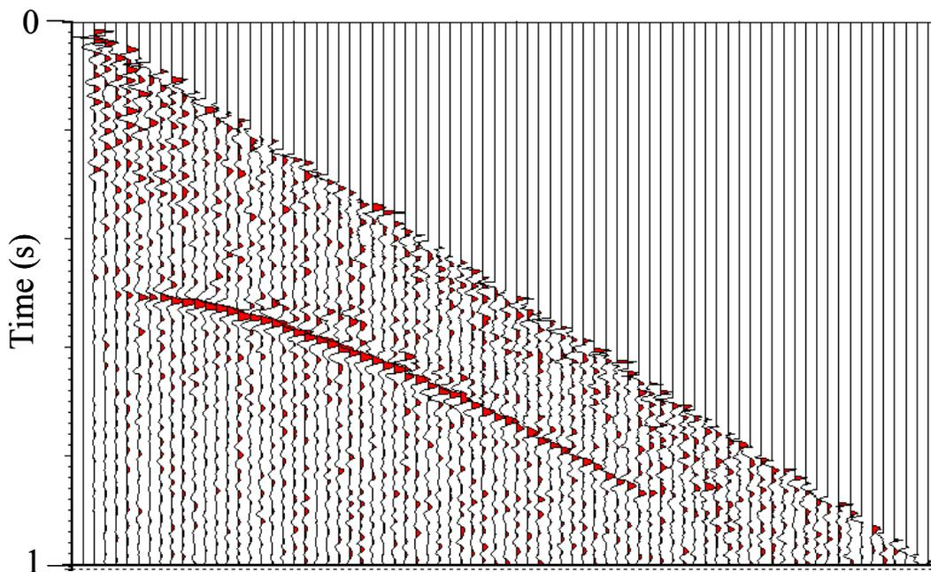
FIG. 7: CSP gather located at  $x=1250\text{m}$ . Amplitudes scaled by match-filtering. Equivalent offset shown on x-axis, where  $dx=12.5\text{m}$ .
