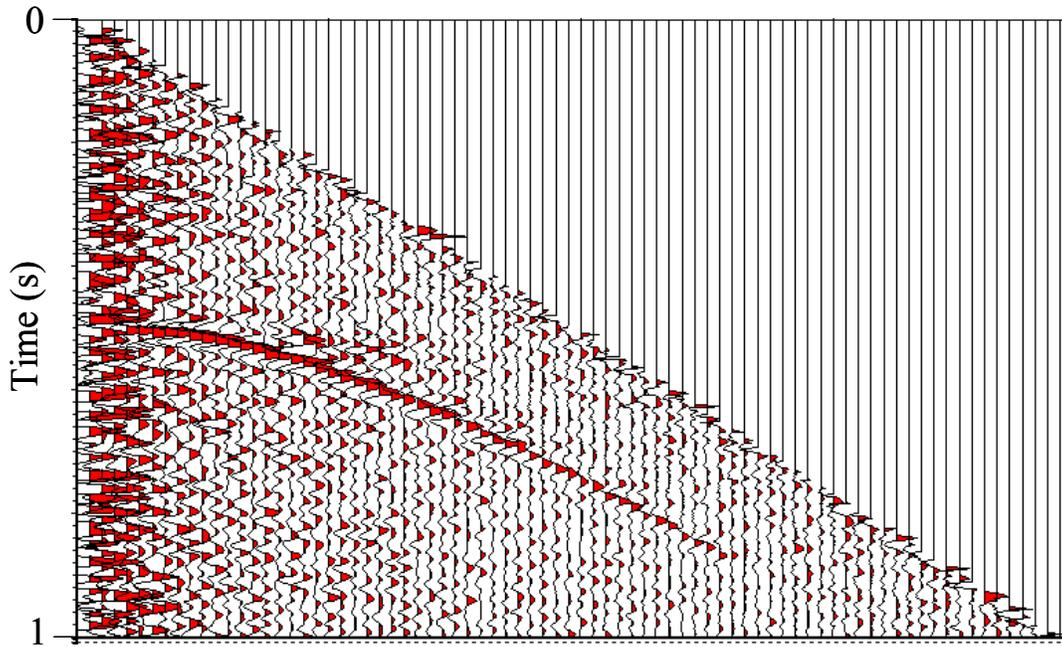
FIG. 6: Conventional CSP gather located at  $x=1250\text{m}$ . Equivalent offset shown on x-axis, where  $dx=12.5\text{m}$ .
