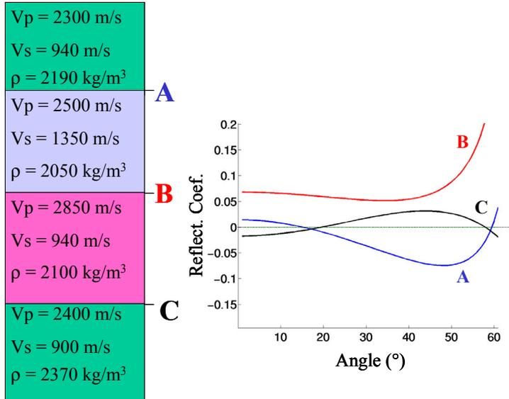
FIG. 9: Earth model for P-wave synthetic on the left. Interfaces A and C represent low impedance contrast, Class II AVO anomalies. Interface B has a high-impedance contrast and is easily imaged. Zoepritz reflection coefficients for each interface are plotted on the right.
