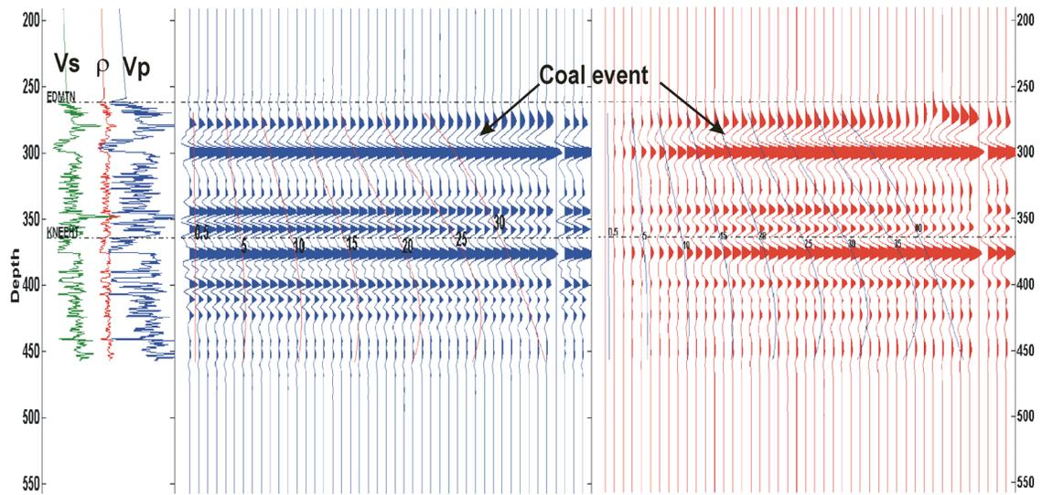
FIG. 6: Comparison of P-P and P-S offset synthetic seismograms displayed in depth. Left is P-P (80-Hz Ricker wavelet); right is P-S (40-Hz Ricker wavelet). Overlays show incidence angles.
