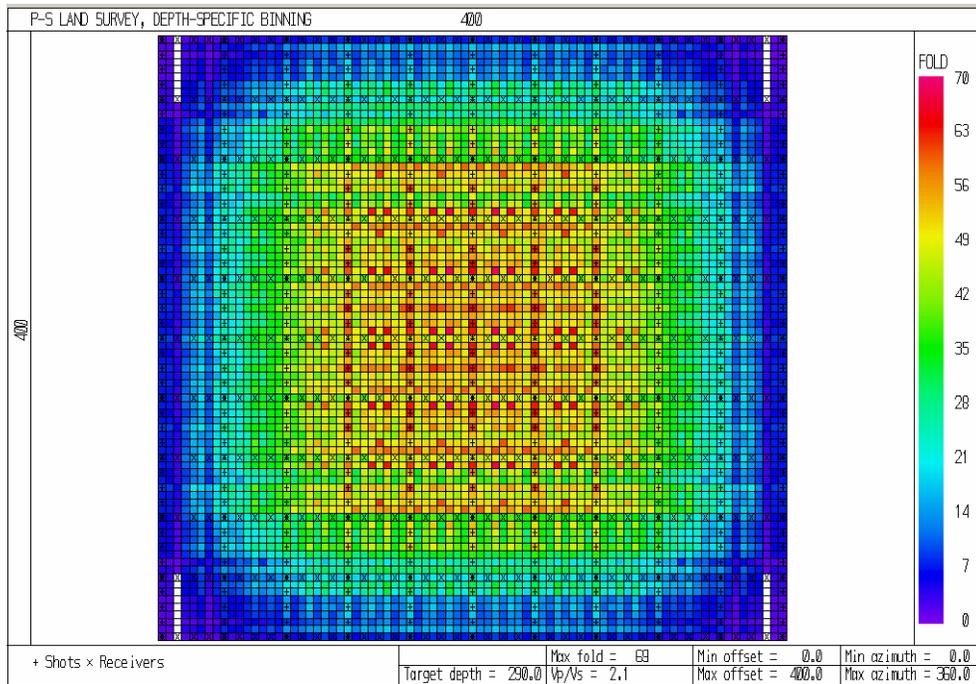
FIG. 9: Depth-specific P-S fold, coalbed methane 3C-3D seismic survey. Vp/Vs = 2.1 and depth = 290 m. Offsets up to 400 m.
