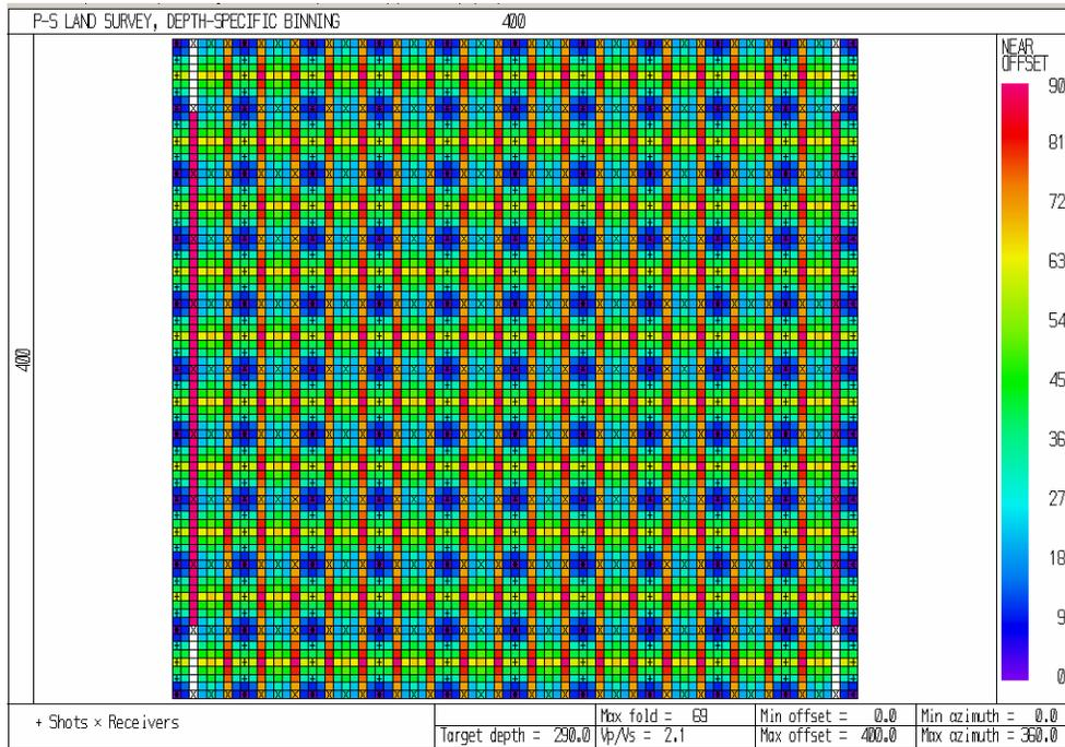
FIG. 11: P-S minimum offset distribution, coalbed methane 3C-3D seismic survey.
