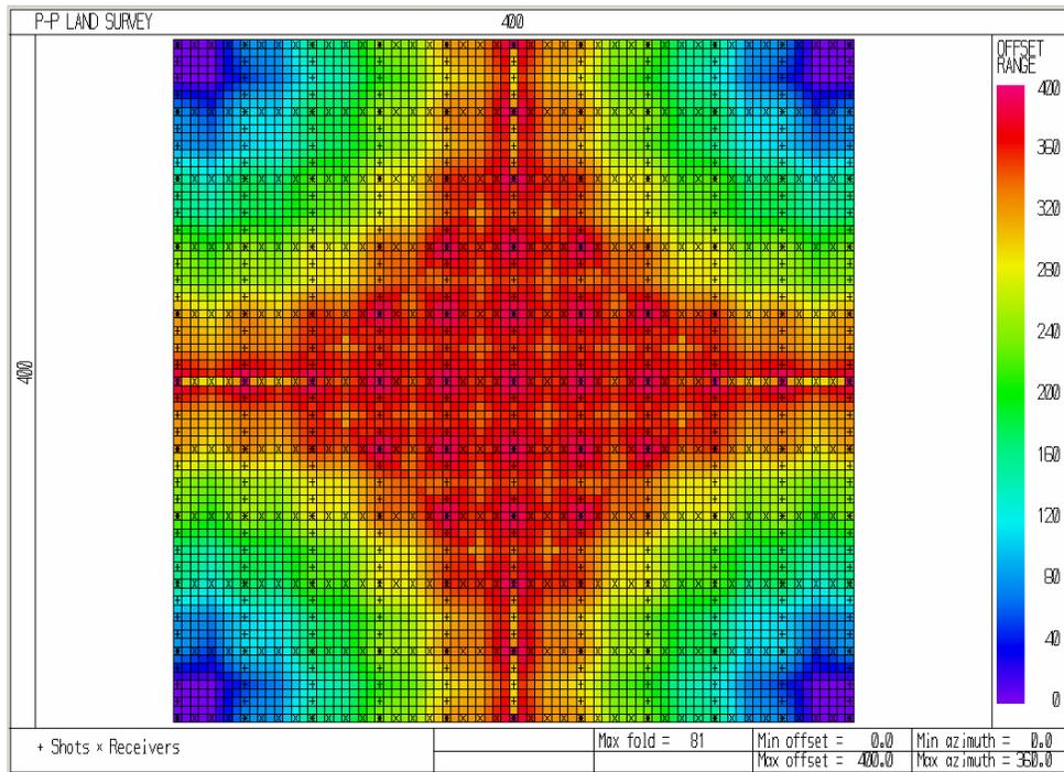
FIG. 12: P-P maximum offset distribution, coalbed methane 3C-3D seismic survey.
