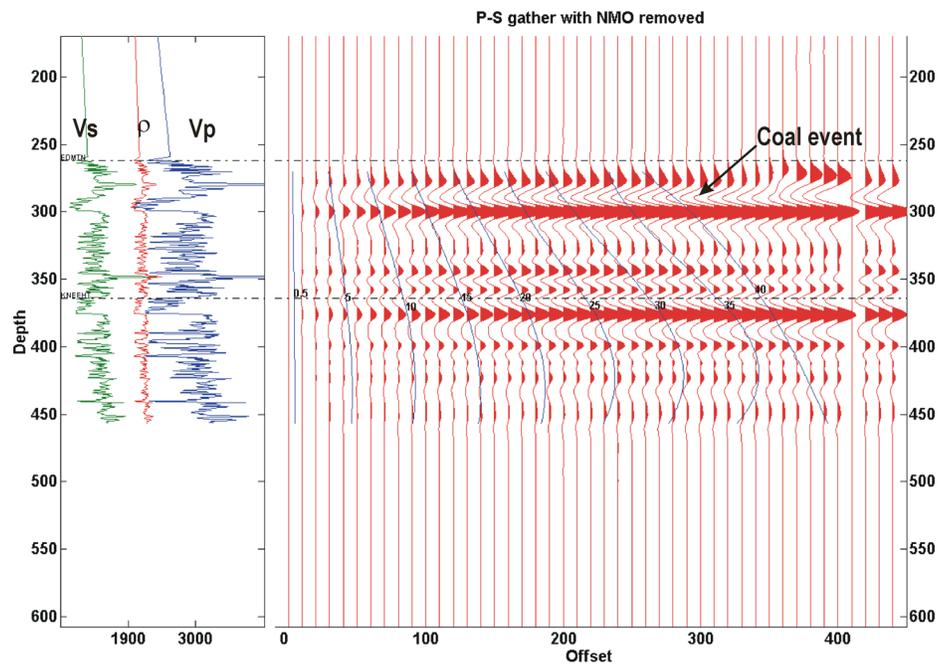
FIG. 5: P-S offset synthetic seismogram (depth) based on the 10-34-38-28W4 sonic log. Offsets 0 to 400 m; 40 Hz Ricker wavelet. Last 3 traces are stacked from the gather. Overlay shows incidence angles.
