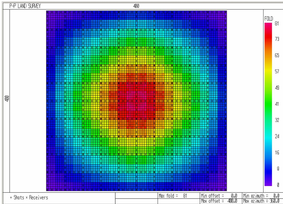
FIG. 8: P-P fold, coalbed methane 3C-3D seismic survey. Offsets up to 400 m.
