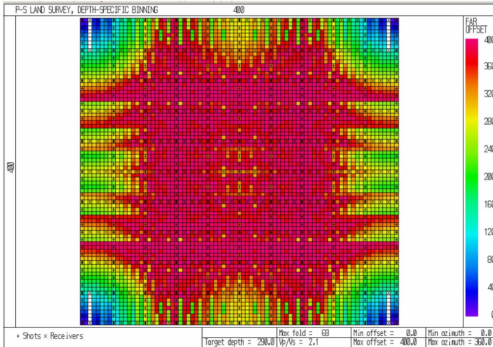
FIG. 13: P-S maximum offset distribution, coalbed methane 3C-3D seismic survey.
