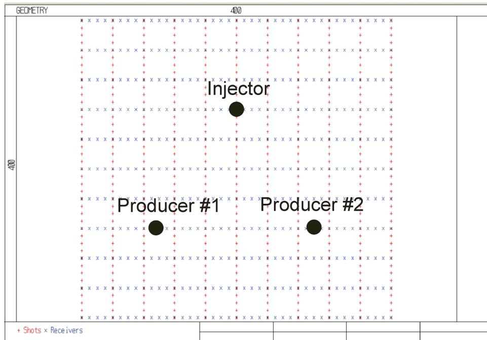
FIG. 7: Surface source and receiver geometry for planned 3C-3D surface seismic survey to monitor enhanced coalbed methane production, stimulated with CO<sub>2</sub> injection.
