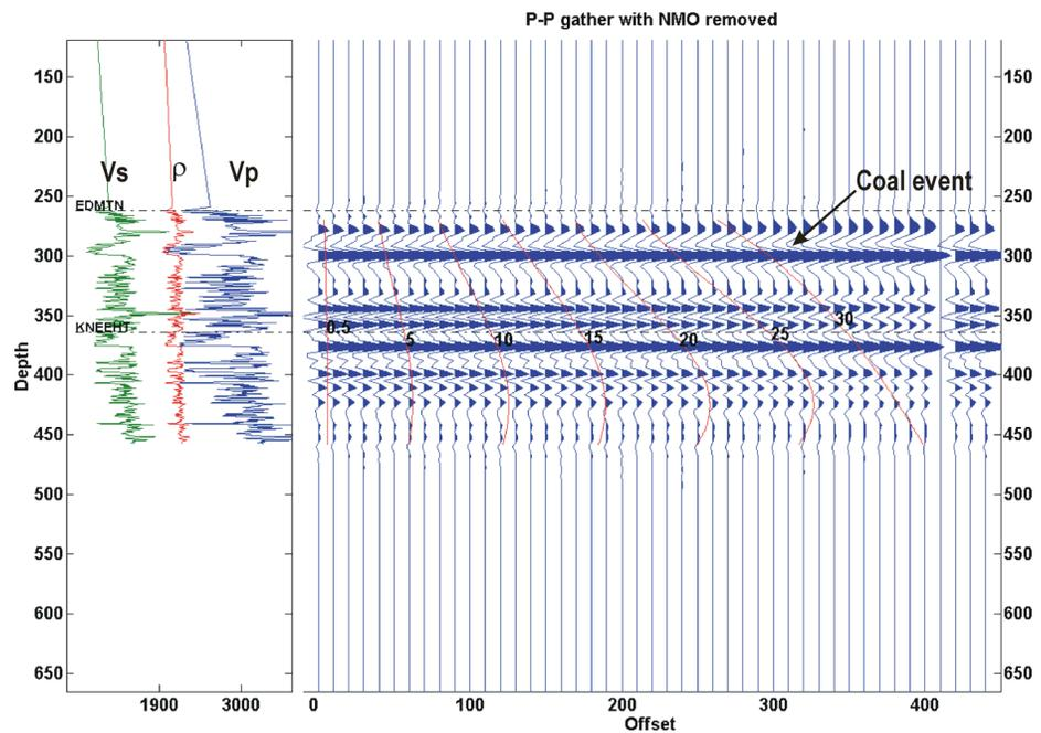
FIG. 3: P-P offset synthetic seismogram (depth) based on the 10-34-38-28W4 sonic log. Offsets 0 to 400 m; 80-Hz Ricker wavelet. Last 3 traces are stacked from the gather. Overlay shows incidence angles.
