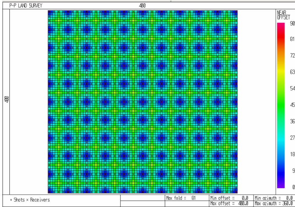
FIG. 10. P-P minimum offset distribution, coalbed methane 3C-3D seismic survey.
