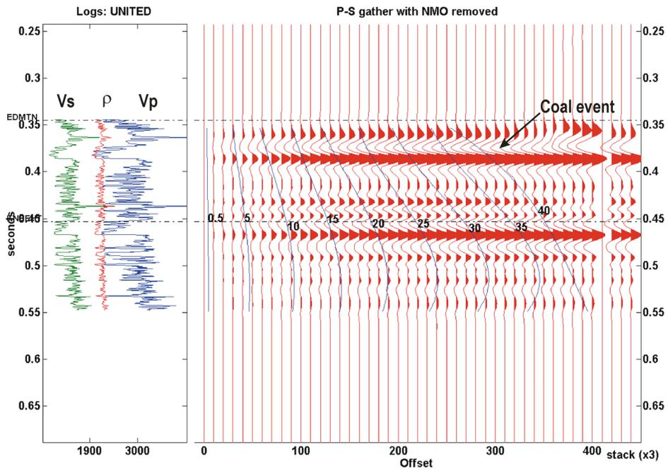
FIG. 4: P-S offset synthetic seismogram (time) based on the 10-34-38-28W4 sonic log. Offsets 0 to 400 m; 40-Hz Ricker wavelet. Last 3 traces are stacked from the gather. Overlay shows incidence angles.
