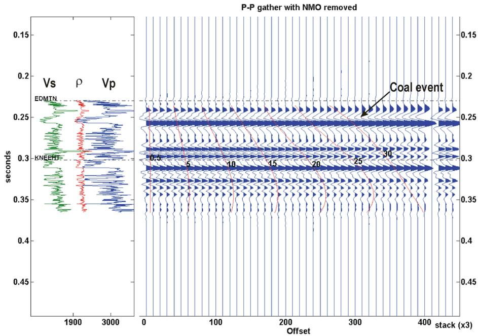
FIG. 2: P-P offset synthetic seismogram (time) based on the 10-34-38-28W4 sonic log. Offsets 0 to 400 m; 80 Hz Ricker wavelet. Last 3 traces are stacked from the gather. Overlay shows incidence angles.
