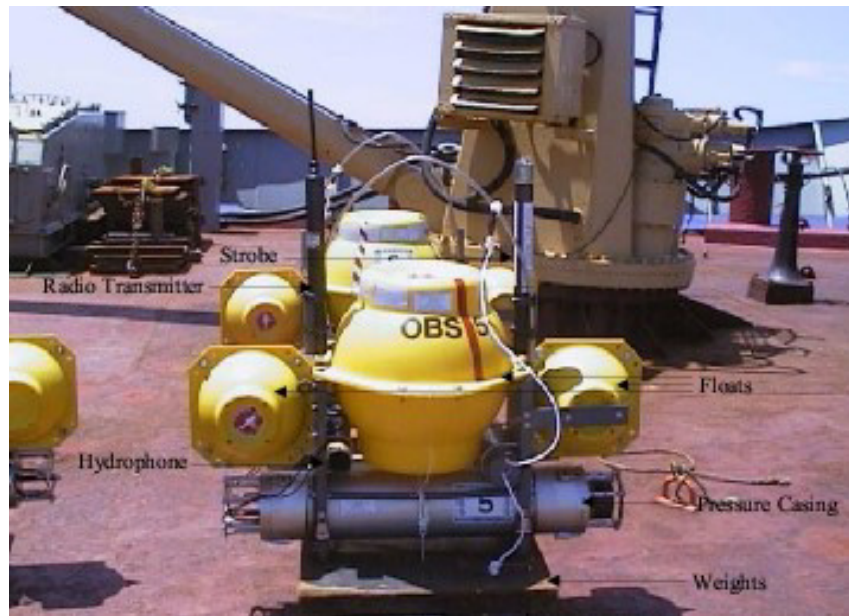
FIG. 1. Dalhousie ocean bottom seismometer (OBS). Picture taken from Dalhousie Seismic Group website ( www.phys.ocean.dal.ca/seismic/ )
