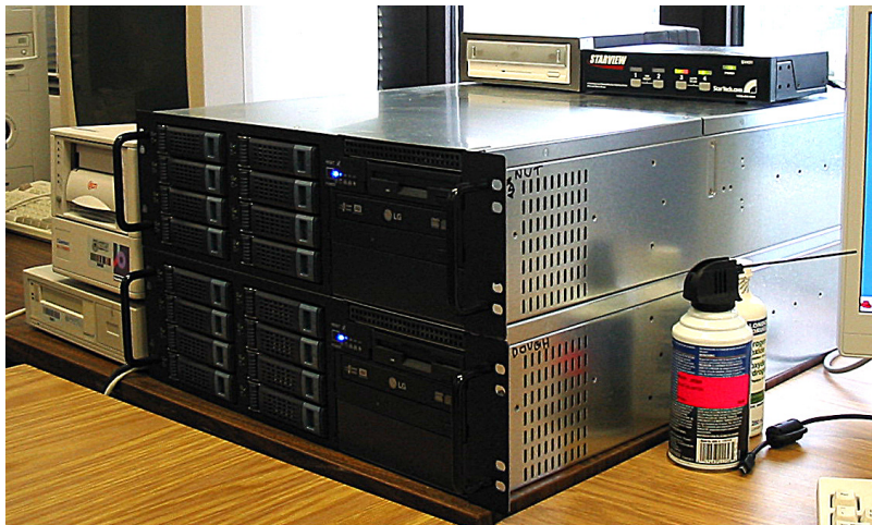
FIG. 1. Two new Linux servers with two 600 GB partitions each provide a total of 2.4 TB of data storage space.
