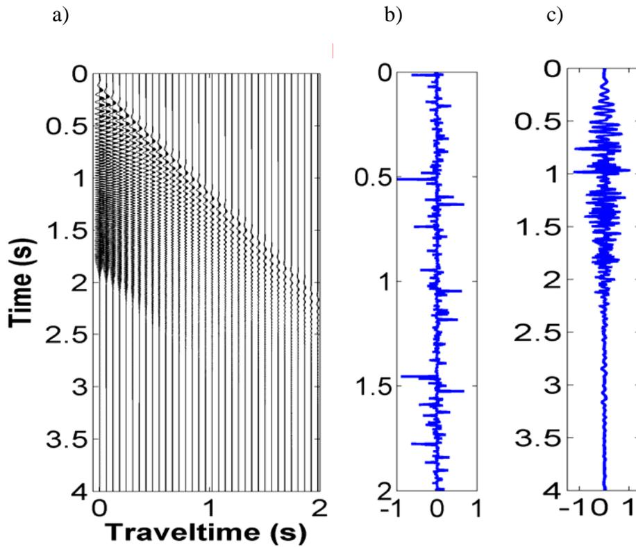
FIG. 5. a) The attenuated sweep, b) reflectivity, and c) uncorrelated trace.
