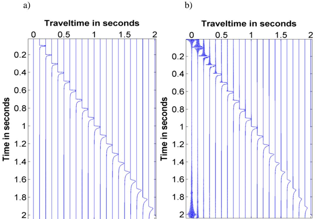
FIG. 7. a) Impulse response of the forward Q filter, and b) the wavelet estimates on the sweep-removed trace.
