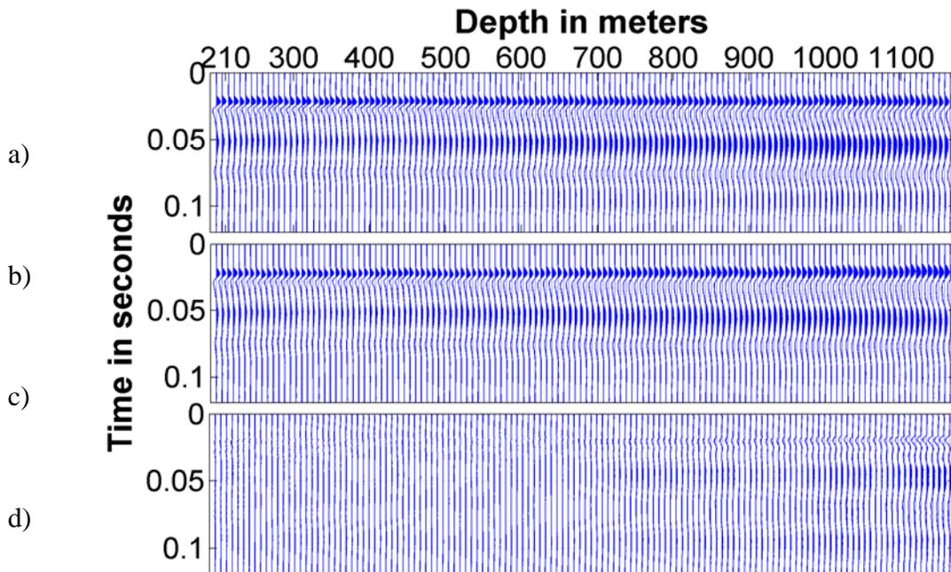
FIG. 3. a) Directly observed wavelets in VSP downgoing waves from Ross Lake (normalized to peak amplitude); b) the minimum-phase equivalents of the wavelets shown in a); and c) the difference between a) and b).
