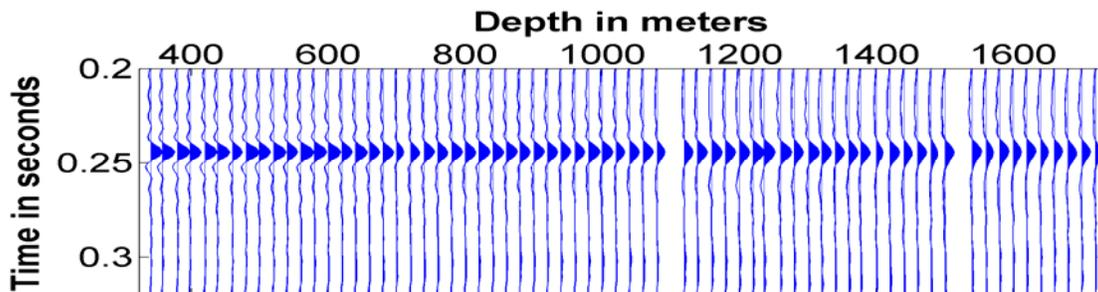
FIG. 1. a) Directly observed wavelets (normalized to peak amplitude), and b) the result of minimum-phase spiking deconvolution on the wavelets of a).
