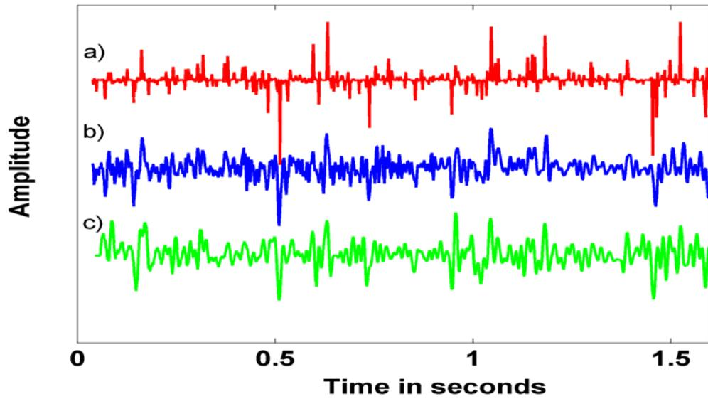
FIG. 8. a) The reflectivity, b) the trace after the Gabor deconvolution on the sweep-removed data, and c) the trace after the Gabor deconvolution on the correlated data.
