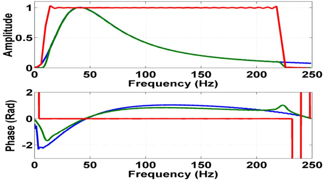
FIG. 4. Spectra of the Klauder wavelet (red), minimum-phase wavelet (blue), and effective minimum-phase wavelet (green).
