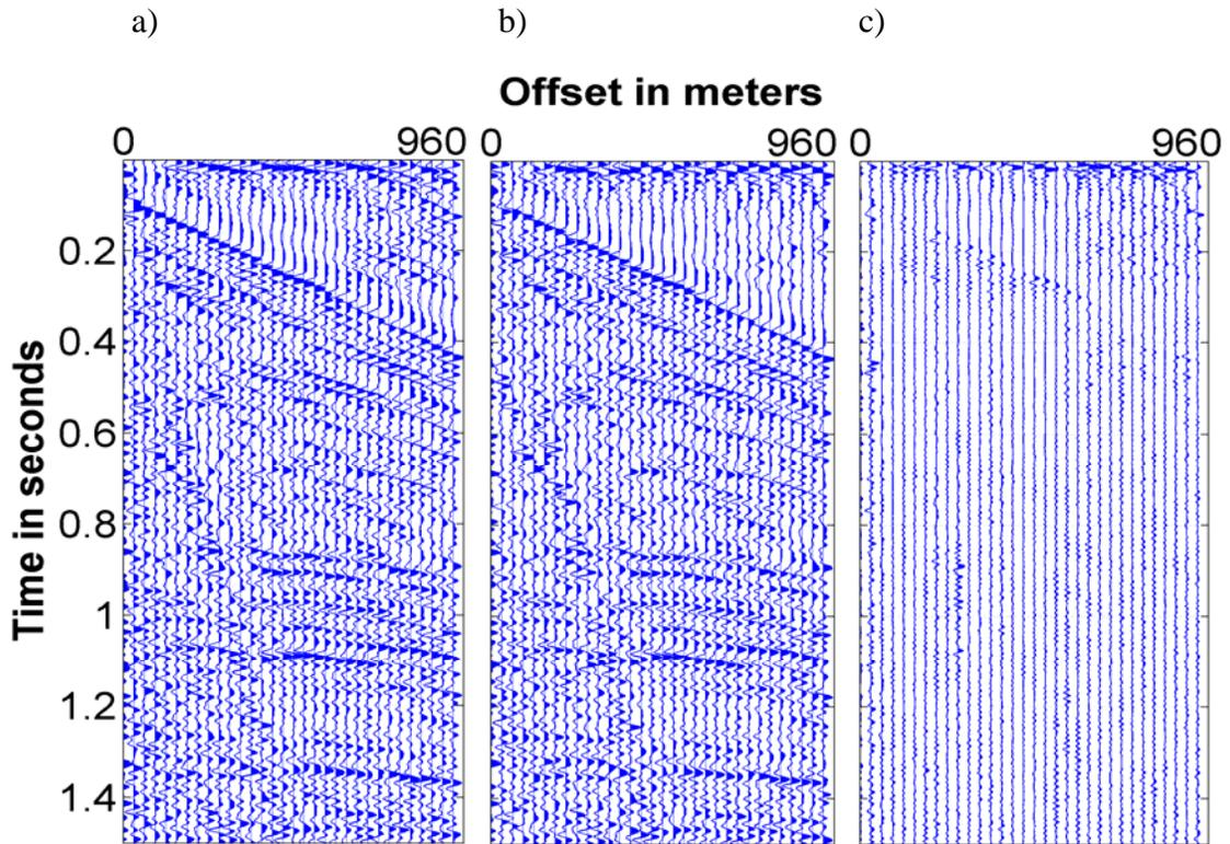
FIG. 9. a) The gather after minimum-phase Gabor deconvolution of the correlated data; b) the gather after minimum-phase Gabor deconvolution of the uncorrelated data; and c) the differences of the data shown in a) and b).
