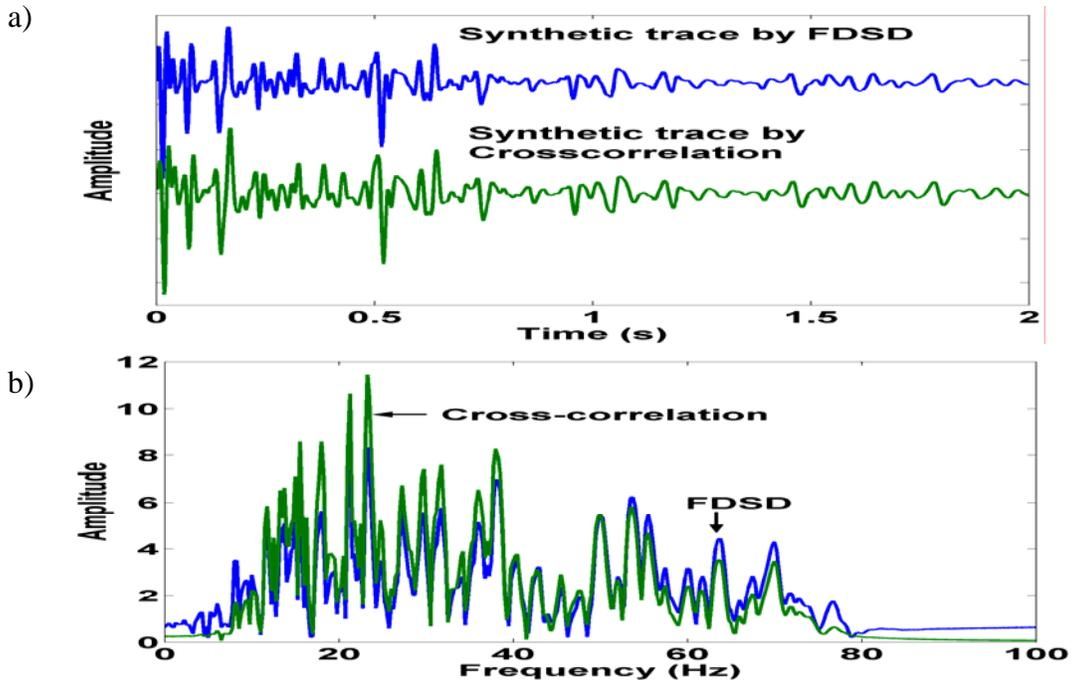
FIG. 6. a) Synthetic traces by FDS and crosscorrelation, and b) amplitude spectra of the synthetic traces.
