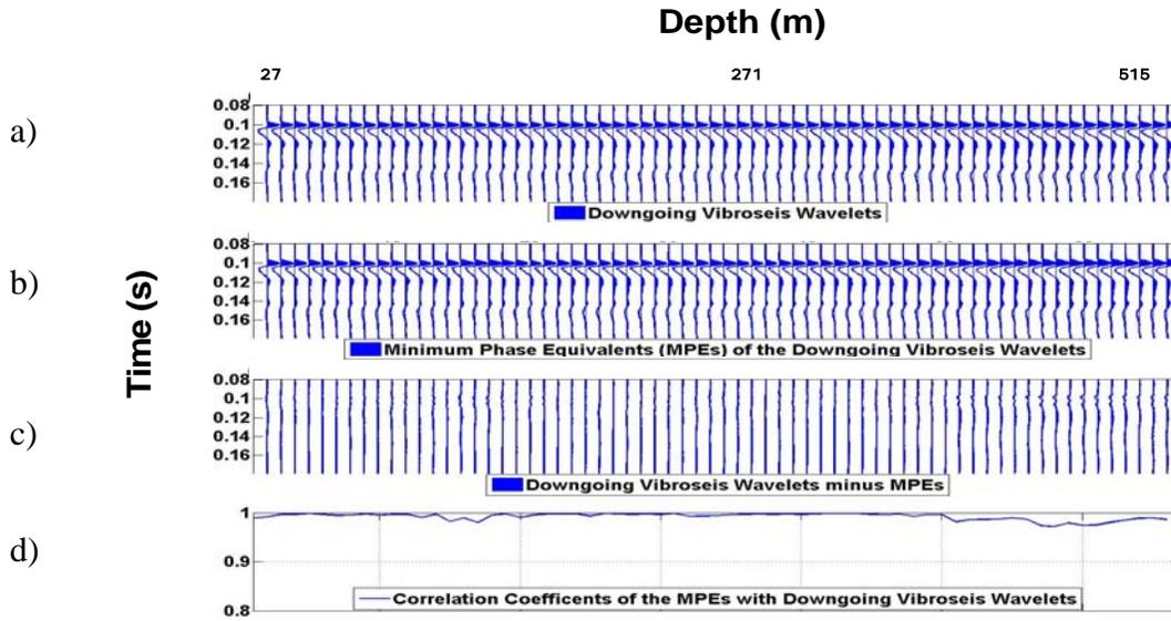
FIG. 2. a) Directly observed wavelets in VSP downgoing waves from Pikes Peak (normalized to peak amplitude); b) the minimum-phase equivalents (MPEs) of the wavelets shown in a); c) the difference between a) and b); and d) the correlation coefficients of the MPEs with downgoing Vibroseis wavelets.
