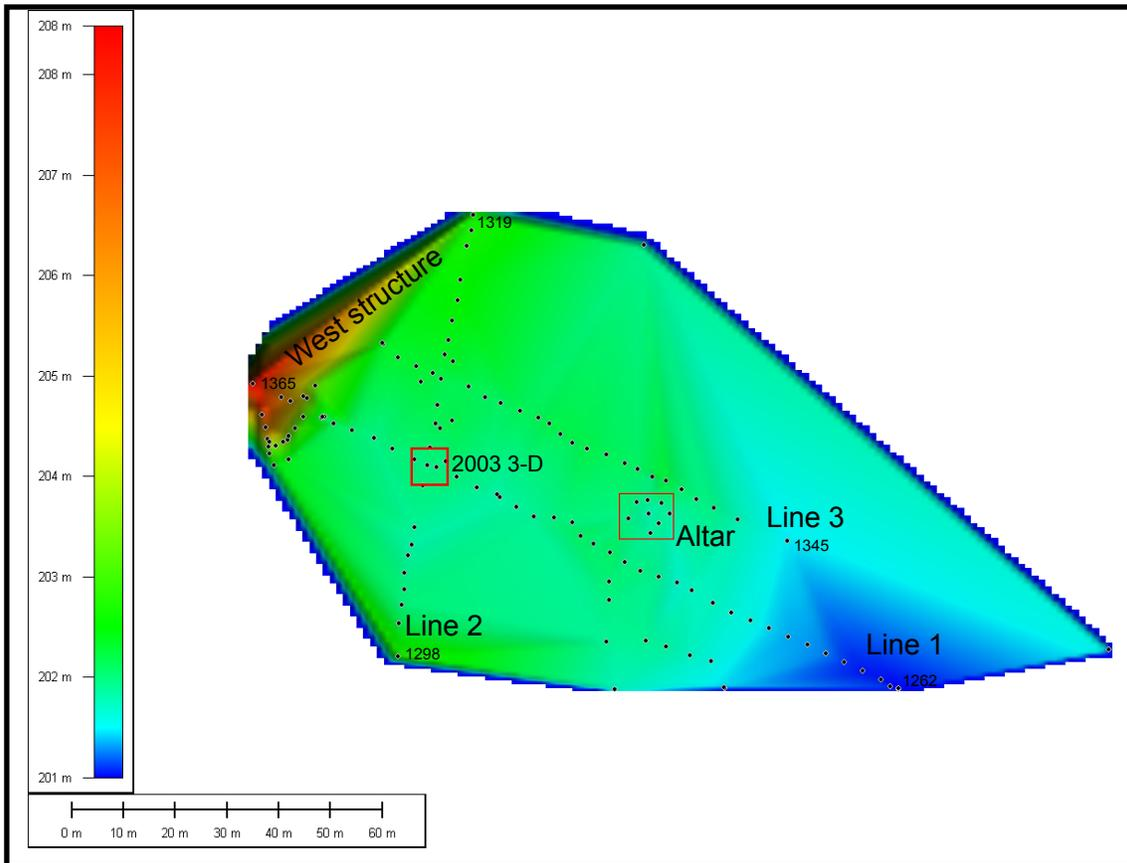
FIG. 5. Elevation and coordinate map for the plaza at Maax Na based on the Total Station survey.
