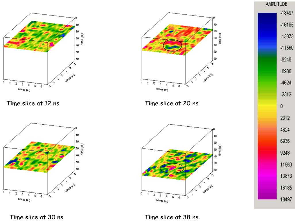
FIG. 10. Time slices from the GPR 3-D volume. Anomalies highlighted in black.
