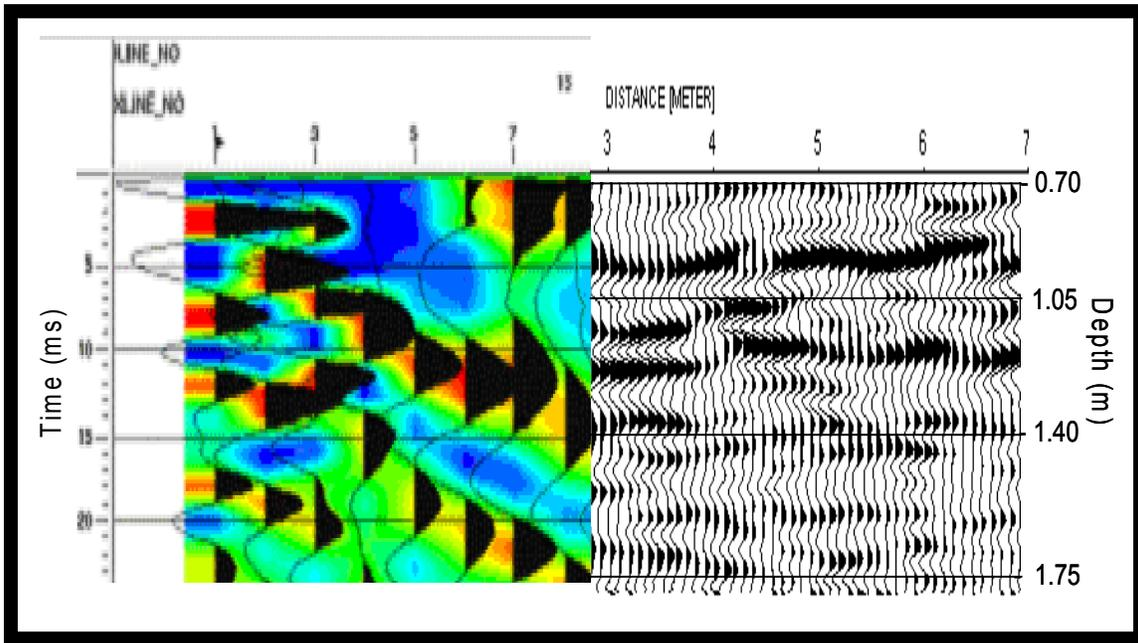
FIG. 17. Comparison of the micro-seismic (left) and GPR (right) surveys at depths 0.7 - 1.75 m.
