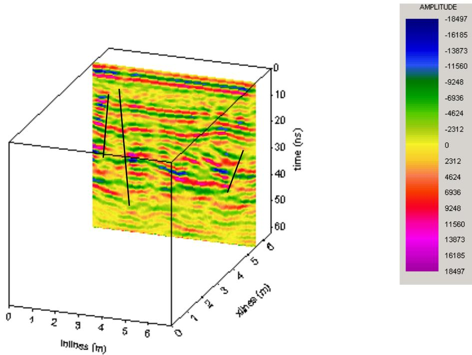
FIG. 8. Inline 3 from 2003 3-D GPR dataset with anomalies and highlighted discontinuities.
