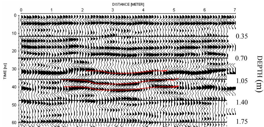
FIG. 16. Wiggle trace display of Inline 15 of the GPR survey. Note the similarity in structure between both lines.
