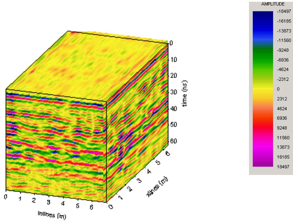
FIG. 7. 3-D cube of GPR data from the 2003 3-D shot over the excavated pit.
