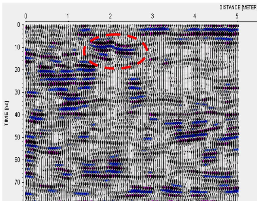
FIG. 12. Wiggle trace display of Grid 2 Line 4 showing structural anomaly in vicinity of “altar”.
