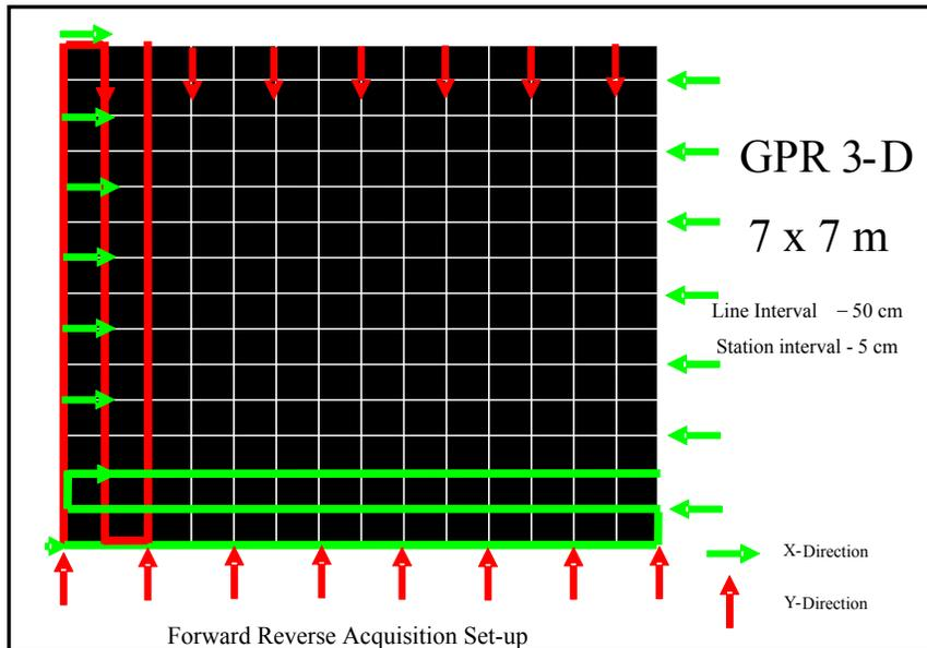
FIG. 4. Layout of 3-D grid with lines acquired in forward and reverse directions both in E-W and N-S orientations.
