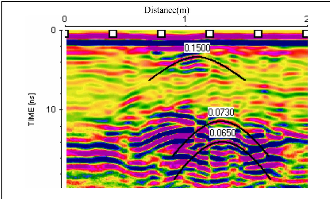
FIG. 3. Velocity determination using interactive curve fitting in the field and using Reflexw.
