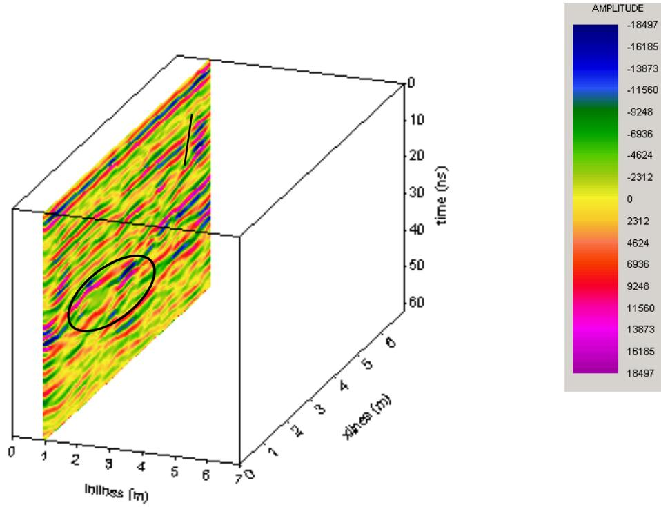
FIG. 9. Xline 3 from 3-D grid showing discontinuities and amplitude anomalies.
