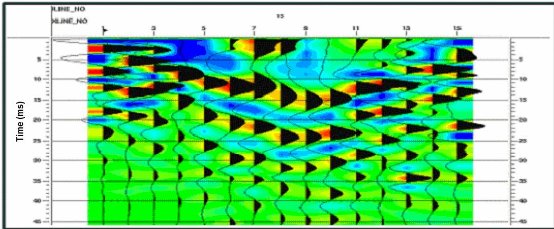
FIG. 15. Inline 15 stacked data, displaying variable density with trace overlay from 3C-3D micro-seismic survey.
