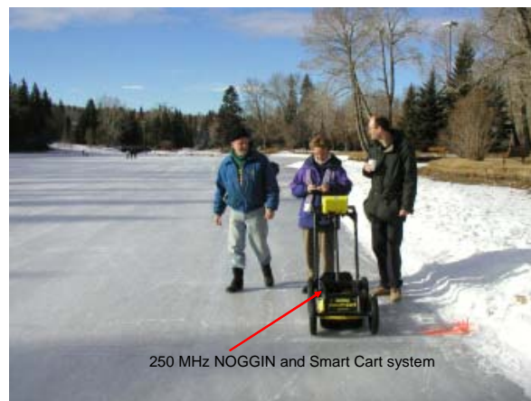
FIG. 1. Dr. Larry Bentley and Ms. Julie Aitken of the University of Calgary and Mr. Greg Johnson of Sensors and Software Inc. conduct a GPR survey, with the Noggin 250-MHz SmartCart®, over the frozen lagoon at Bowness Park, Calgary.
