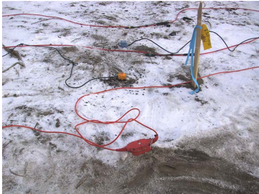
FIG. 5. Three of the geophones planted at station 5184. Order from bottom to top is Sercel DSU3, IO-Spike and GS-3C (IO-Nail is missing from this view).
