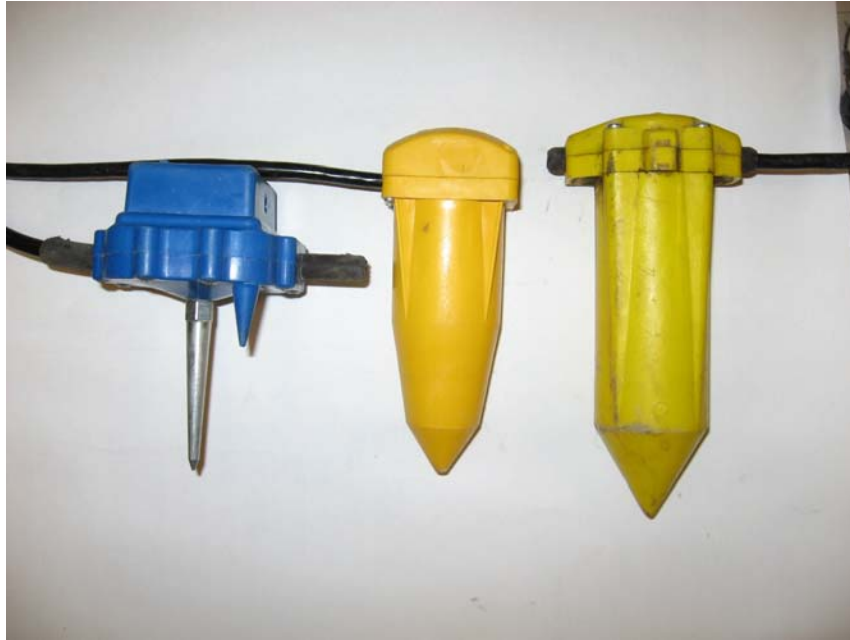
FIG. 4. Coil geophones used in the experiment. GS-3C (left); IO-Spike (centre) and OG-Nail (right).
