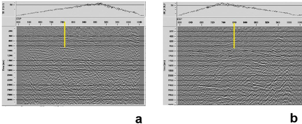
FIG. 14. Processing dip line converted wave, L-99 survey. (a) Positive offset. (b) Negative offset.
