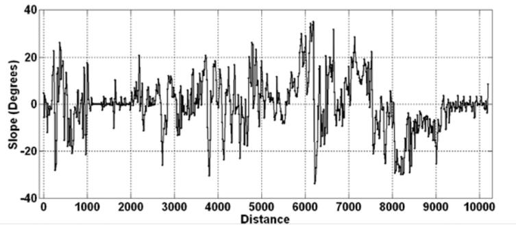
FIG. 6. Slope in degrees along the line, calculated for each receiver.
