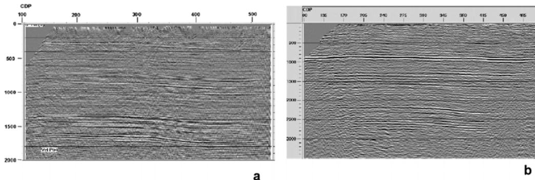
FIG. 13. Strike line of L-99. (a) P-wave stack, (b) PS-wave stack.
