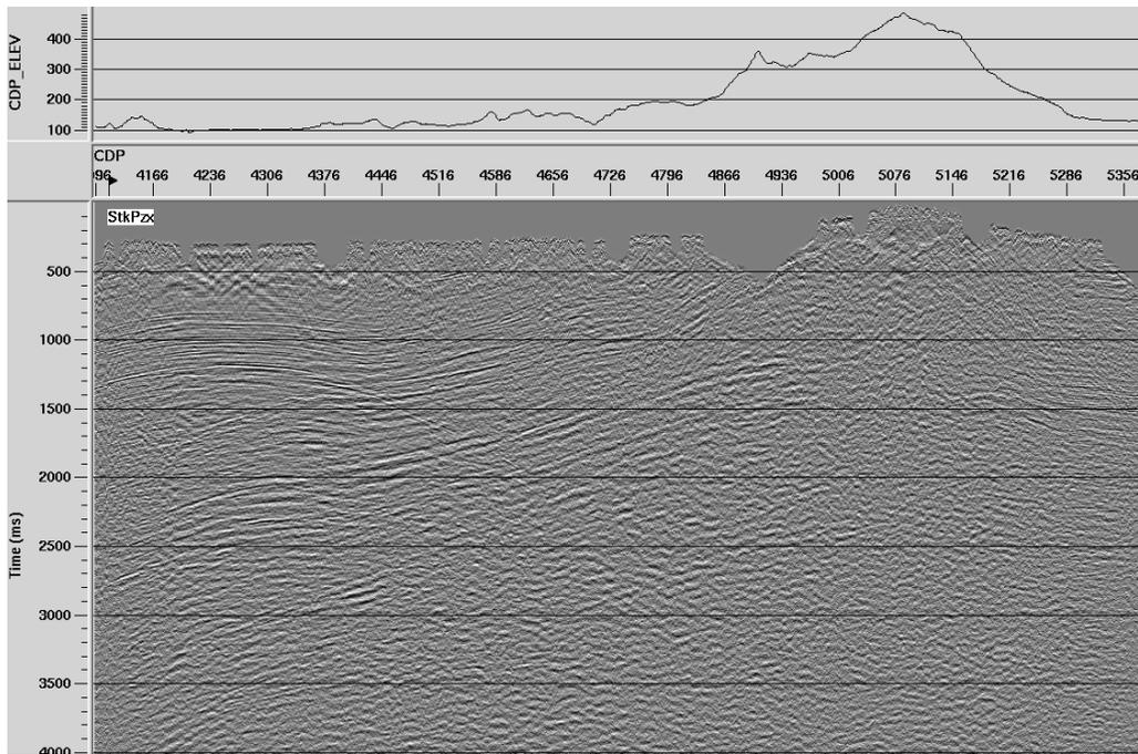
FIG. 9. Stacked section after mode-wave separation taking into account the topography.
