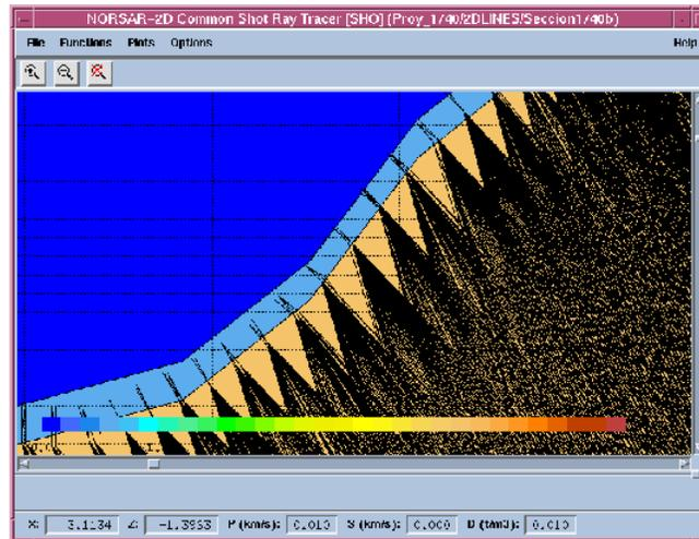
FIG. 4. Ray tracing with a low velocity layer and topography.
