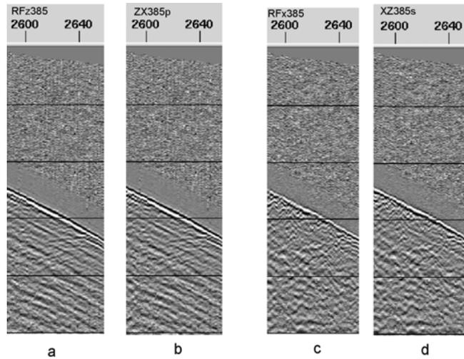
FIG. 8. Comparison of the two components before (left) and after (right) rotation. A) and b), vertical, (c) and (d) horizontal.
