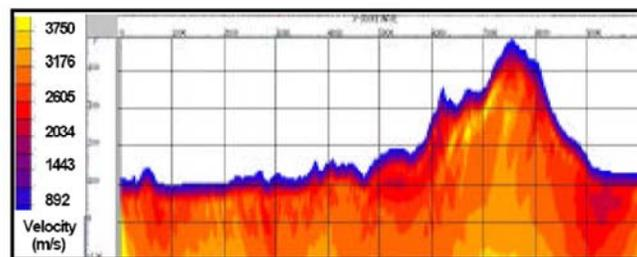
FIG. 11. Near surface velocity model from tomography (From Acevedo et al., 2006).
