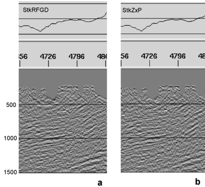
FIG. 10. Close-up of stacked sections (a) before wave mode separation and (b) after wave mode separation. Subtle differences can be observed.
