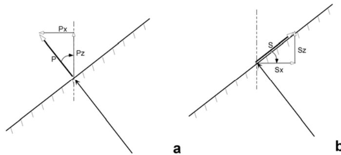
FIG. 5. Arrival direction and multicomponent detection in a steep slope area. a) Components of the P-wave. b) Components of the S-wave.
