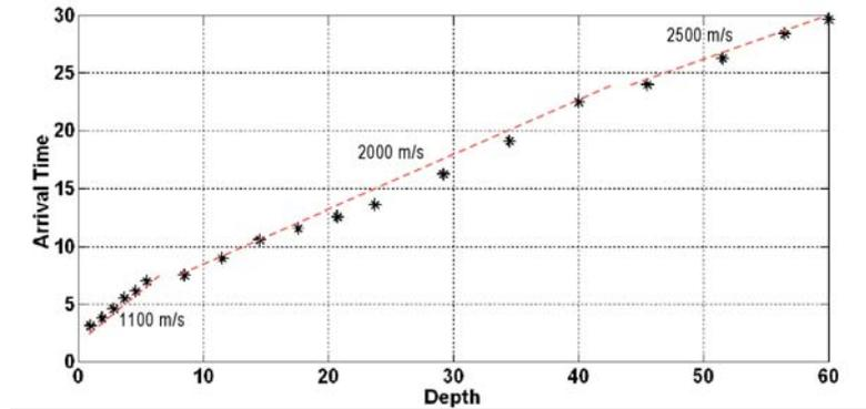
FIG. 12. Arrival times for the Uphole. Notice high velocities close to the surface.
