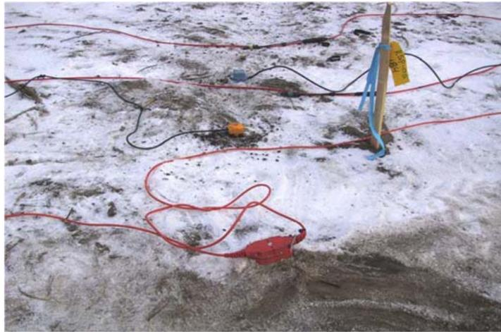
FIG. 2. From the top: OYO 3C (blue), ION Spike (orange) and DSU3 (red) (Lawton et al., 2005).
