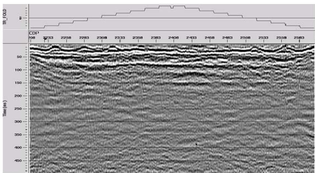
Priddis pulse probe—Dynamite + 20 Hz—CDP stack, 2000 m/s LM 0, reverse polarity
