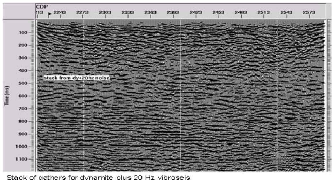
Stack of gathers for dynamite plus 20 Hz vibroseis
