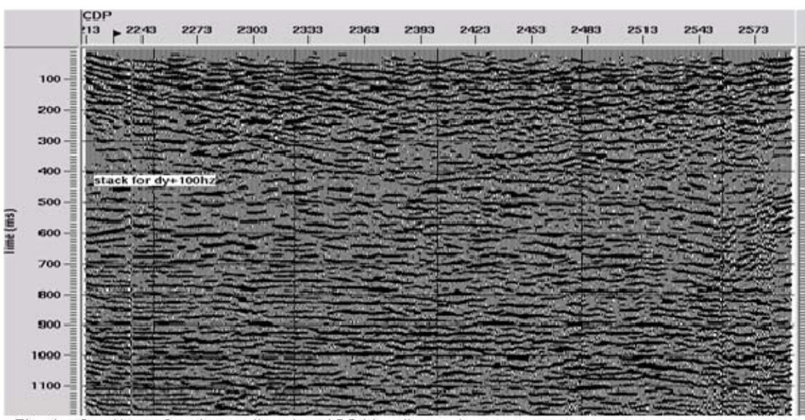
Stack of gathers for dynamite plus 100 Hz vibroseis
