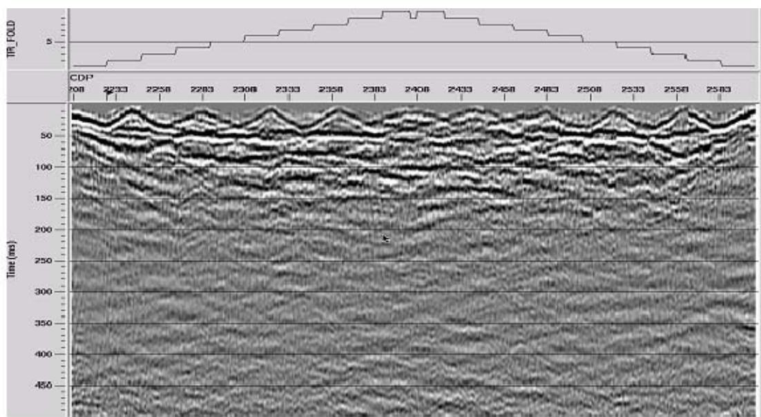
Priddis pulse probe—Dynamite + 20 Hz—CDP stack, 2000 m/s NMO, reverse polarity
