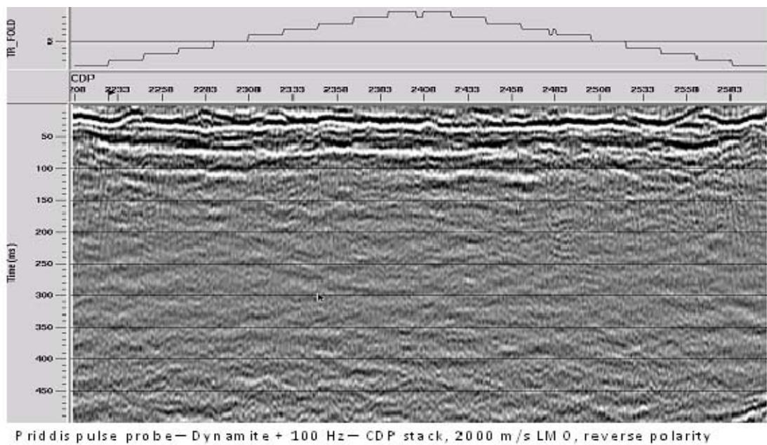
FIG. 53. CDP stack of 100 Hz pump-probe survey with 2000 m/s LMO applied to shot gathers.
