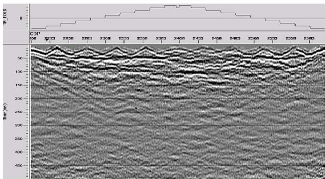
FIG. 47. CDP stack of 50 Hz pump-probe survey with 2000 m/s NMO applied to shot gathers.
