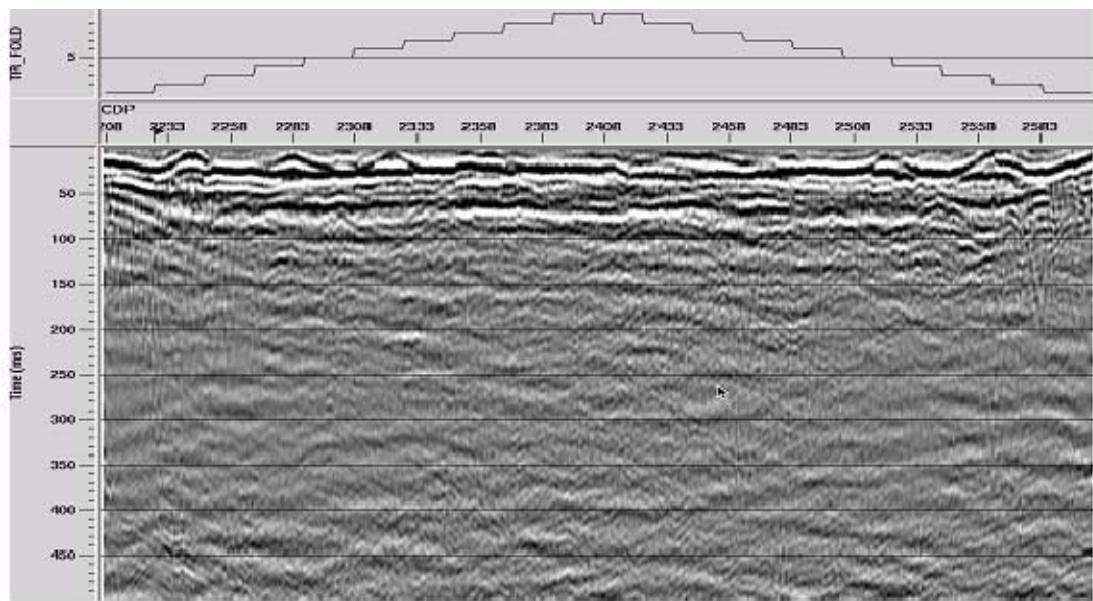
CDP stack of vertical component—dynamite only—2000 m/s LMO
