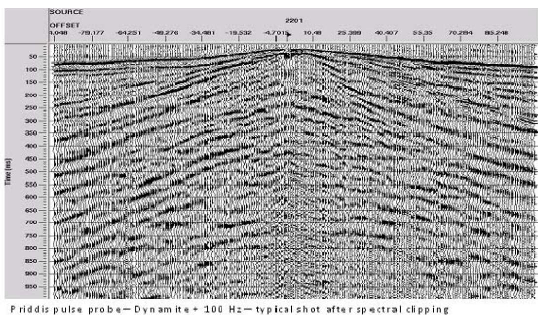
FIG. 42. Shot gather from Figure 41 after spectral clipping.
