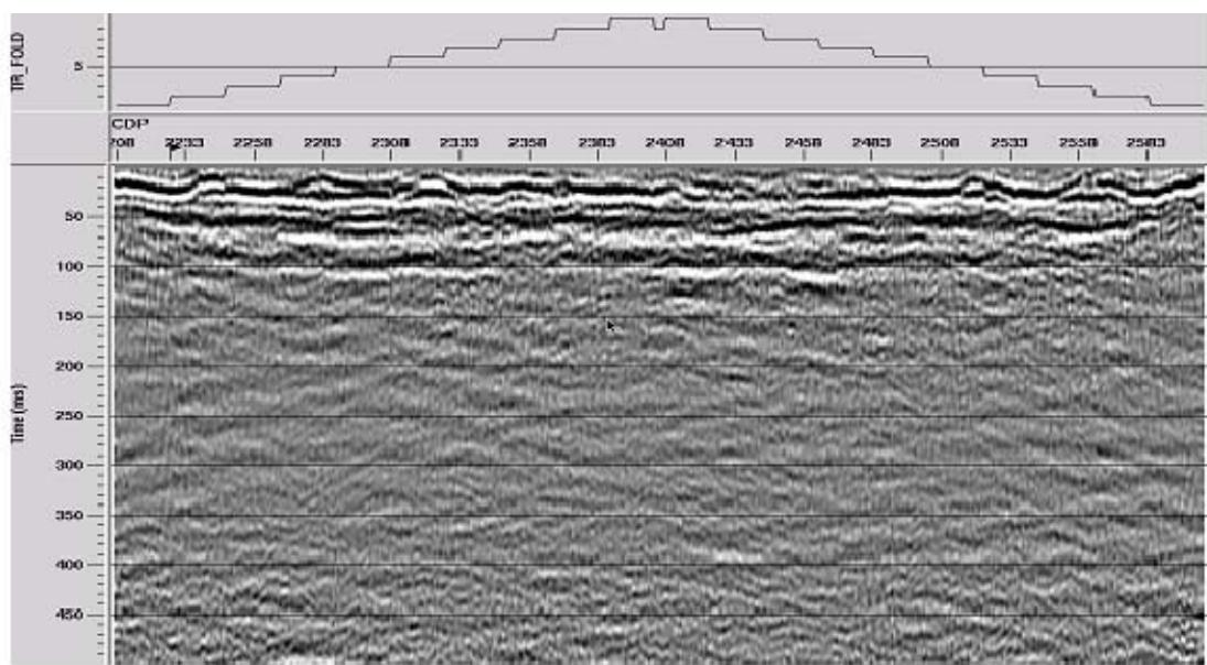
Priddis pulse probe—Dynamite + 50 Hz—CDP stack, 2000 m/s LM 0, reverse polarity
