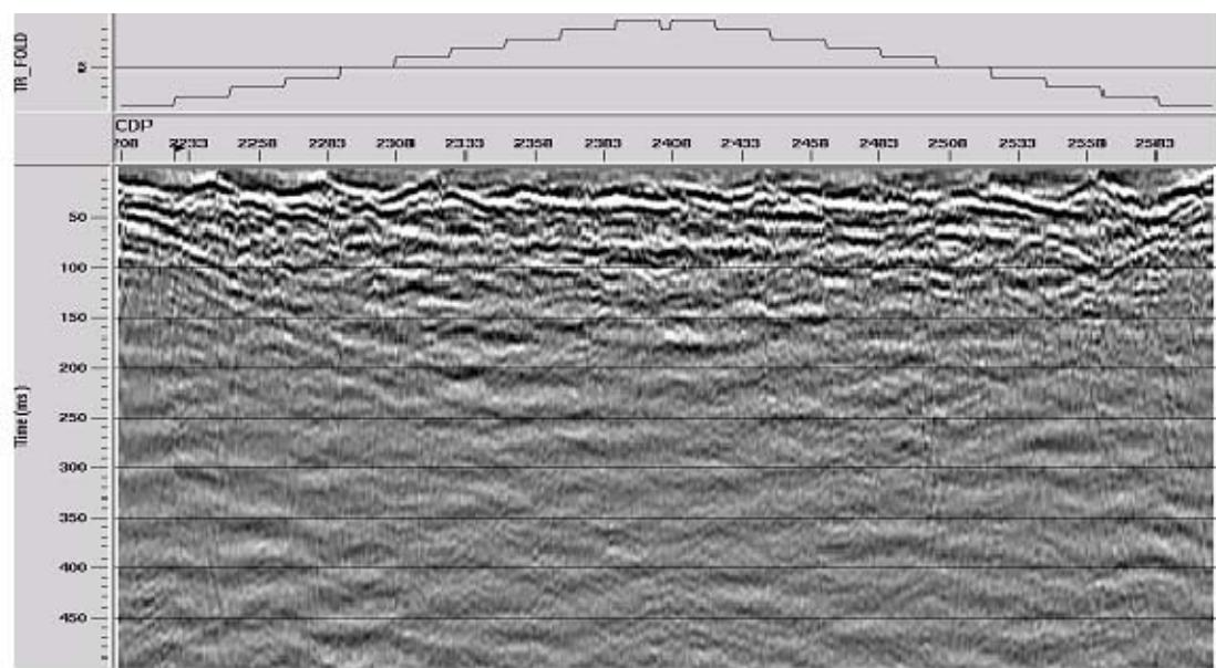
C D P stack of radial component—dynamite only—2000 m/s L M O
