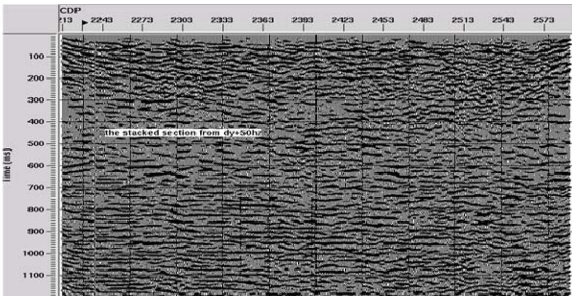
Stack of gathers for dynamite plus 50 Hz vibroseis
