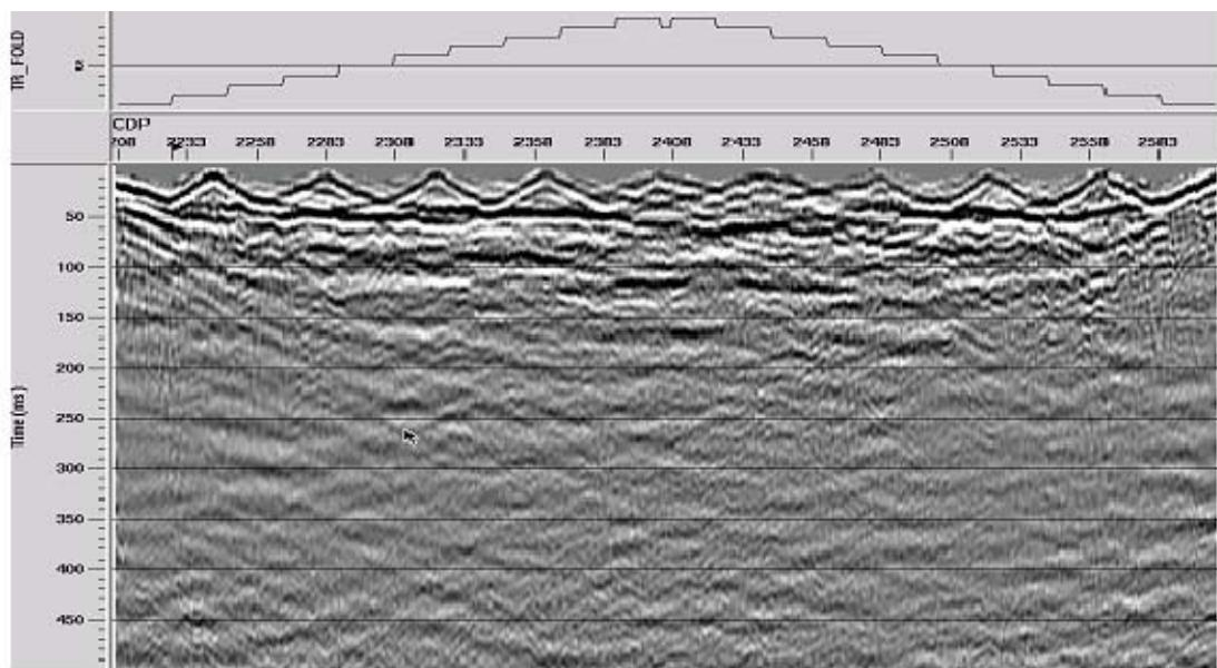
CDP stack of vertical component shots—dynamite only—2000 m/s NMO
