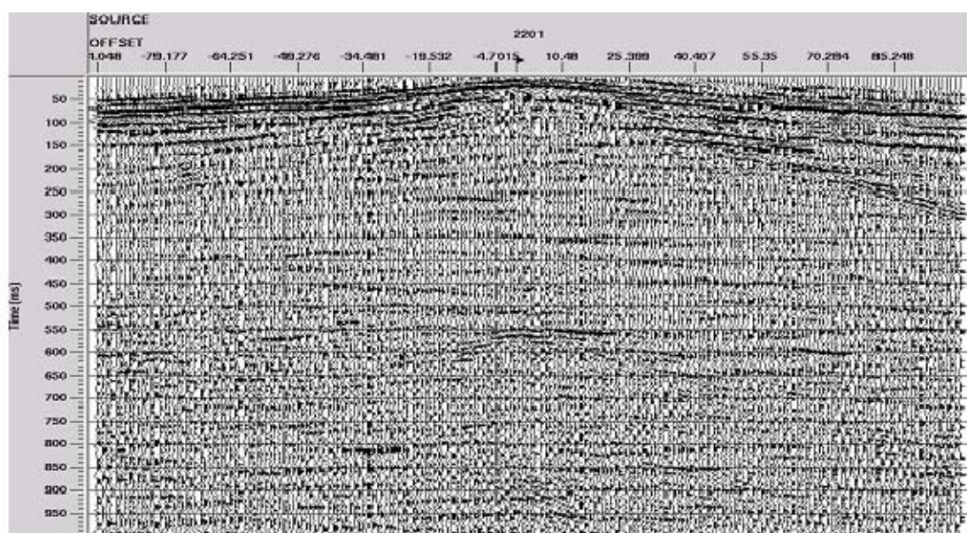
Priddis pulse probe—Dynamite + 50 Hz—typical shot after spectral clipping, filtering, decon
