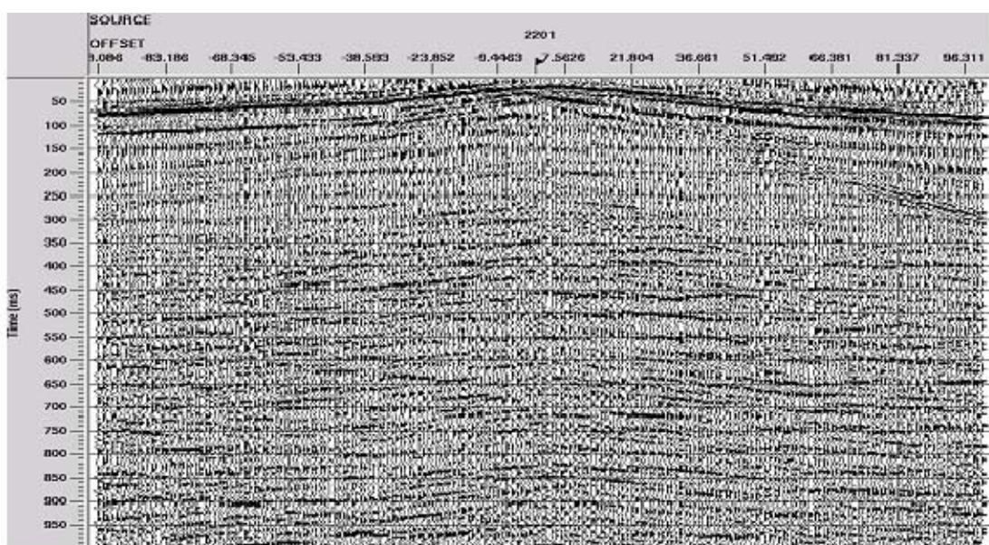
Typical shot gather—vibroseis only—after filtering and deconvolution
