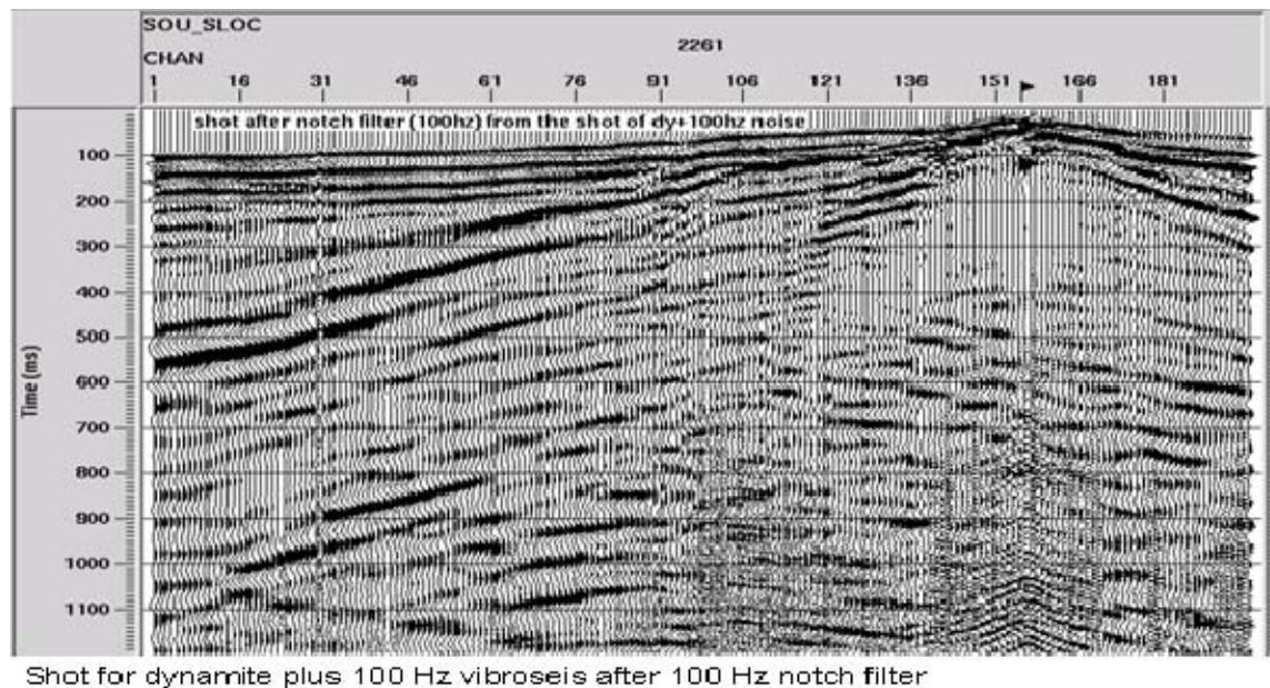
FIG. 21. 100 Hz pump-probe shot with 100 Hz notch filter applied. There is less residual noise on this gather, probably because of the display bandpass.
