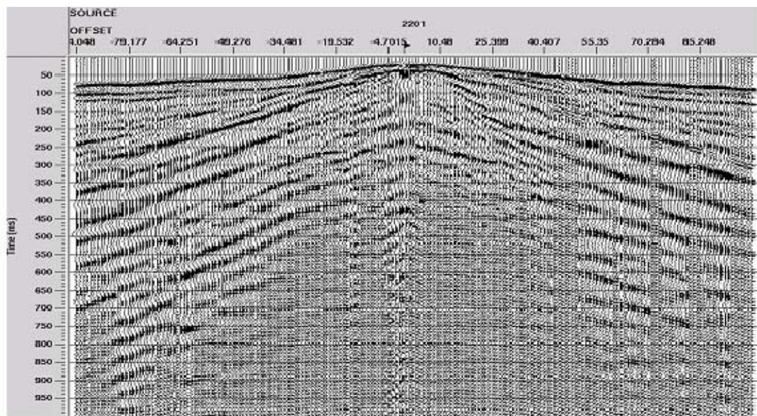
FIG. 41. Typical shot gather from 100 Hz pump-probe survey. 100 Hz Vibroseis signal is strong, but not dominant.
