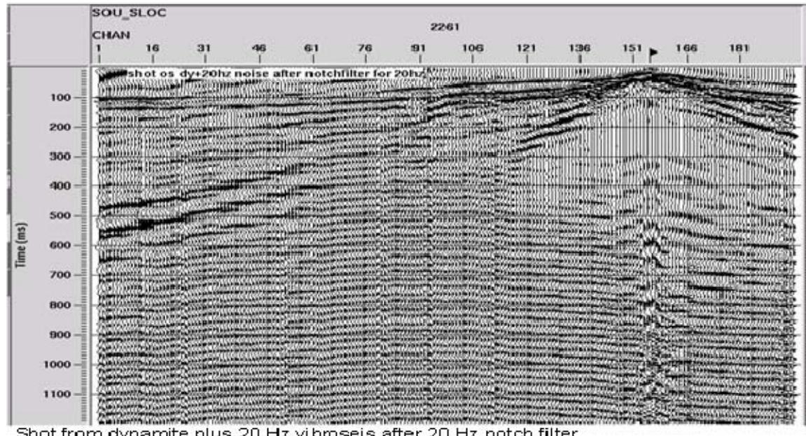
FIG. 18. Pump-probe gather from Figure 15 after application of 20 Hz notch filter. There is lots of Vibroseis signal left in this gather.
