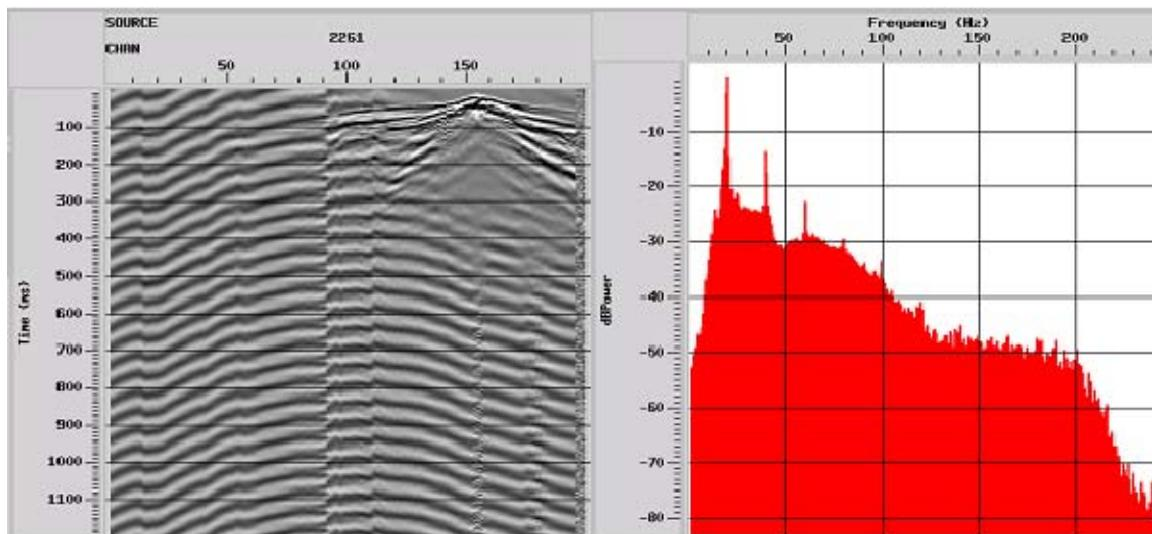
Amplitude spectrum for dynamite shot plus 20 Hz vibroseis—note significant harmonics at 40 Hz, 60 Hz
