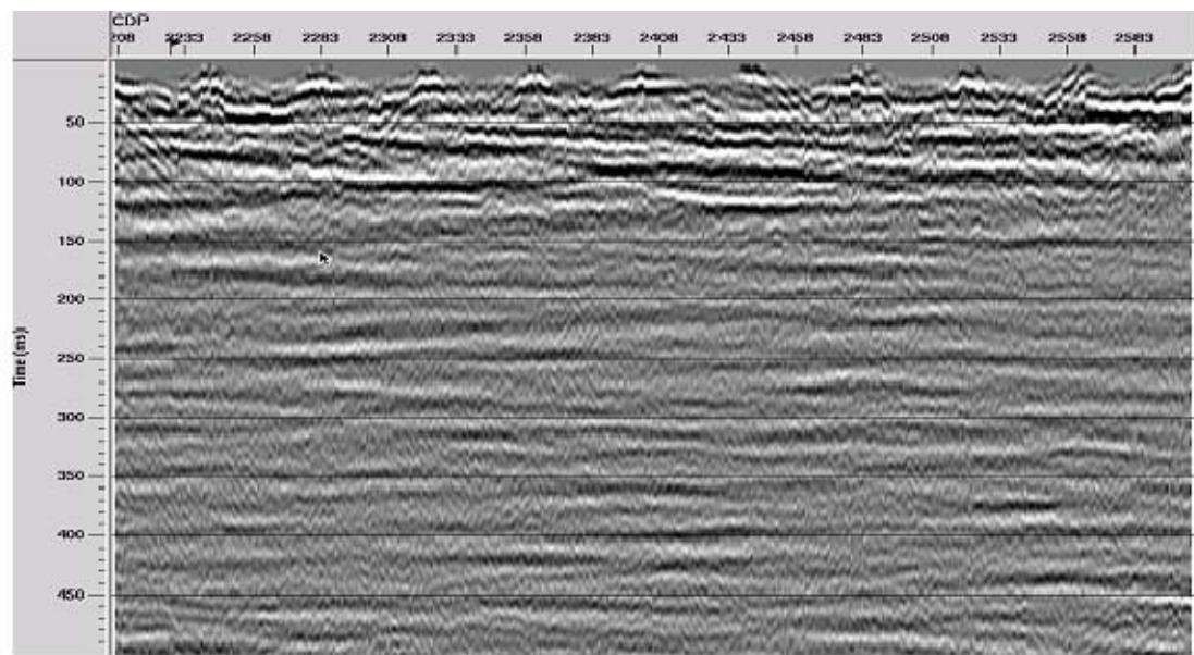
Dynamite plus 50 Hz with refractions attenuated
