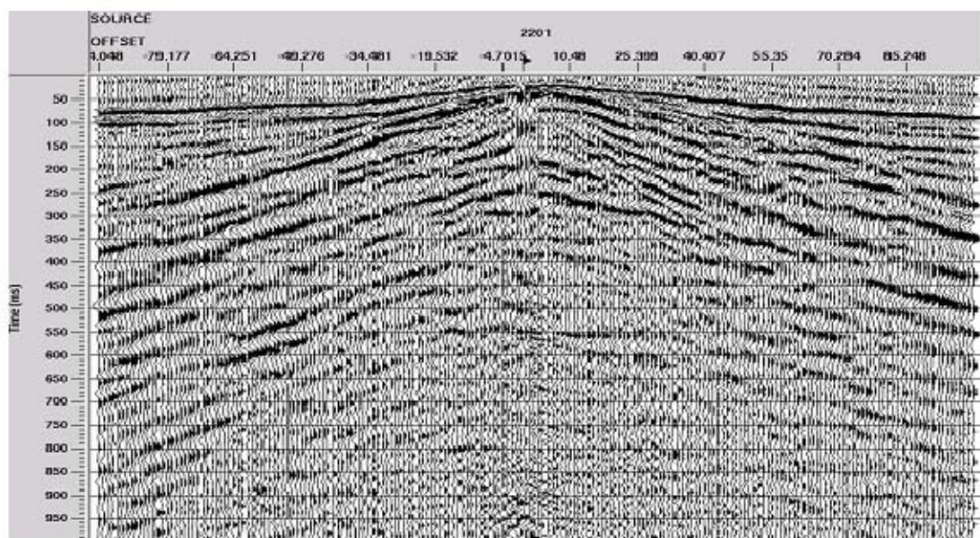
Priddis pulse probe—Dynamite + 50 Hz—typical shot after spectral clipping
