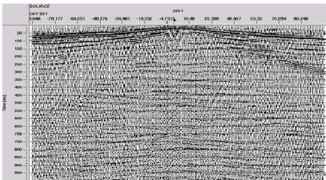
Priddis pulse probe — Dynamite + 100 Hz — typical shot after spectral clipping, filtering, deconvolution.
