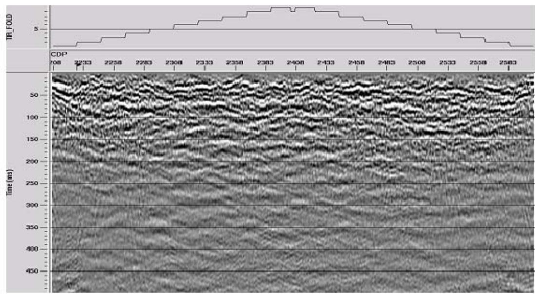
C D P stack of transverse component—dynamite only—2000 m/s L M O
