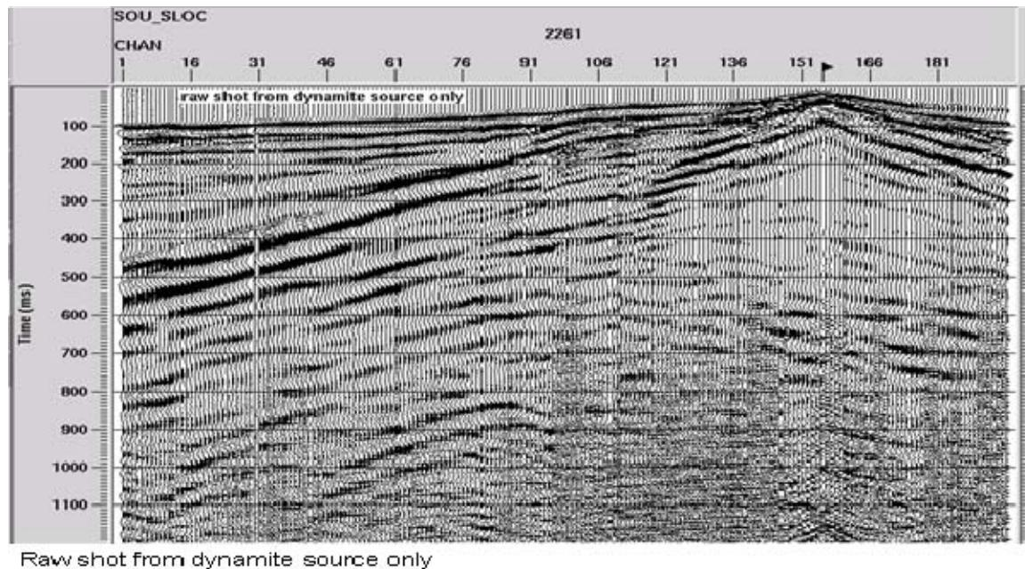
FIG. 14. Typical raw shot gather from 'dynamite only' survey. This gather is dominated by coherent noise and 60 Hz power line noise.
