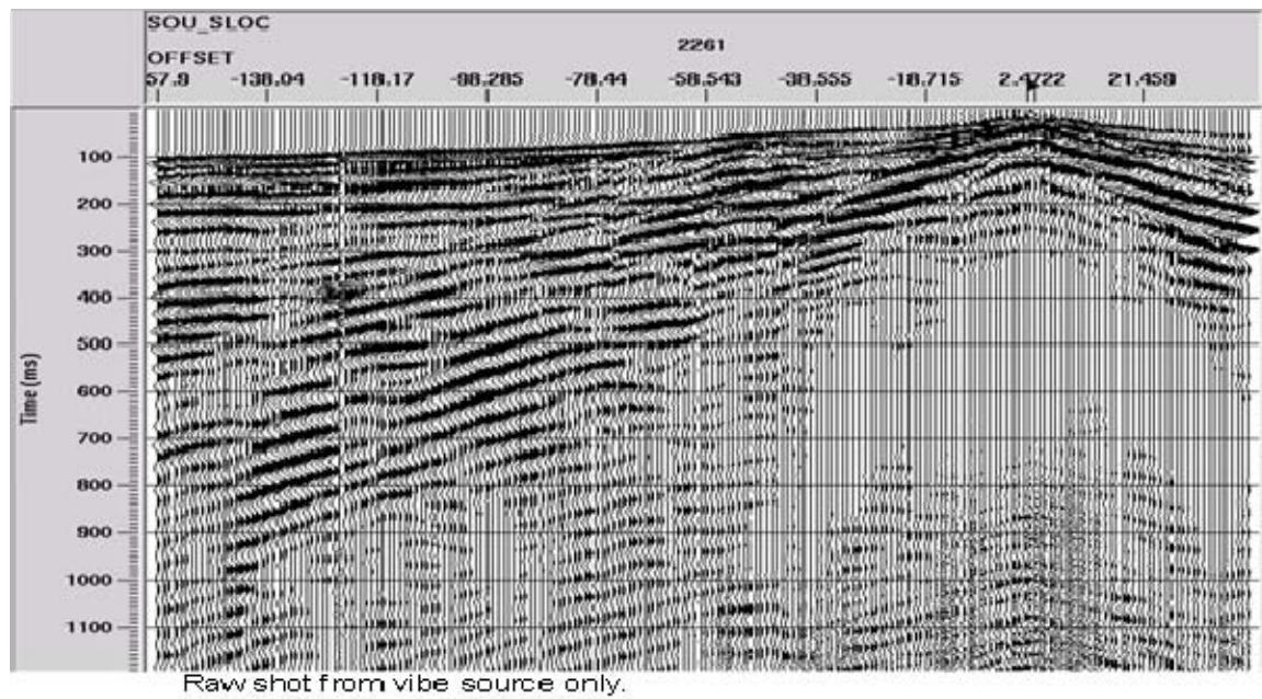
FIG. 13. Typical raw shot gather from 'Vibroseis only' survey. Coherent noise dominates the record.
