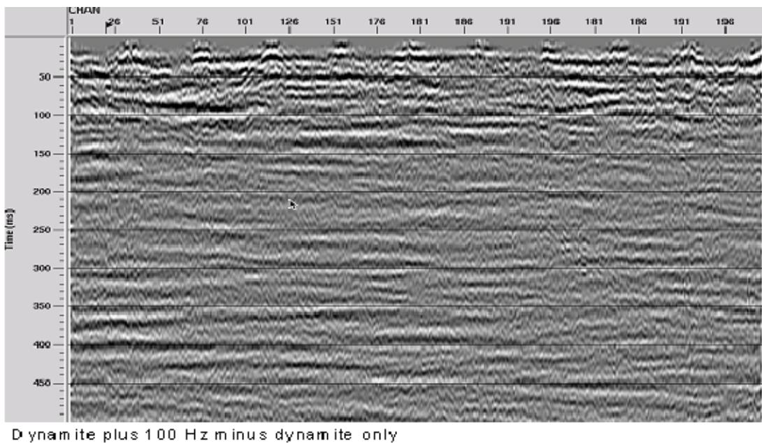
FIG. 60 CDP stack of 'dynamite plus 100 Hz' pulse-probe survey minus CDP stack of 'dynamite only' survey
