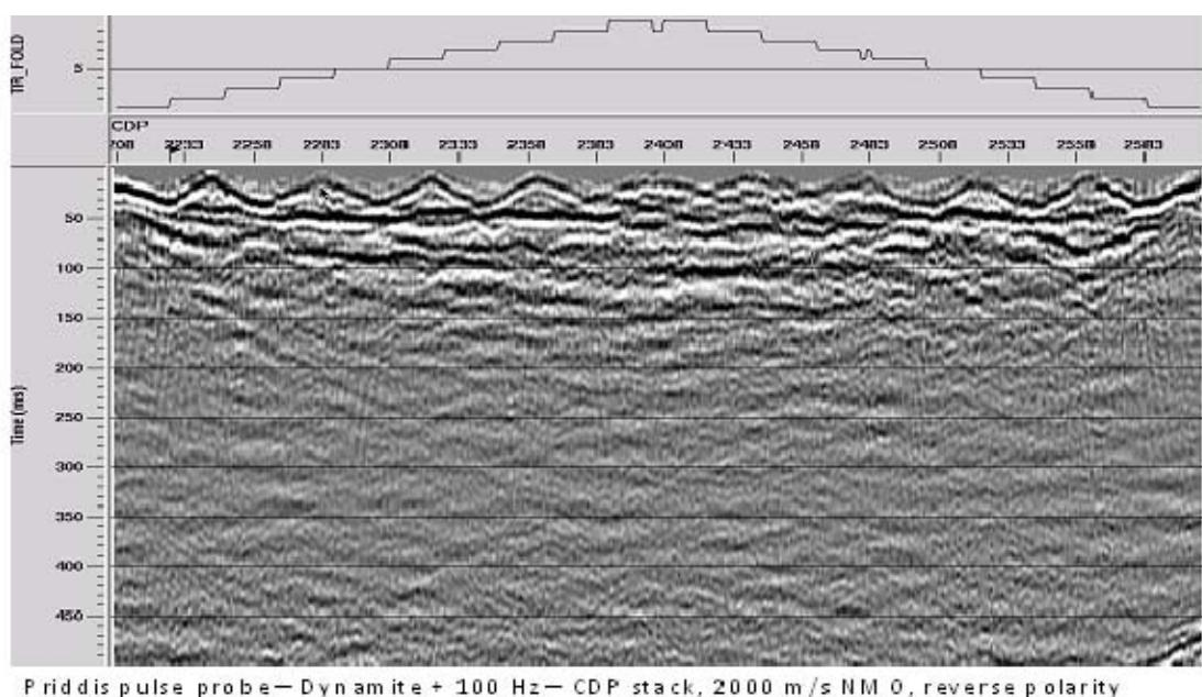
FIG. 48. CDP stack of 100 Hz pump-probe survey with 2000 m/s NMO applied to shot gathers.
