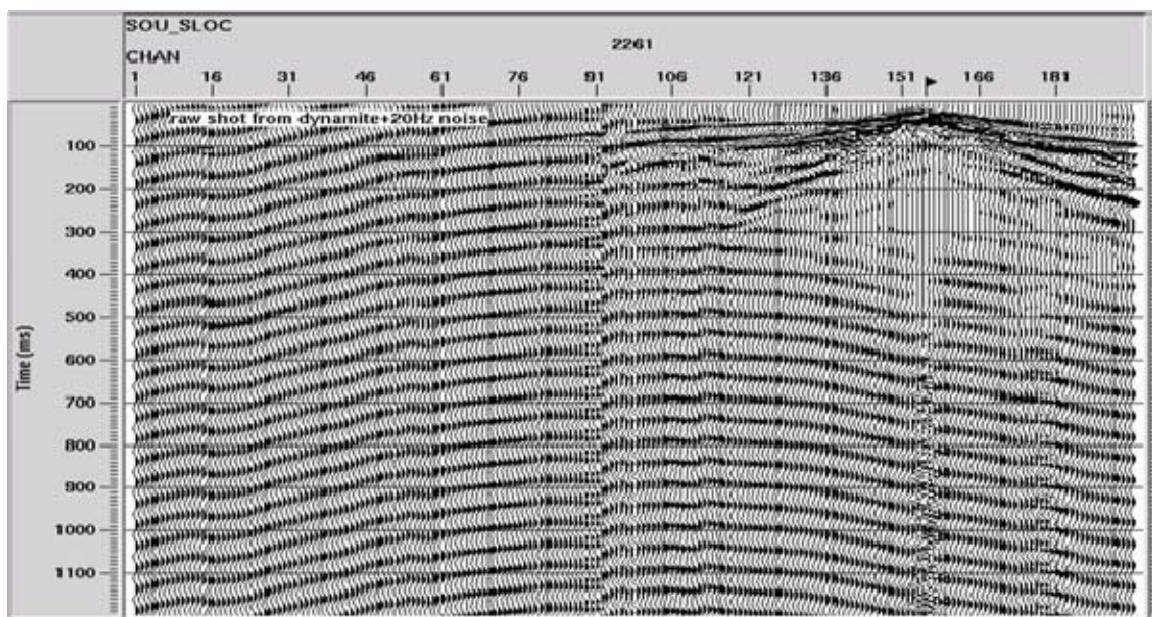
Raw shot from dynamite plus 20 Hz vibroseis
