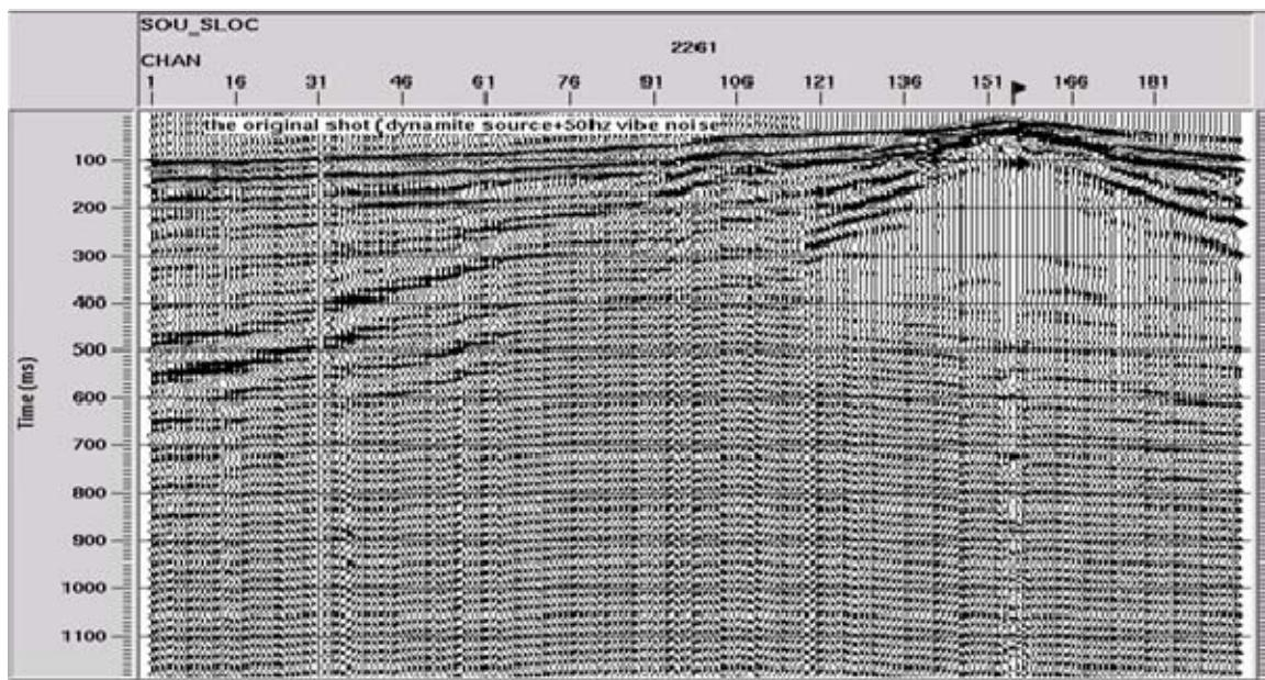
Raw shot from dynamite plus 50 Hz vibroseis
