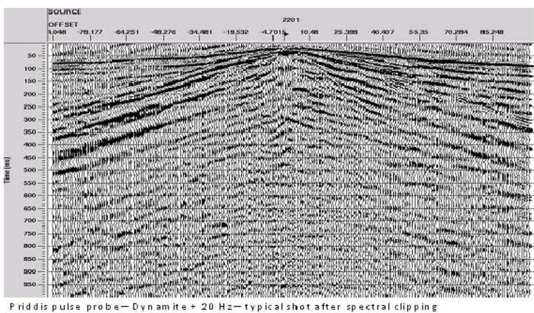
FIG. 36. Shot gather of Figure 35 after spectral clipping.
