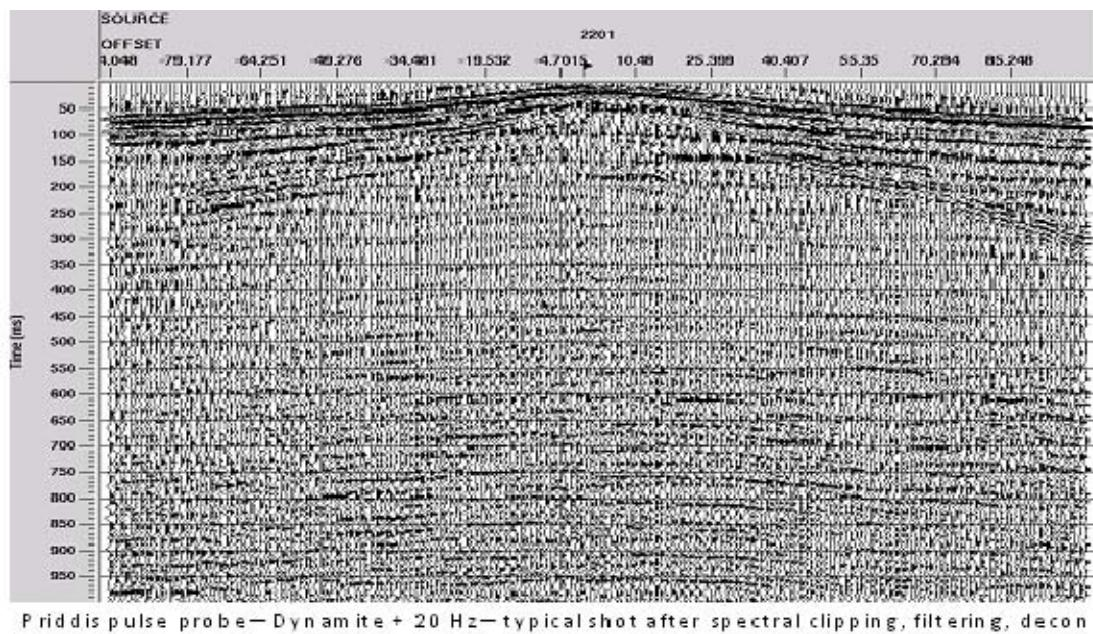
P riddis pulse probe—Dynamite + 20 Hz—typical shot after spectral clipping, filtering, decon
