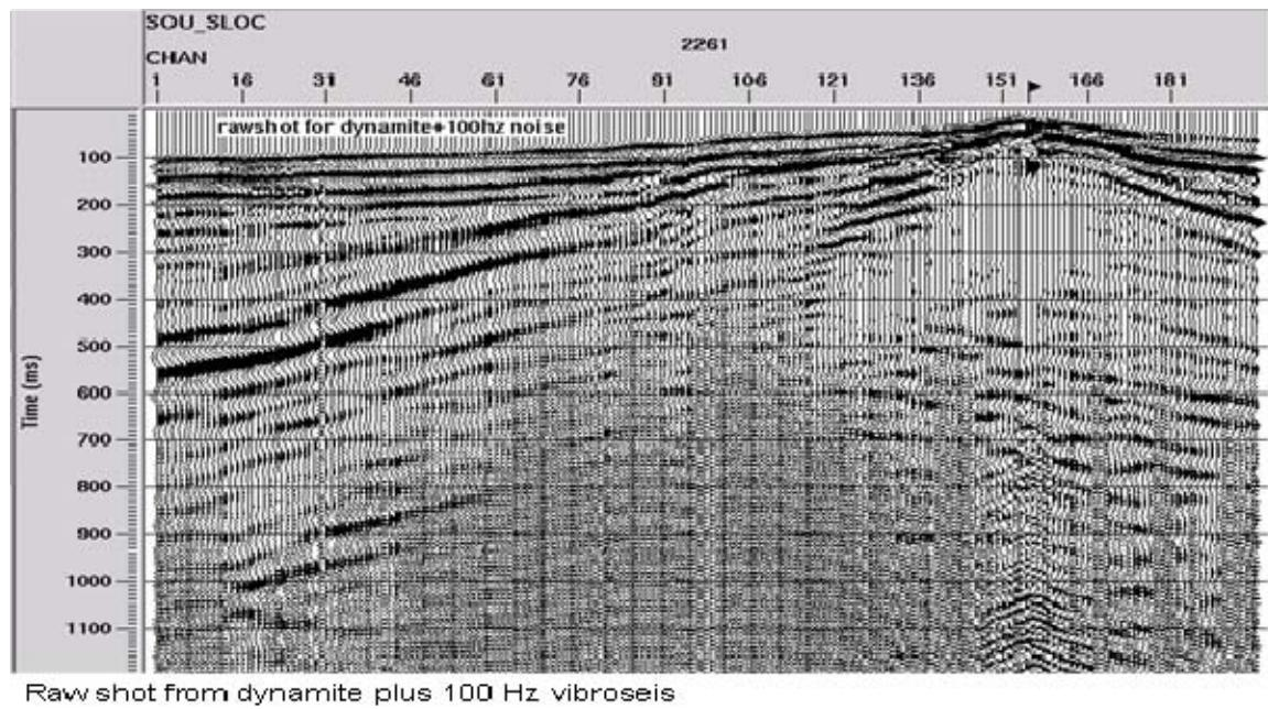
Raw shot from dynamite plus 100 Hz vibroseis
