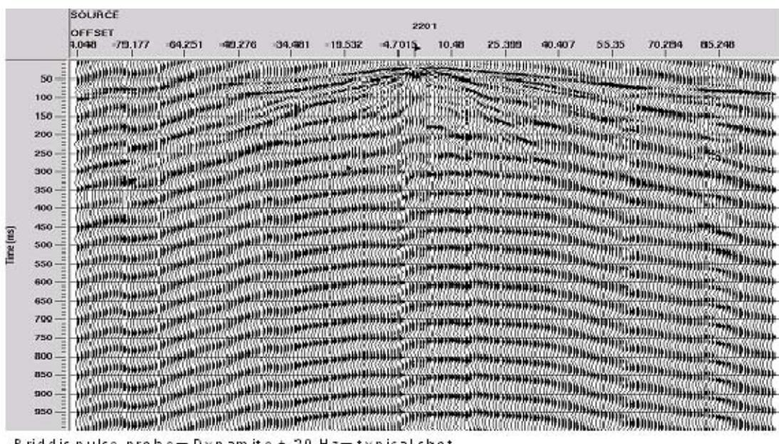
FIG. 35. Typical shot gather for 20 Hz pump-probe survey. Vibroseis signal dominates the record.
