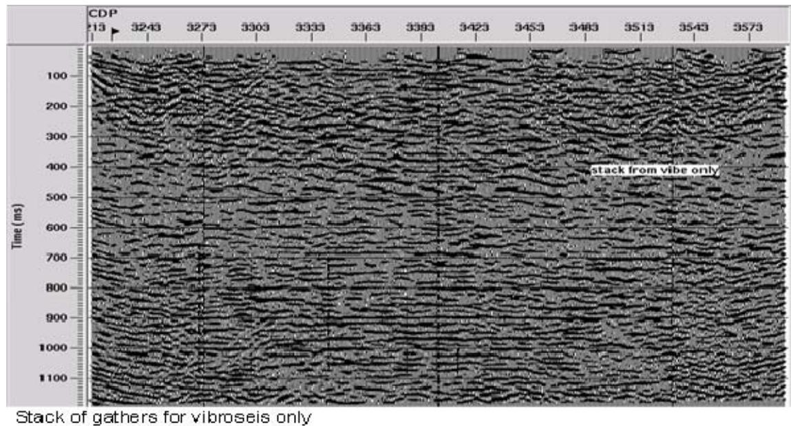
FIG. 26. CDP stack of the 'Vibroseis only' gathers. Coherent events between 600 ms and 900 ms may not be reflections, since we can't reliably see known dipping reflections at 250 ms and 450 ms.
