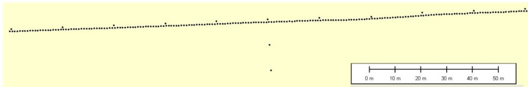
FIG. 1. Source and receiver location map (North is up). Multicomponent geophones were planted at 1 m spacing, with station numbers increasing to the east. Shot holes nominally 1.8 m deep were drilled and cased every 20 m, offset 1 m to the north of the receiver line. Centred on the receiver line, but offset 10 m to the south we have the test borehole location with a single 3C clamping geophone at 75 m depth. A single shot hole was located a further 10 m south of the borehole.
