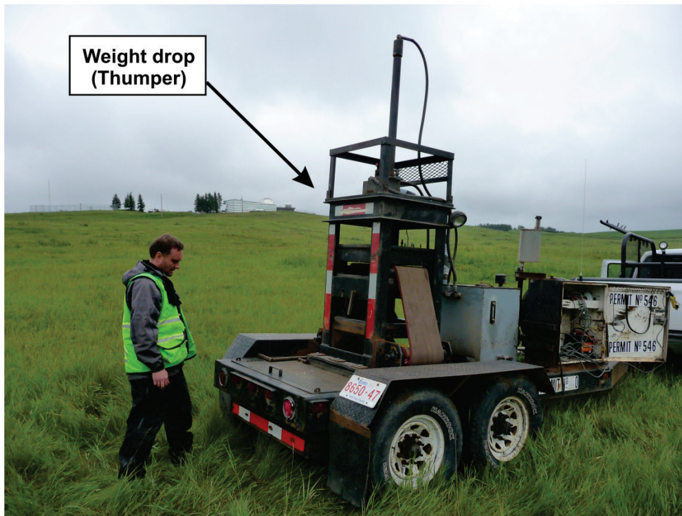
Fig. 3. Layout of the field experiment. Top panel shows the procedure for installing the Trillium-240 seismometer and Taurus digital seismograph. Lower panel shows the weight-drop source.
