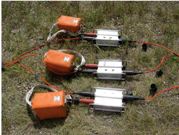
FIG 3. 3-component acquisition with each component defined as a separate ARAM receiver line.
