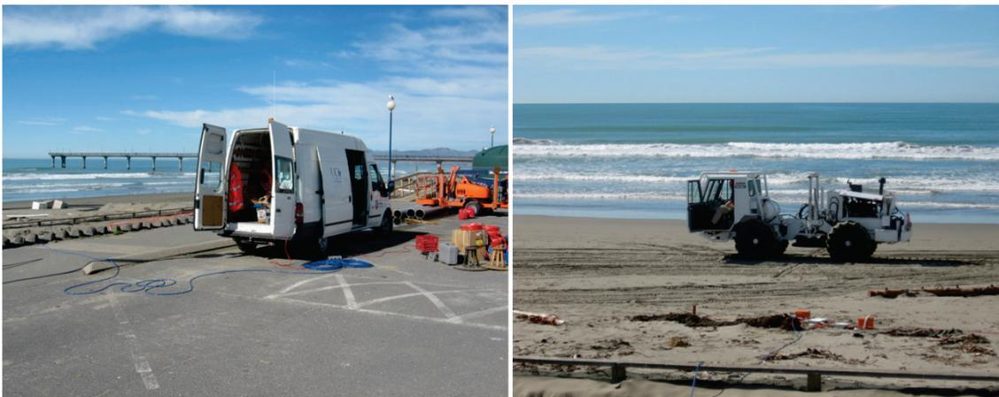
FIG. 6. Recording the seismic line along New Brighton Beach, Christchurch. Recorder van is in left picture and geophone spread is in the foreground of the picture on right.
