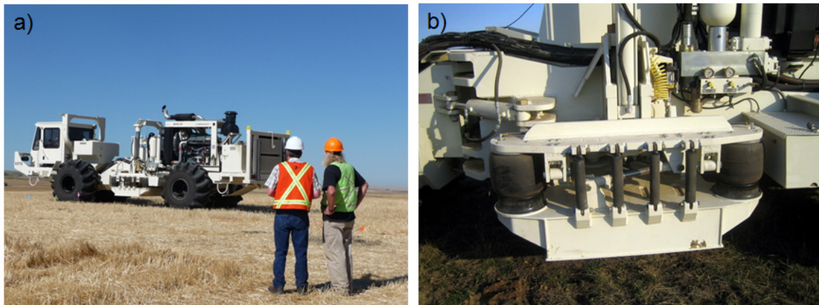
Fig. 5: a) The 62,000 lb INOVA 364 low-frequency vibrator in action at Hussar. b) A close-up of the specially stiffened baseplate.
