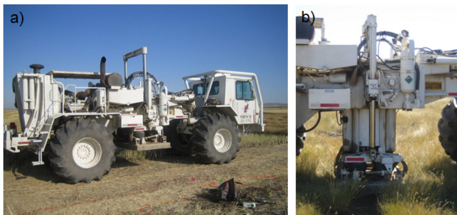
Fig. 6: a) The 47,000lb Failing Y-2400 production vibrator. b) A close-up of the baseplate assembly.
