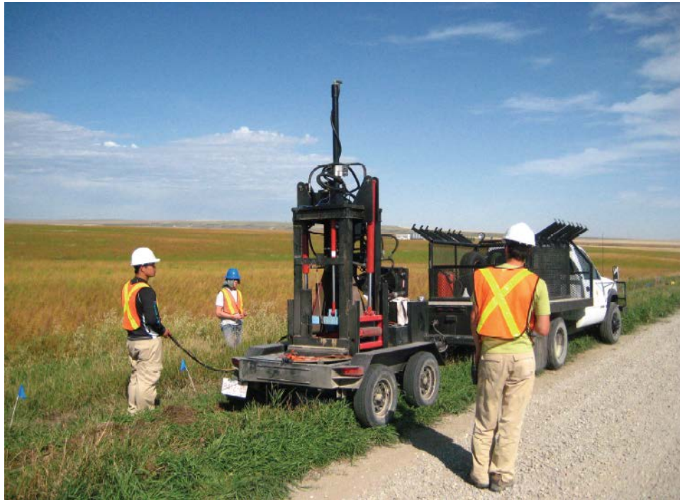
FIG. 5. The seismic thumper.
