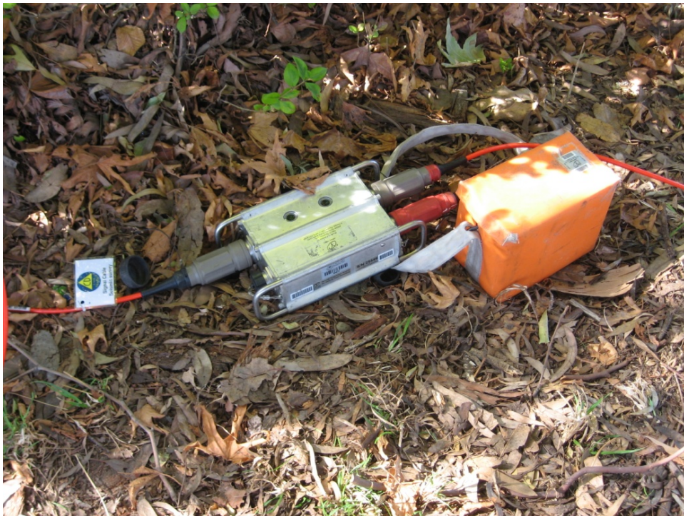
FIG. 4. Remote Acquisition Module and battery on the line.
