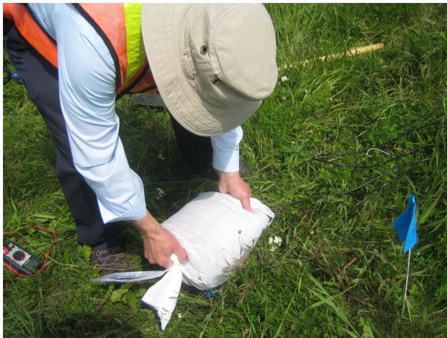
FIG. 15. Laying a sandbag on top of a geophone.
