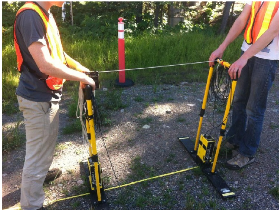
FIG. 7. The Pulse Ekko Pro GPR system.
