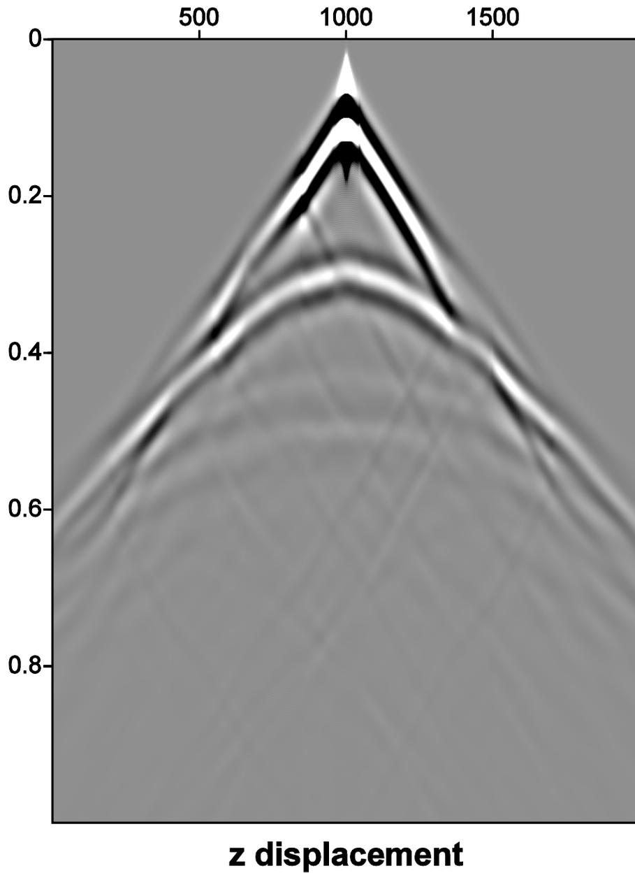
FIG. 1. Plot of all traces of one shot, showing alternating clear and grayed out first breaks due to low velocity pockets, and straight lines due to the vertical boundaries of the low velocity pockets.
