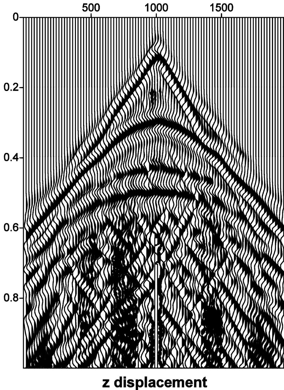
FIG 3. This variable area / wiggly plot shows poorly on monitors, but a printed version reveals two traces at the centre which, after a spike, become straight lines. A hardcopy plot also reveals expected numerical jitter towards the bottom.
