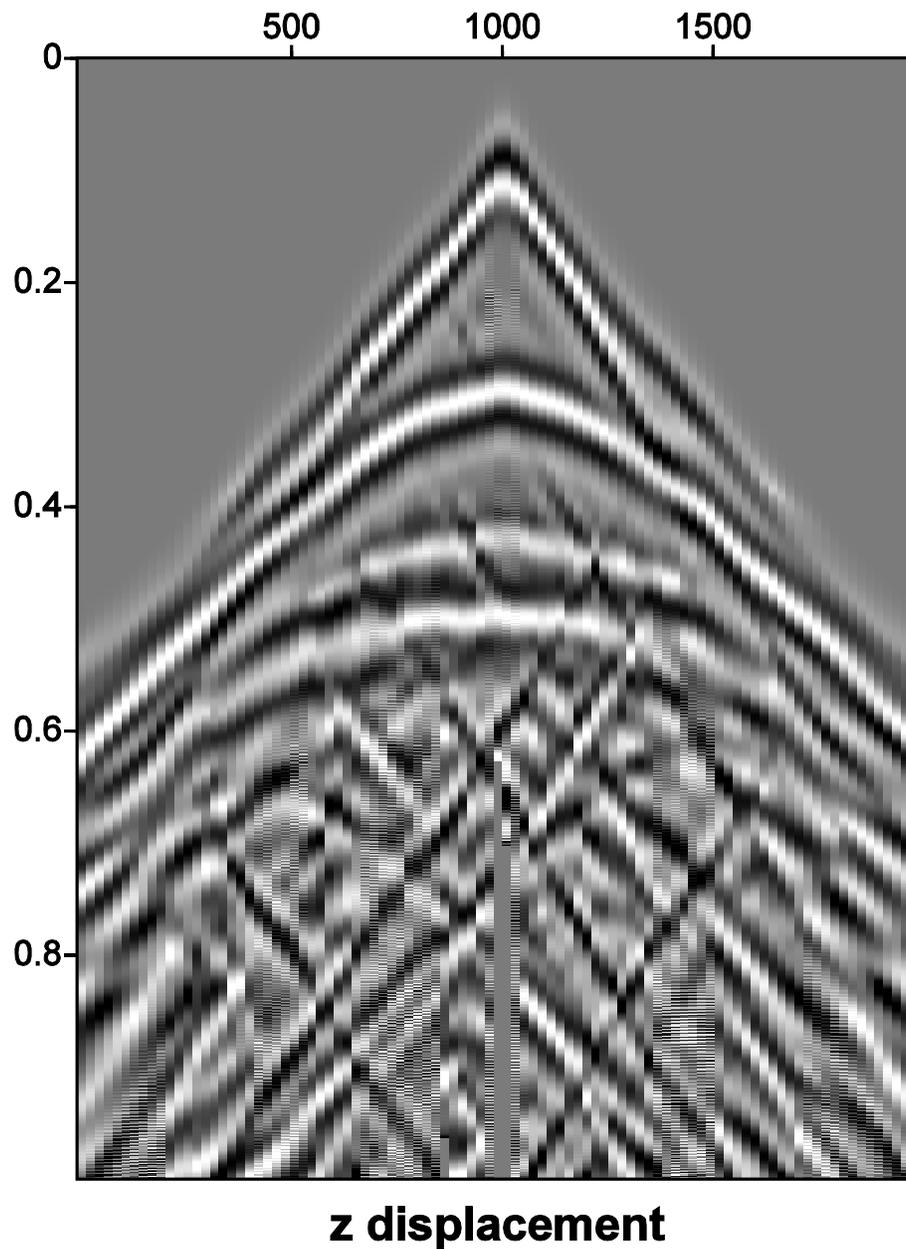
FIG 2. The same data displaying only every 7th trace. The effect of the low velocity layers on the first breaks becomes more readily visible, as do reflections which look as if due to a slanted interface but must be the result of a reflection of ray a hitting first a low/high velocity boundary near the surface, then an interface.
