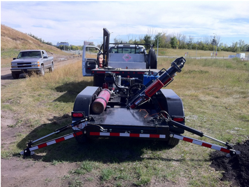
FIG. 1. The new CREWES S-wave seismic source in S-wave mode.
