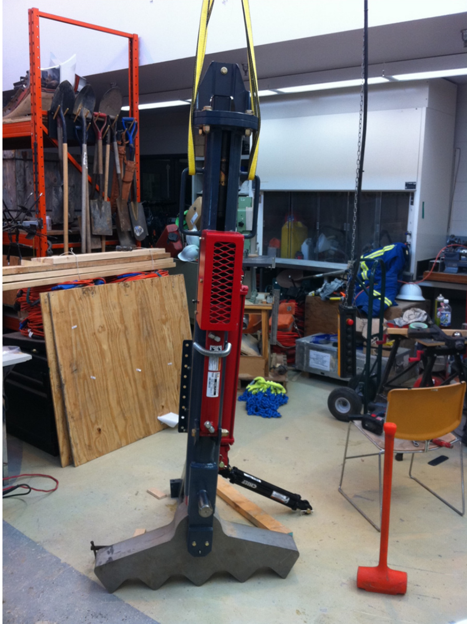
FIG. 2. The USAInc compressed nitrogen accelerated weight-drop source as delivered.
