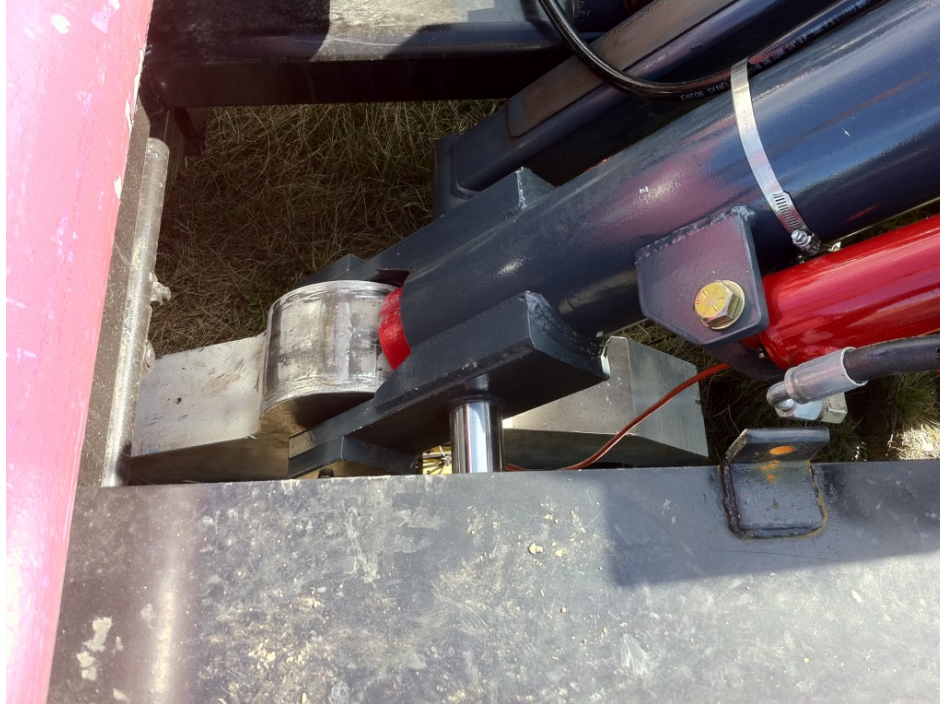
FIG. 4. S-wave source hammer and foot in contact with the ground.
