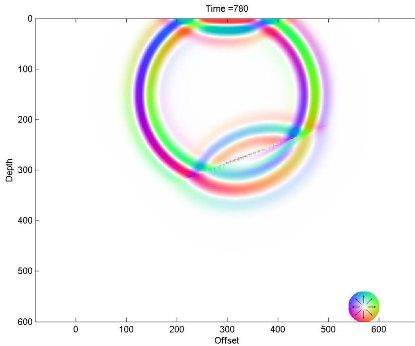
Figure 5: A wave front snapshot as in Figure 4, but with a slope of 37%. With this slope instability begins to appear which will gradually dominate the plot.
