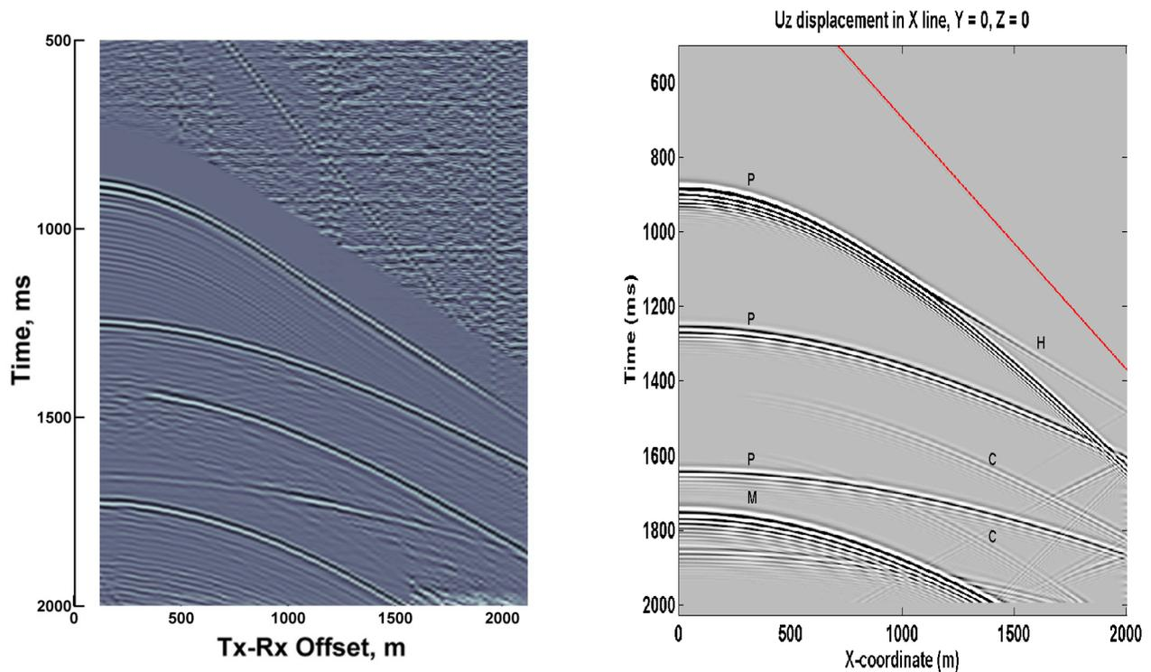
Figure 1: At left is a physical model with 200 ms AGC. At right is a numerical model with parameters of the layers approximately the same as those from the physical model. Primaries are marked P, a multiple marked M, a head-wave marked H, and converted wave events, reconverted, are marked C. The most obvious difference is the complete conversion of the first primary reflection into a head-wave in the physical model.
